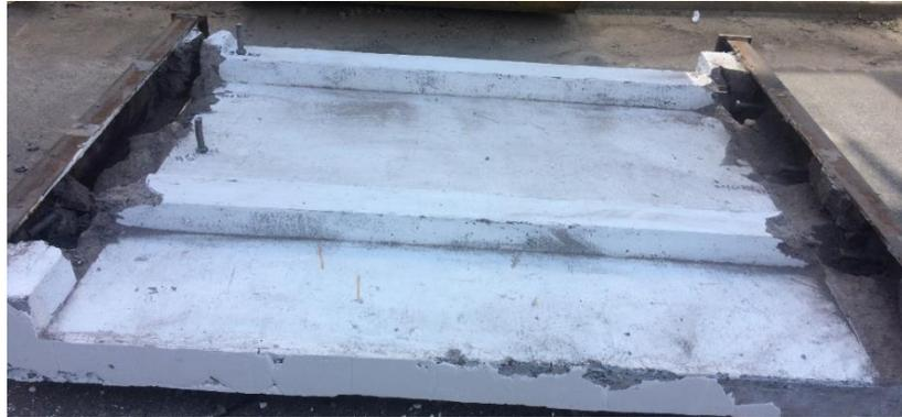
(a): Bending and shearing off of the shear stud connectors
