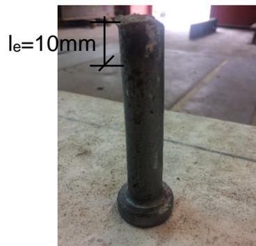
(b): Bending length of the shear connector
