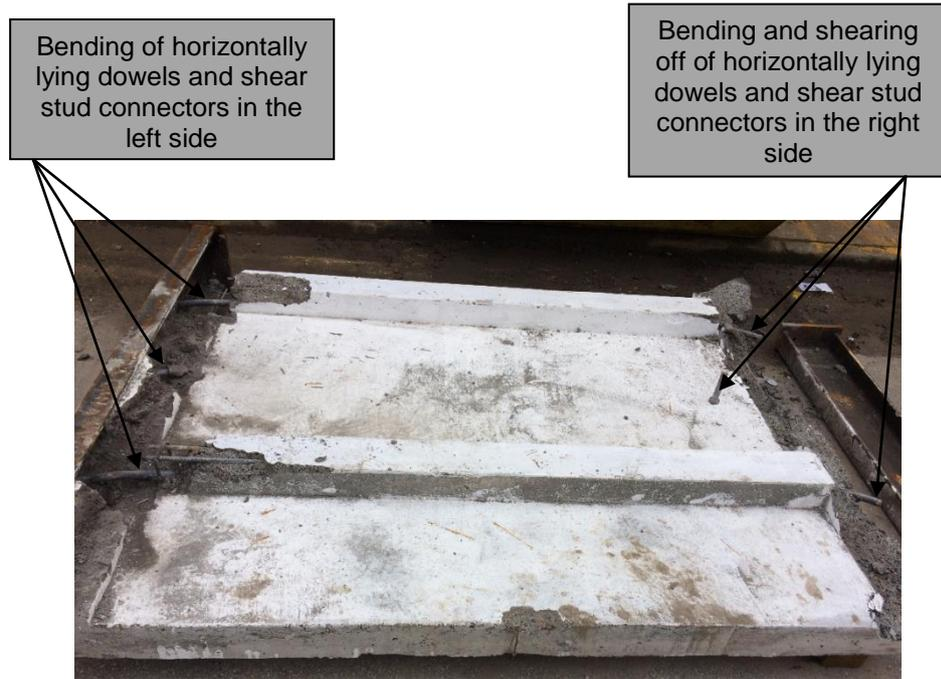
(a): Bending and shearing off of the shear connectors
