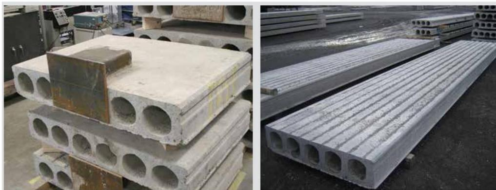
(a) Specimen with machine-finished (b) Longitudinally raked slab
