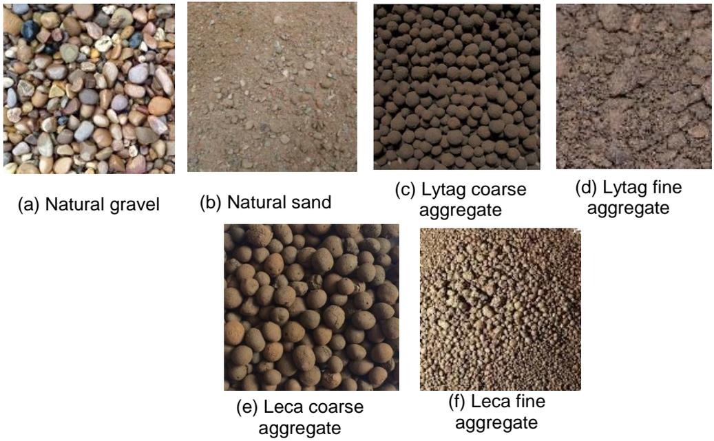
Figure 3-1: Different types of aggregates used in preparing concrete mixes
