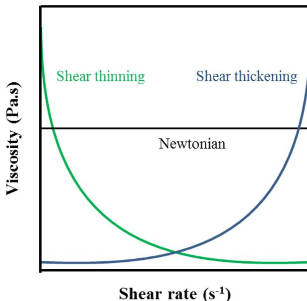
**Figure 1.4. Typical flow-curves for Newtonian and non-Newtonian fluids (van Vliet 2014).**
