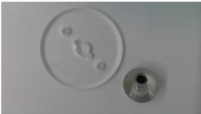
**Figure 1.7. Commercial PDMS ball and disc tribology specimens.**
