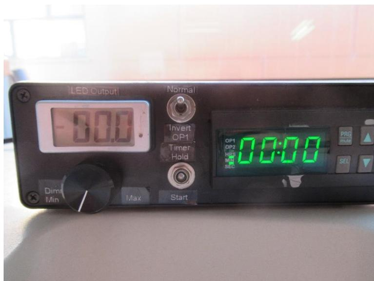
**Figure 145: Irradiation control unit developed at the University of York. On the left side is a dimmer switch and power readout to control the power drawn by the LED. On the right side is a programmable timer function that allows repeated on/off cycles.**
