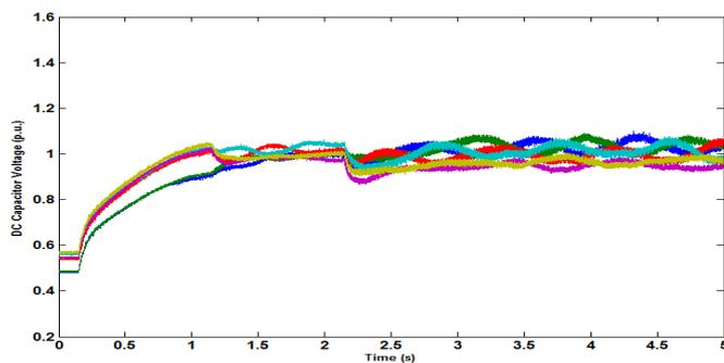
Fig. 5.18 6 Module DC capacitor voltage waveforms
