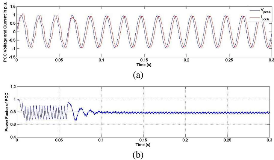
Fig. 3.32 (a) PCC voltage and current and (b) PCC power factor variation with harmonics control but without reactive power compensation
