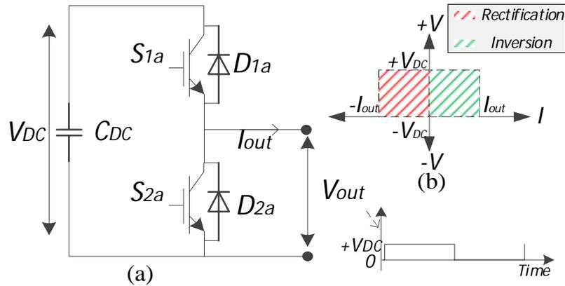
Fig. 2.1 (a) Half-bridge SM circuit; (b) Operating quadrants
