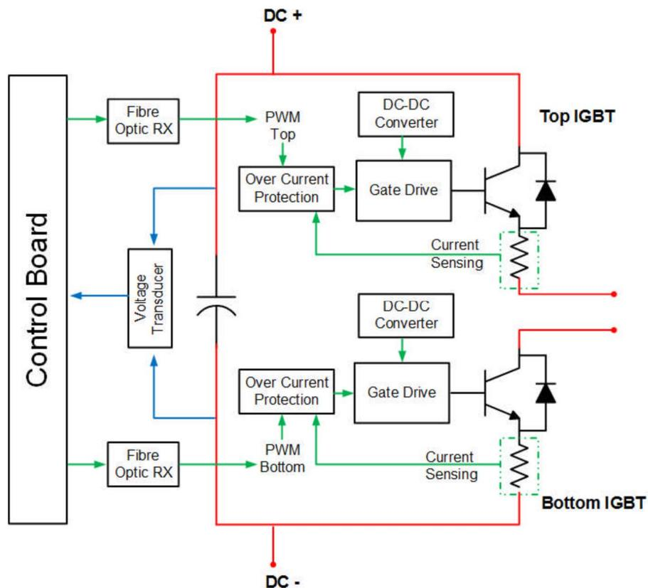
Fig. 5.4 Cell card power circuit
