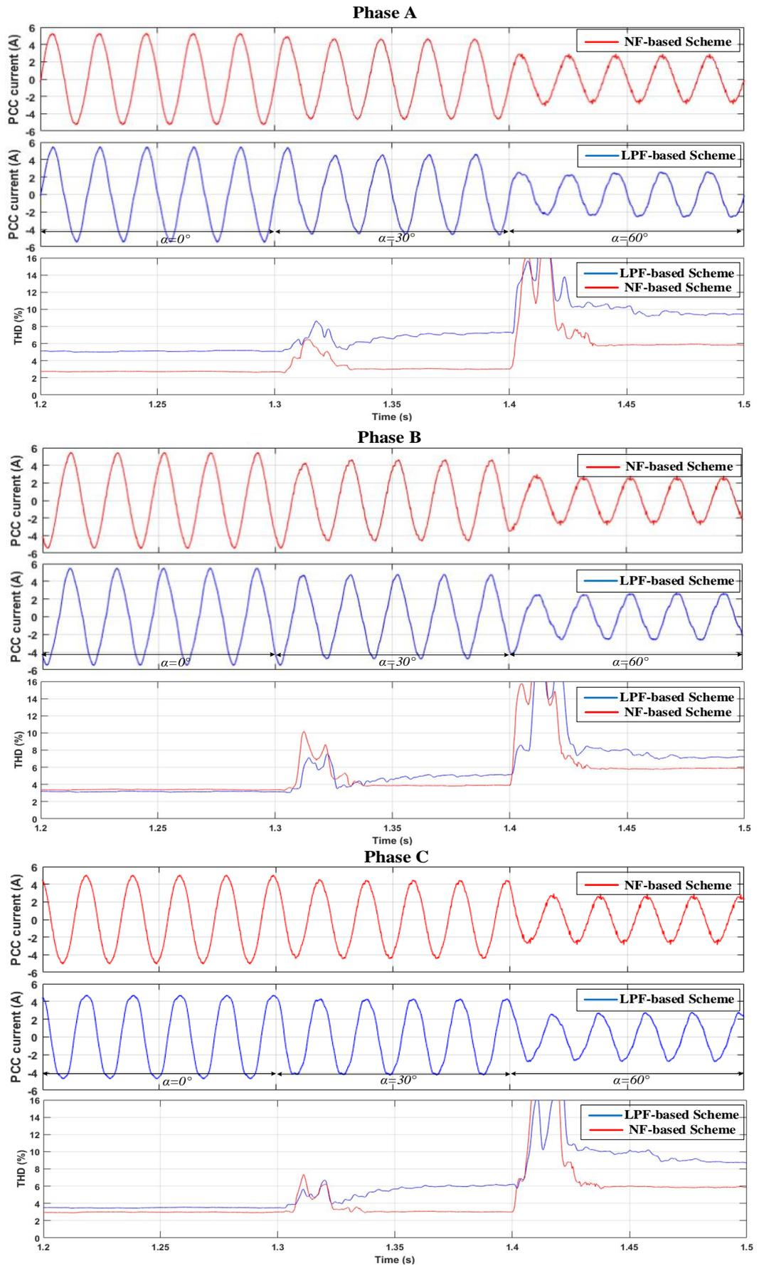
Fig. 4.13 Three phases compensated currents and their THD comparison under NF and LPF-based schemes
