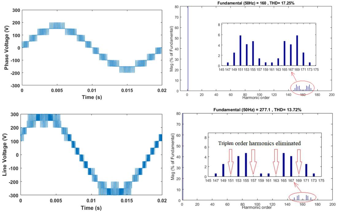
Fig. 2.17 5-level MMCC output phase voltage (upper) and line voltage (bottom) with their harmonics spectra for PS-PWM when  $f_c=1$  kHz
