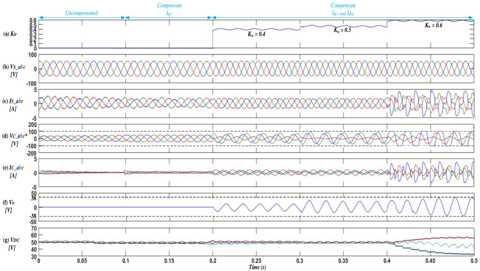
Fig. 5.19 SSBC Compensation of load current imbalance without harmonics
