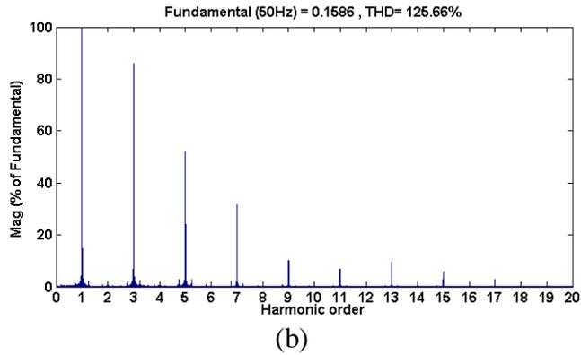
Fig. 3.3 (a) LCD monitor steady-state current waveform and (b) its harmonic spectrum
