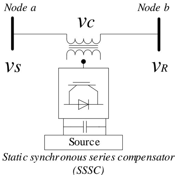
Fig. 1.6 Static synchronous series compensator (SSSC)
