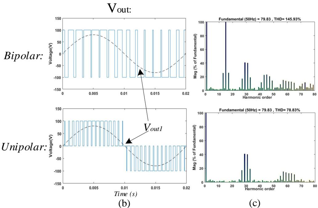
Fig. 2.14 Bipolar & Unipolar sine-triangle PWM applied to the full bridge converter and the corresponding AC terminal voltage waveform with their harmonic spectra
