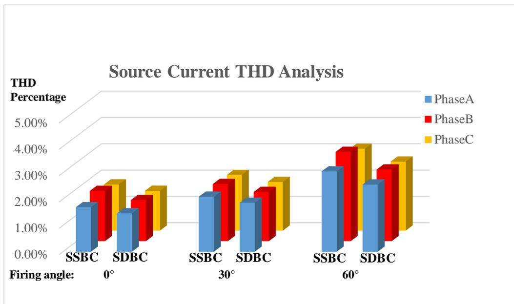
Fig. 4.27 The THDs of the 3-phase source current for Case A
