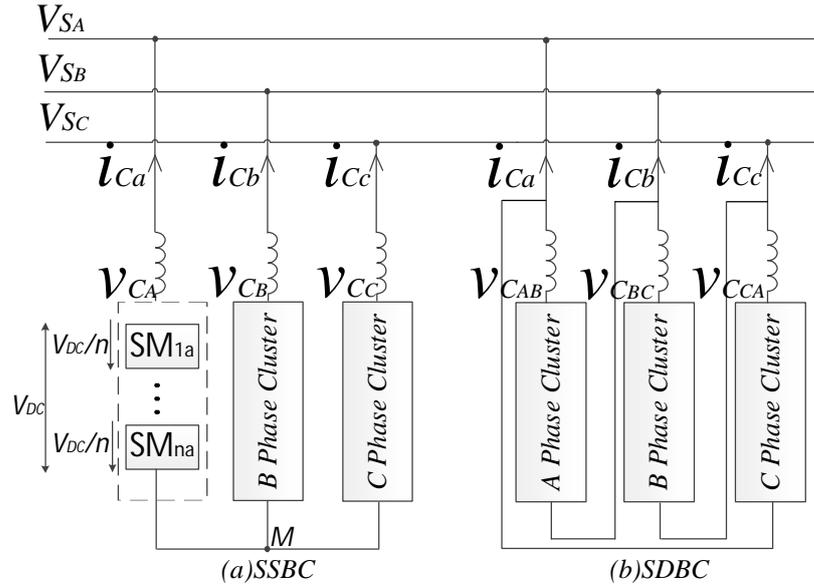
Fig. 4.16 Simplified configuration of (a) SSBC and (b) SDBC
