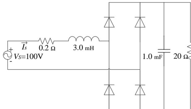
Fig. 3.1 Single-phase diode rectifier with output filter
