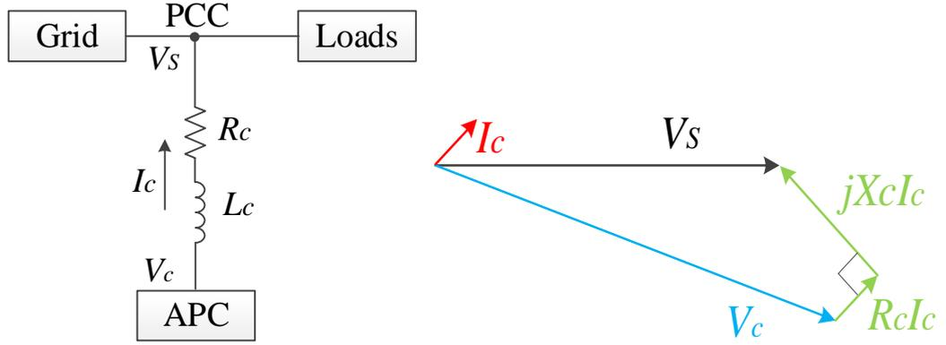
Fig. 3.15 (a) APC block diagram and (b) phasor diagram
