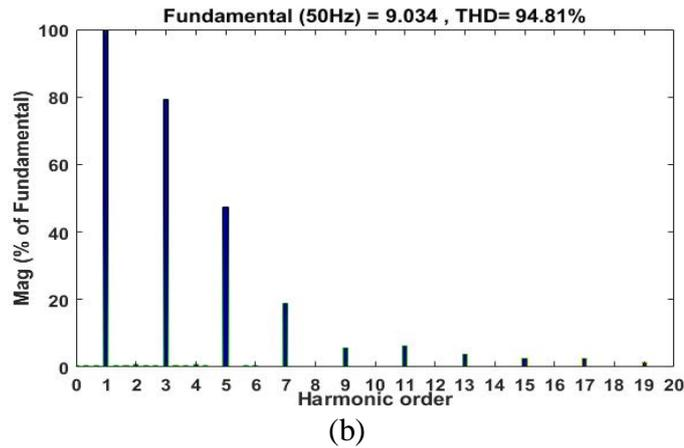
Fig. 3.2 (a) AC current waveform and its (b) harmonics spectrum
