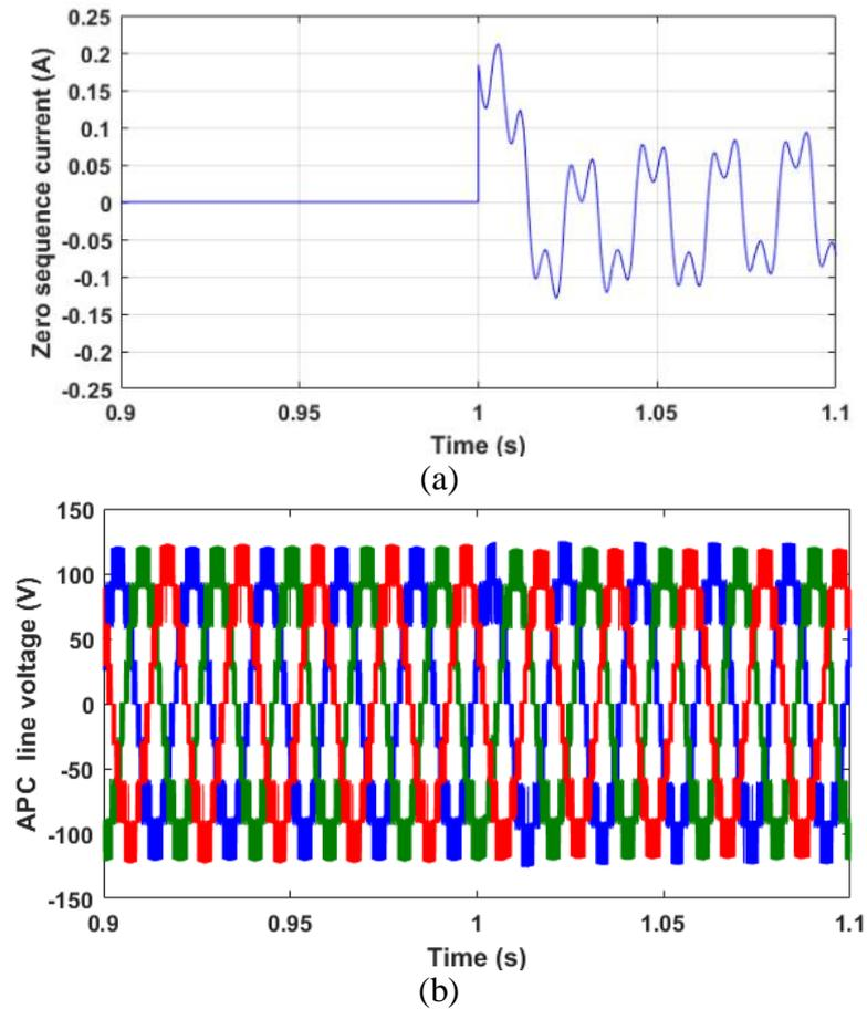
Fig. 4.24 (a) Zero sequence current and (b) three-phase line voltage for **SDBC** (Phase A: blue, Phase B: green, Phase C: red)
