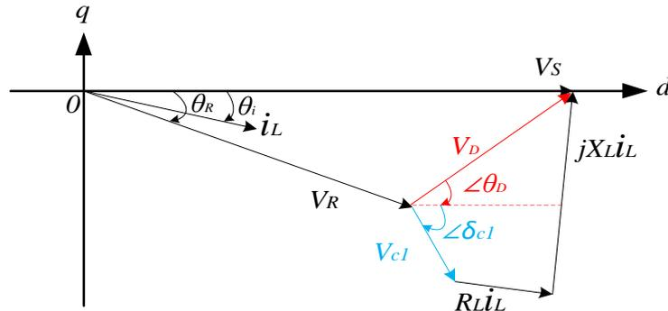
Fig. 6.6 SSSC phasor diagram
