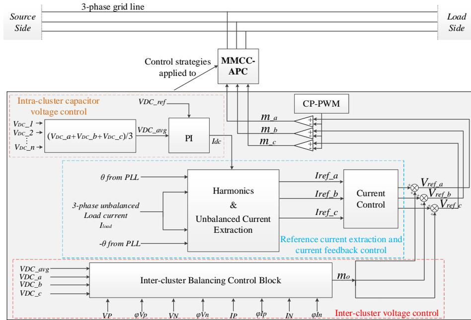
Fig. 4.19 Blocks diagram of overall control scheme
