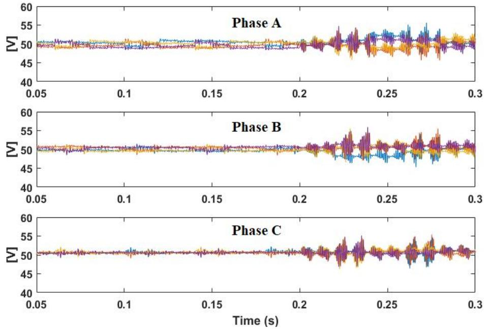
Fig. 3.36 Submodule inner flying capacitors voltage waveforms
