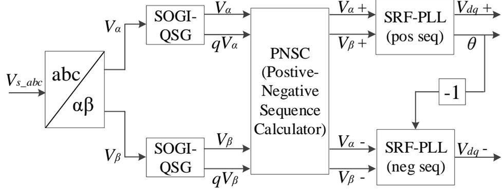
Fig. 1.20 Block diagram of Decoupled Second Order General Integrator-PLL
