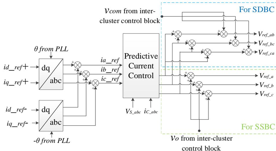
Fig. 4.20 Predictive current control block diagram
