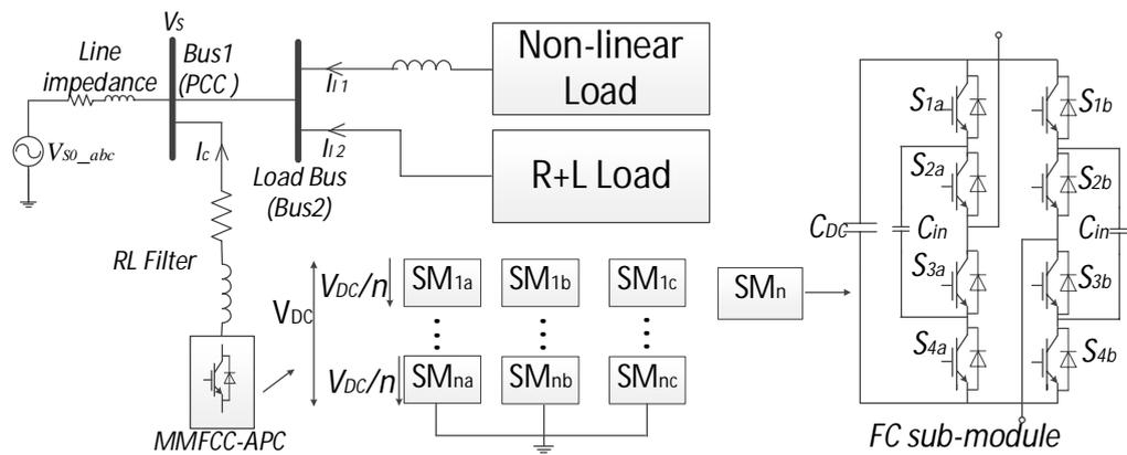
Fig. 3.12 Circuit configuration of MMFCC-APC
