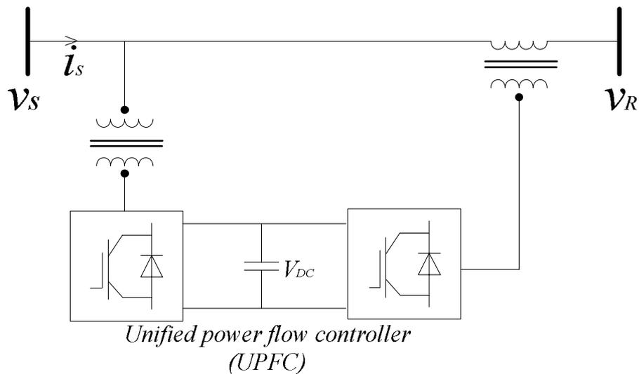
Fig. 1.8 Unified Power Flow Controller (UPFC)
