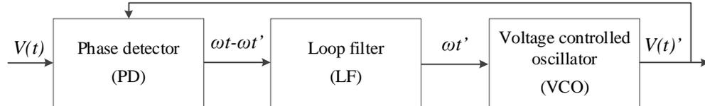
Fig. 1.15 Basic structure of closed-loop PLL schemes
