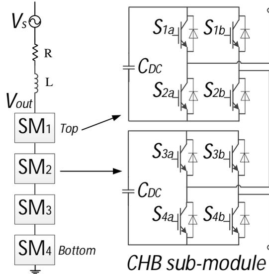
Fig. 2.16 One arm of a 5-level CHB-MMCC circuit
