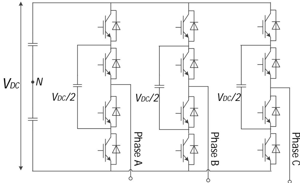
Fig. 1.13 3-phase 5-level FCC converter topology
