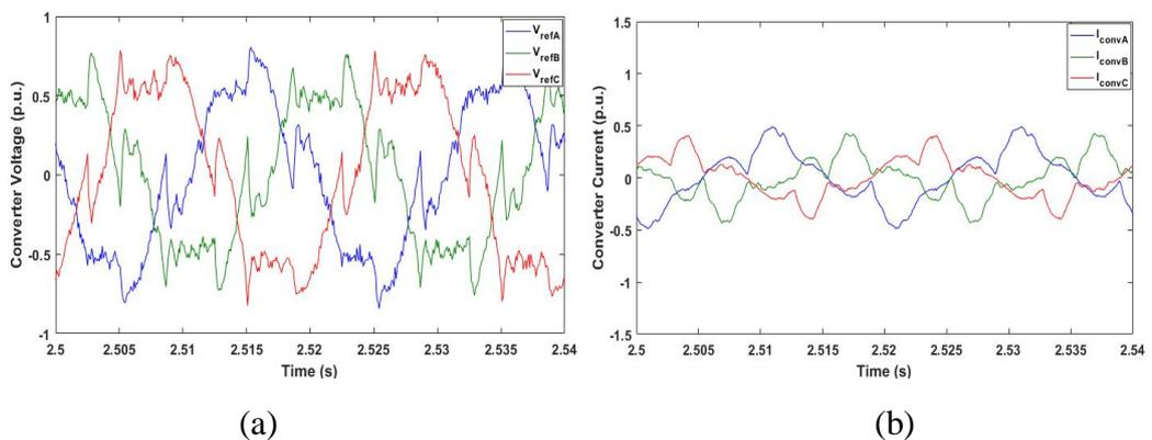
Fig. 5.17 3-phase converter (a)reference voltage and (b)current
