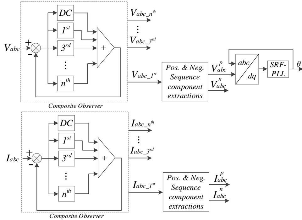
Fig. 4.7 Composite observer-based scheme
