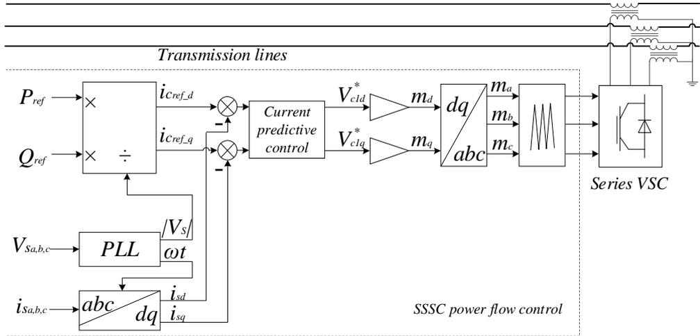
Fig. 6.8 SSSC power flow control block diagram
