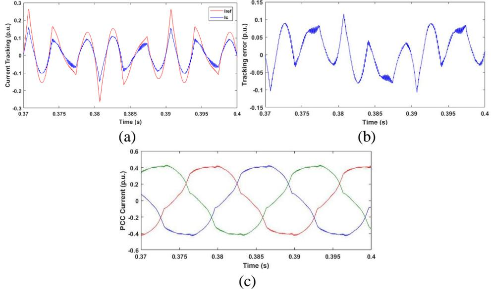
Fig. 3.16 (a) Simulated converter current reference tracking waveforms; (b) Reference tracking error; (c) Three-phase source current at PCC
