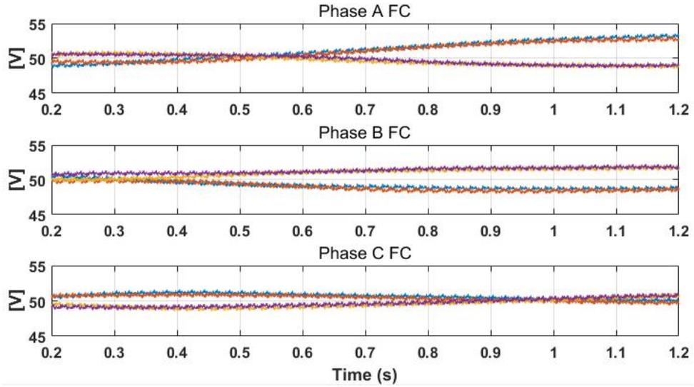
Fig. 3.21 SM FC voltages with conventional PS-PWM
