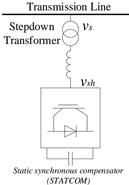
Fig. 1.2 Static synchronous compensator (STATCOM)
