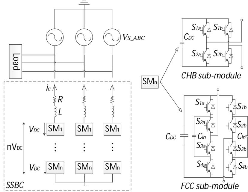
Fig. 2.6 Single star bridge cell
