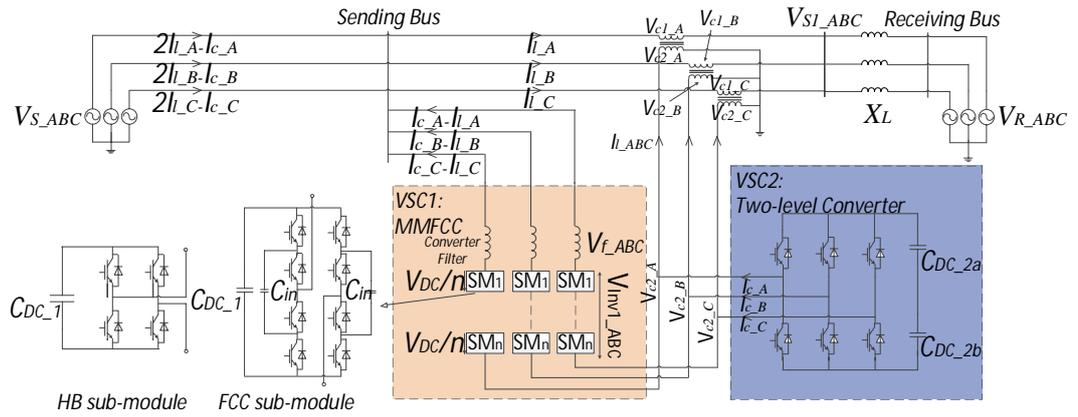
Fig. 6.11 3-phase transmission system with novel MMCC-UPFC circuit diagram
