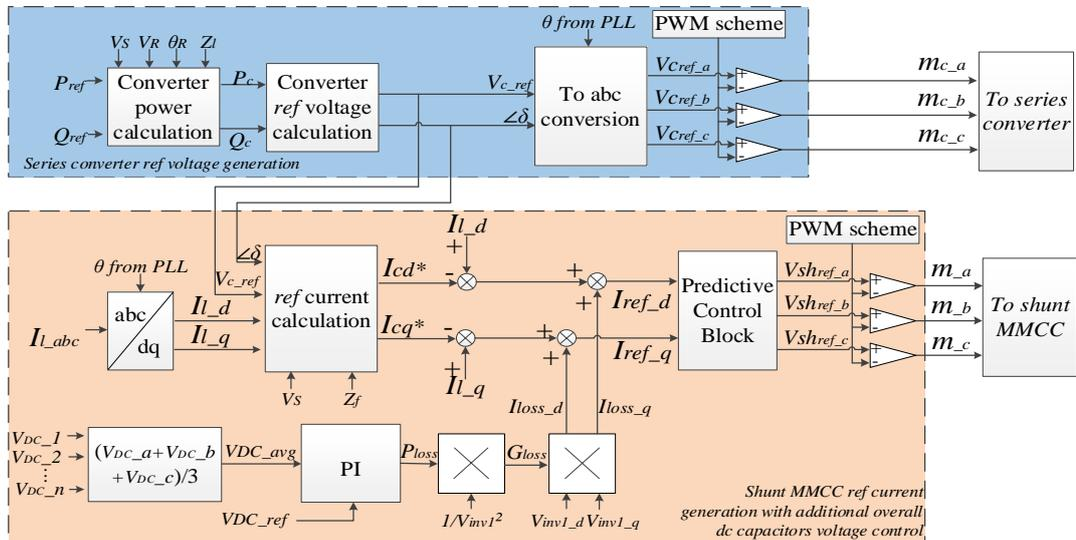
Fig. 6.15 MMCC-UPFC control block diagram
