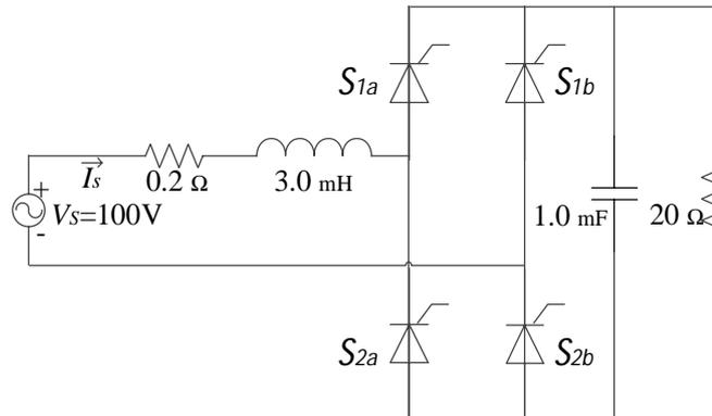
Fig. 3.5 Single-phase thyristor controlled rectifier circuit
