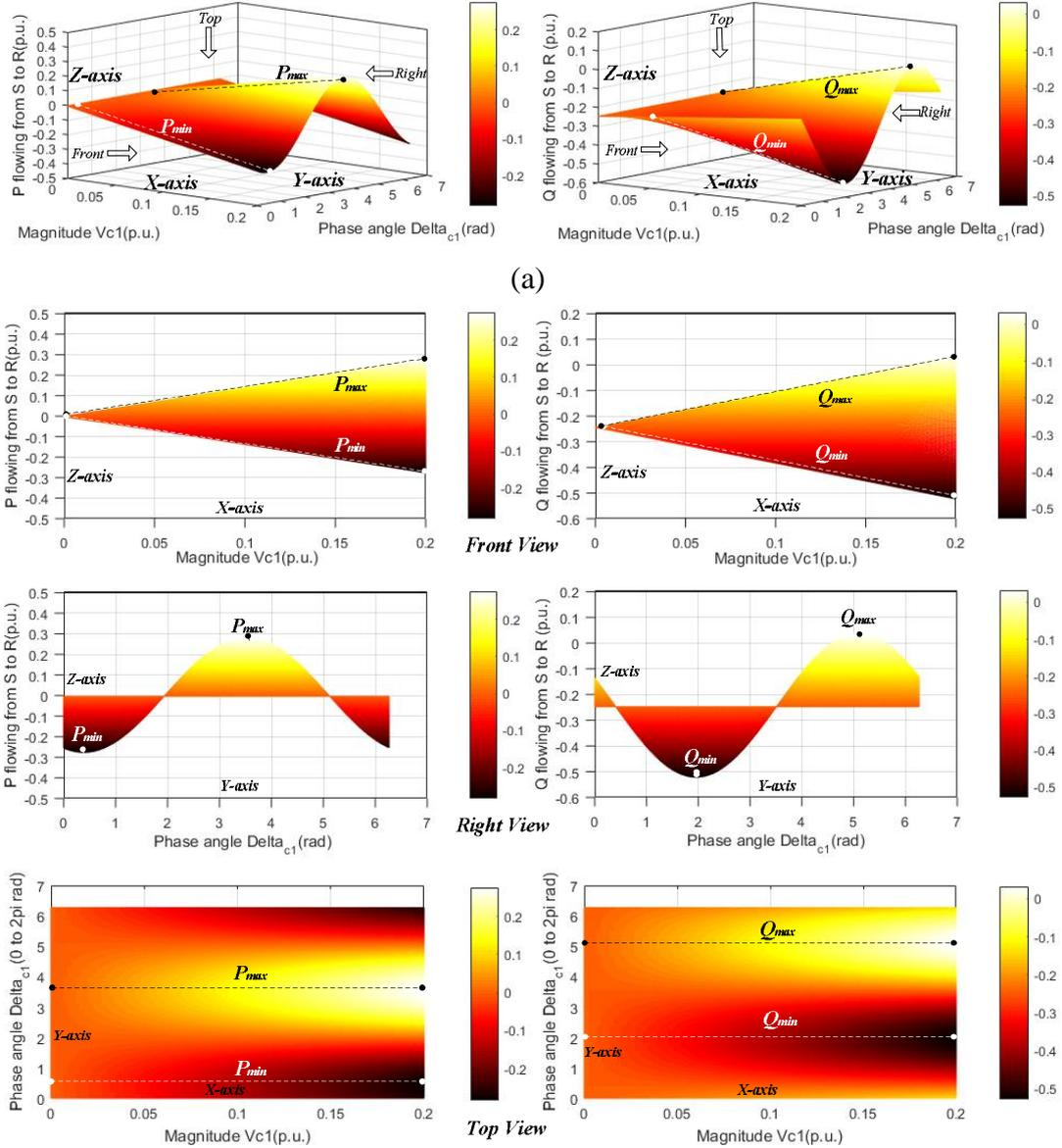
Fig. 6.7 (a) 3-D Plot of power flow margin of transmission line with SSSC operation
