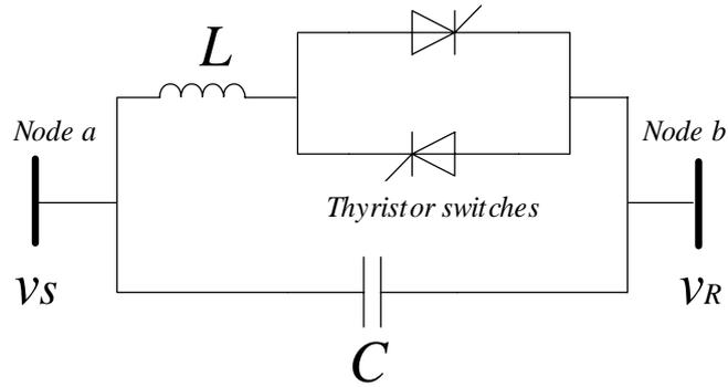
Fig. 1.5 Thyristor controlled series capacitor (TCSC)
