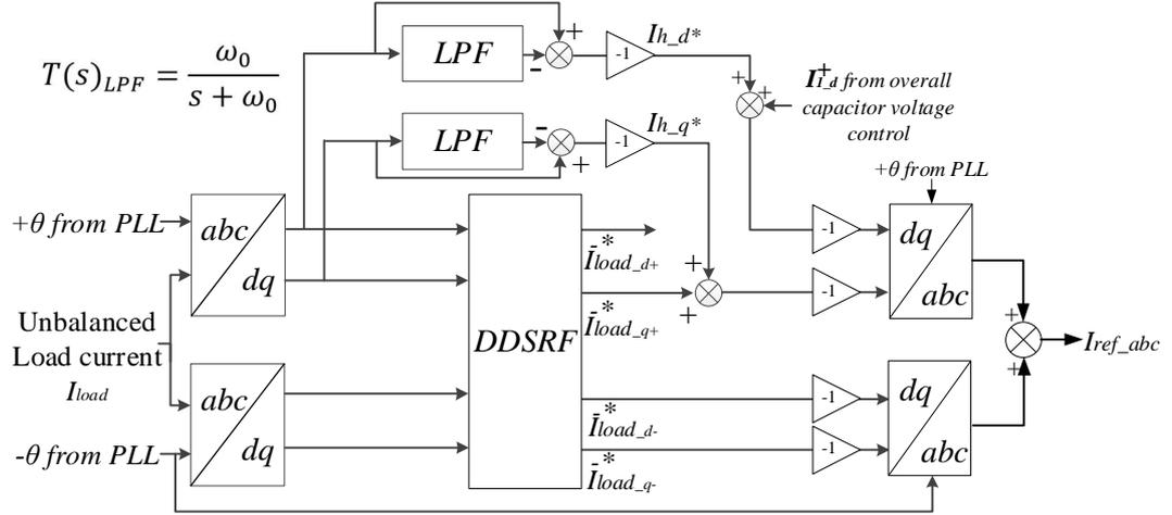
Fig. 4.9 LPF-based harmonic and reactive power extraction scheme
