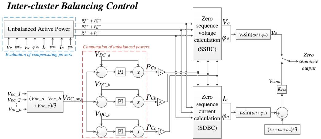
Fig. 4.18 Block diagram of Inter-cluster voltage Balancing control
