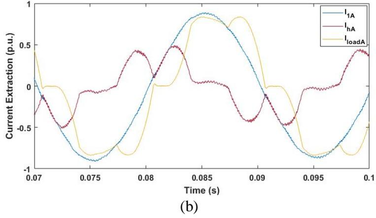
Fig. 3.14 (a) Harmonic extraction and reactive power compensation control block and (b) corresponding current harmonics extraction from phase A load current
