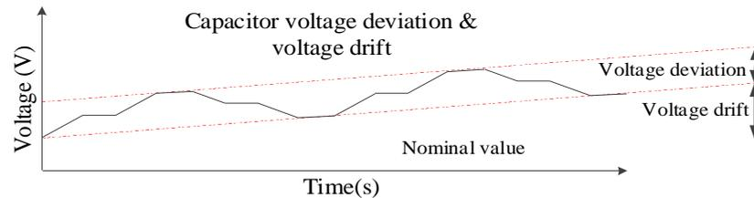
Fig. 3.18 Capacitor voltage drift and voltage deviation diagram
