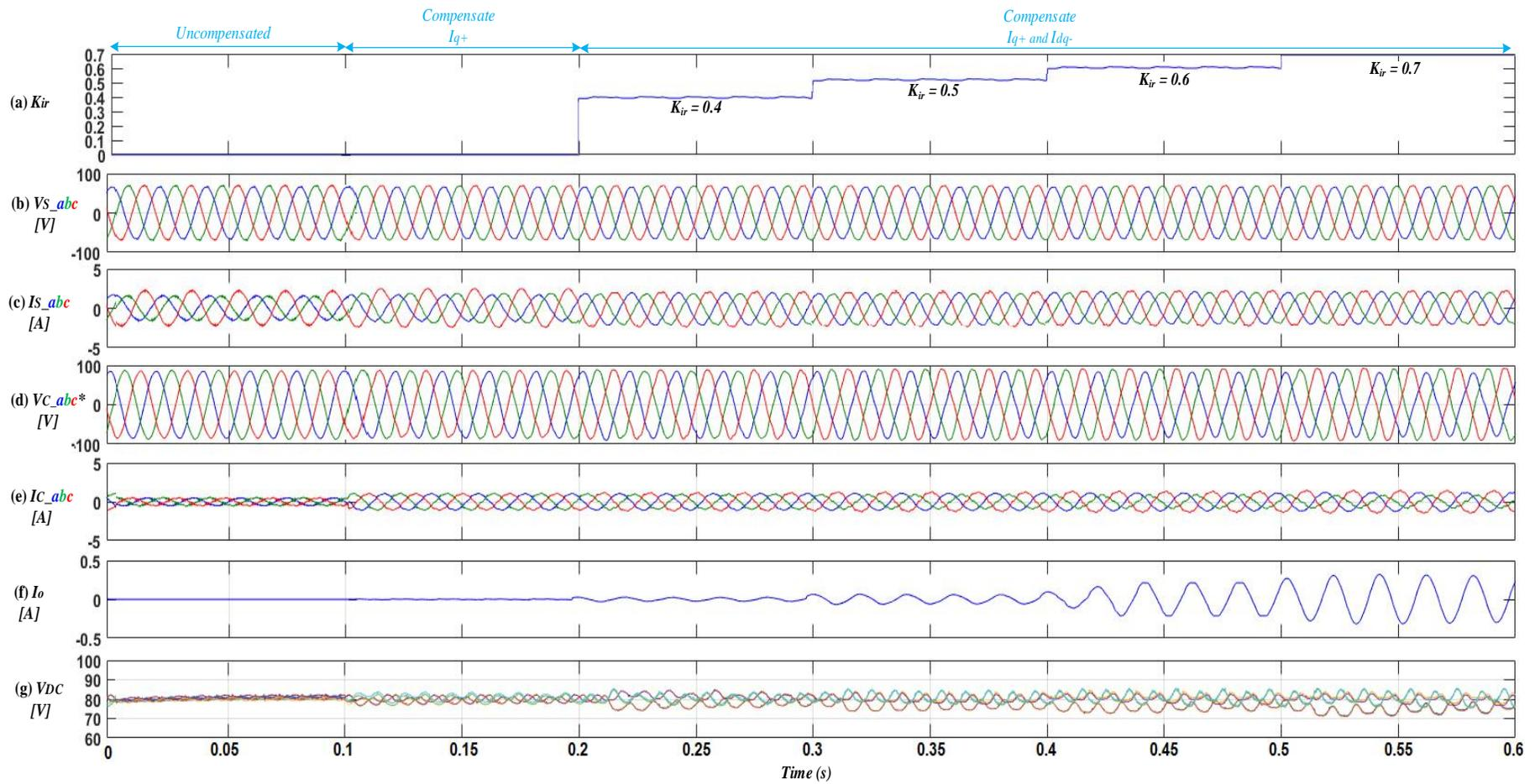
Fig. 5.21 SDBC Compensation of load current imbalance without harmonics
