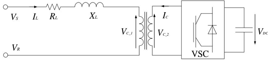
Fig. 6.5 Single line system with VSC-SSSC circuit
