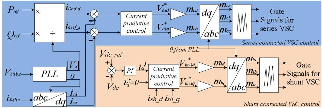
Fig. 6.10 UPFC control system blocks diagram
