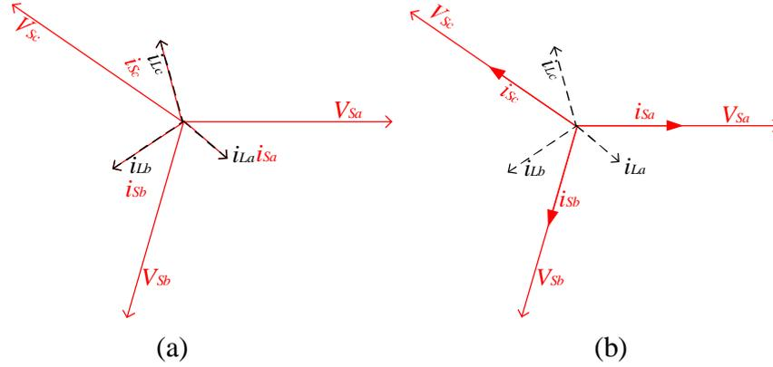
Fig. 4.6 The phasor diagram of (a) 3-phase network voltage and unbalanced current and (b) when it achieves rebalanced current and unity power factor
