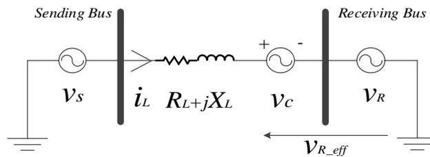
Fig. 6.3 Single line diagram with injected series voltage
