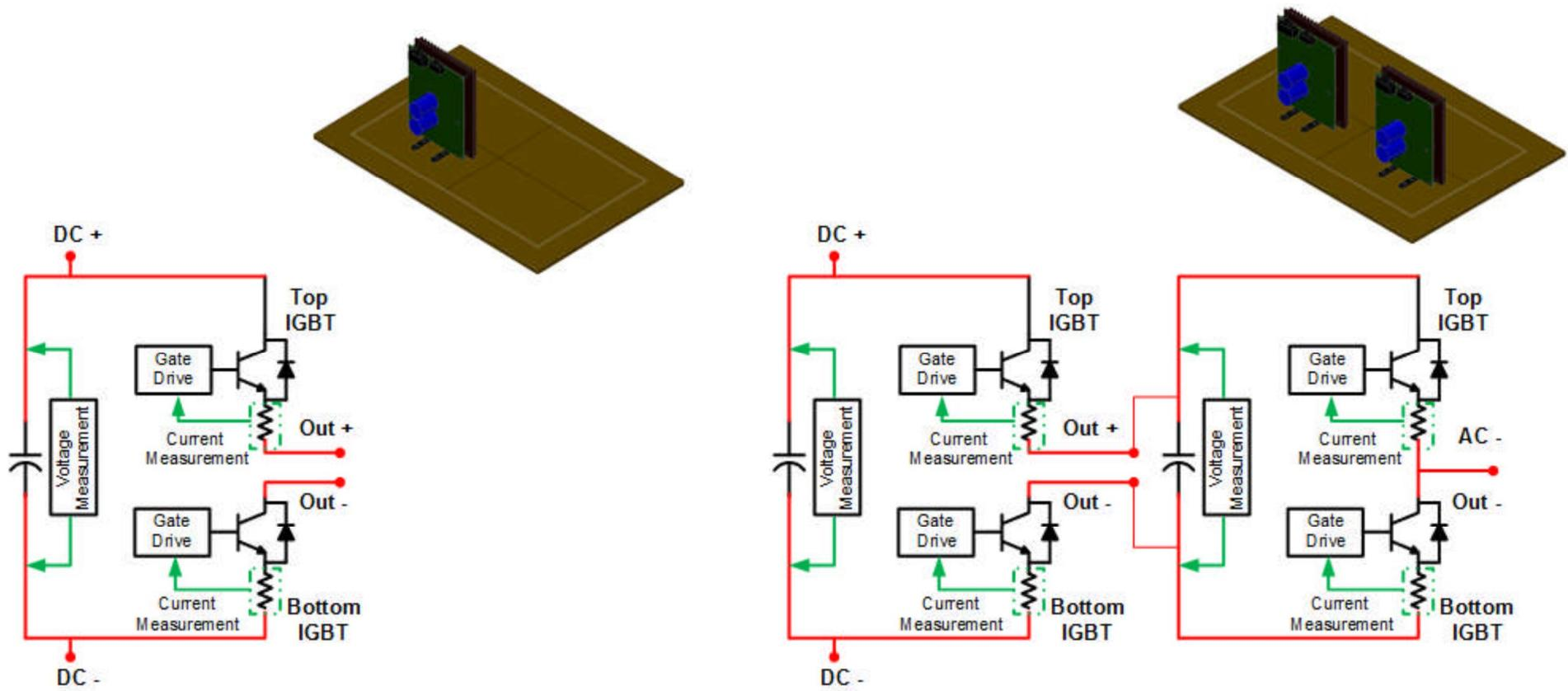
Fig. 5.2 (a) FC half-bridge cell and (b) 3-level FC half-bridge
