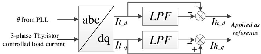
Fig. 3.10 LPF current harmonics extraction block diagram
