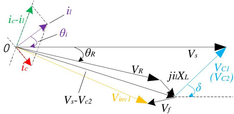
Fig. 6.13 UPFC voltage and current phasor diagram
