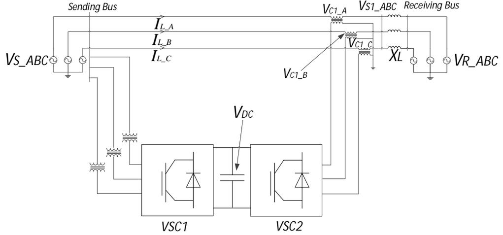
Fig. 6.1 VSC-based UPFC circuit diagram
