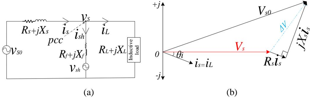
Fig. 1.3 (a) Simplified circuit of a balanced power network; (b) the circuit phasor diagram without STATCOM compensation
