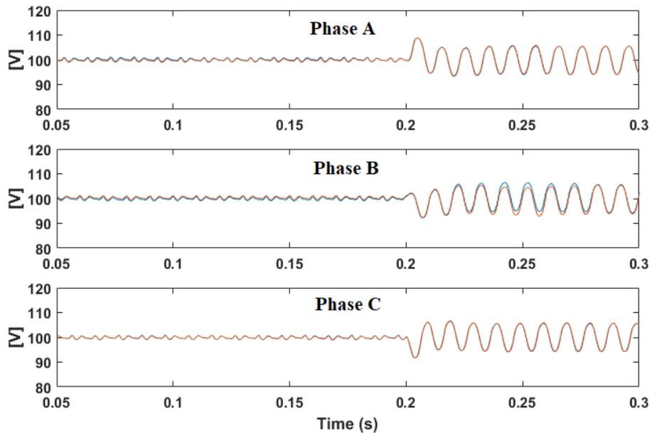
Fig. 3.35 Submodule DC capacitors voltage waveforms
