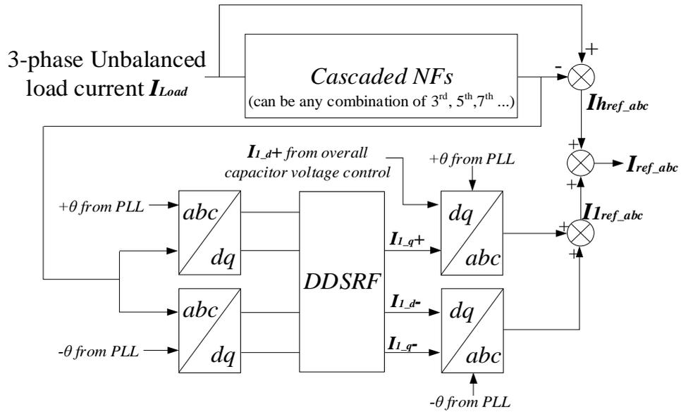
Fig. 4.12 NF-based harmonic extraction and reactive power compensation extraction scheme
