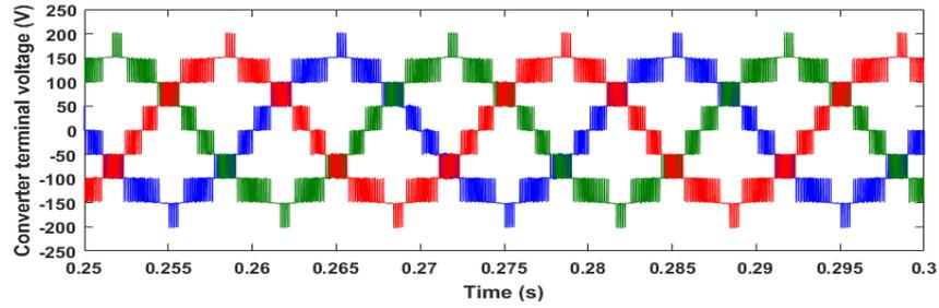
Fig. 3.29 3-phase converter voltage waveforms
