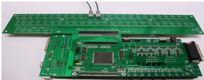
Fig. 5.6 FPGA cards connected with fibre optic breakout board
