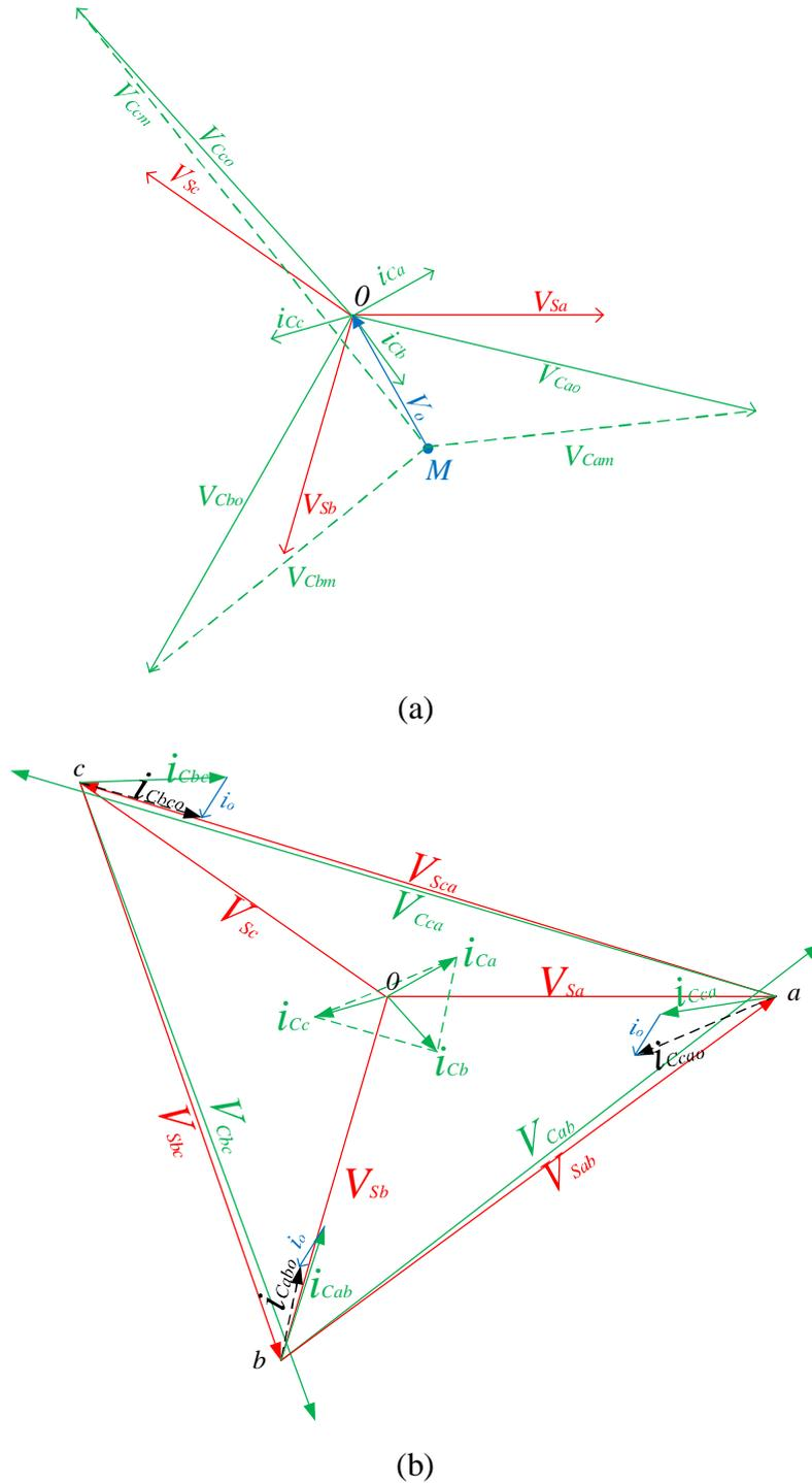
Fig. 4.17 3-phase voltage and current phasor diagram with (a) zero sequence voltage injection for SSBC and (b) zero sequence current injection for SDBC
