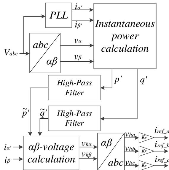
Fig. 4.8 Instantaneous reactive power theory-based scheme
