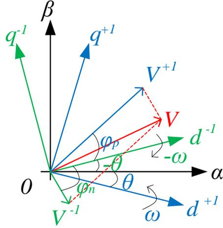
Fig. 1.18 Double synchronous reference frames
