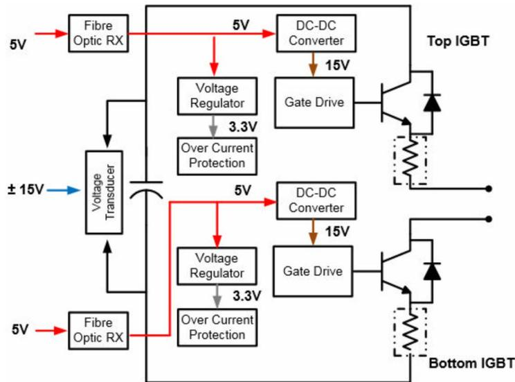
Fig. 5.5 Cell card power supply layout
