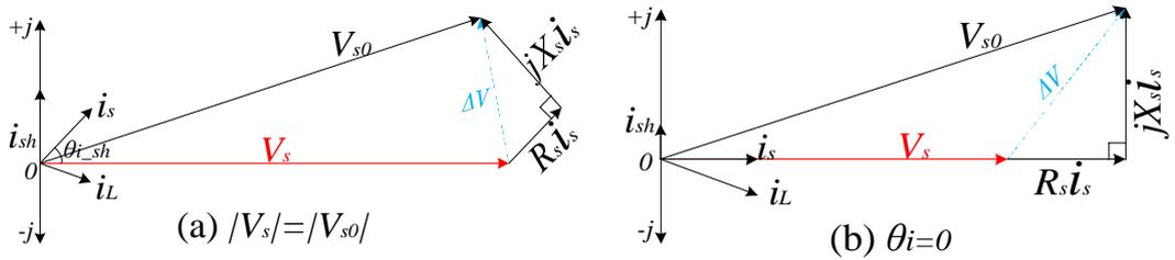
Fig. 1.4 STATCOM reactive power compensations: (a) Voltage regulation and (b) unity power factor
