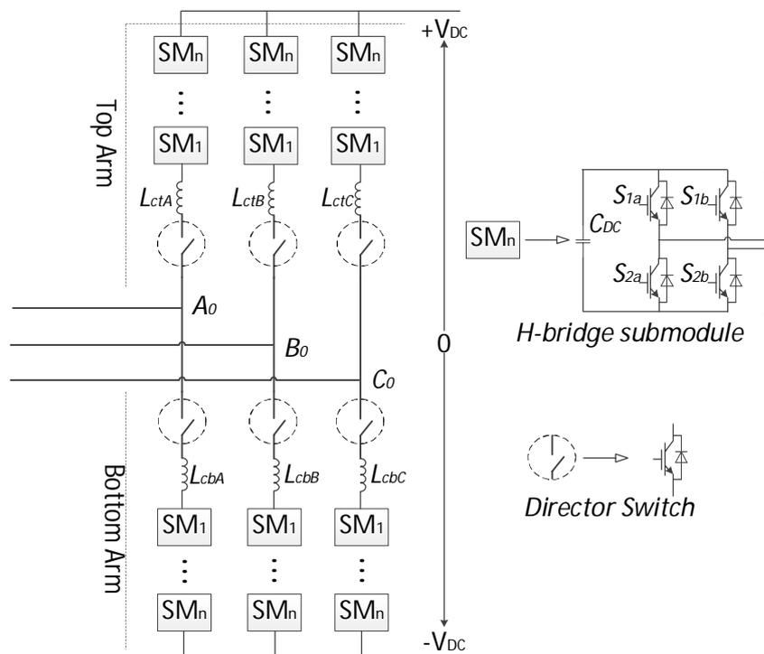
Fig. 2.10 Alternate Arm Converter (AAC) schematic diagram
