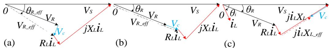
Fig. 6.4 Power flow control phasor diagrams: (a) phase shifting and real power control; (b) voltage magnitude and reactive power control; (c) line impedance control
