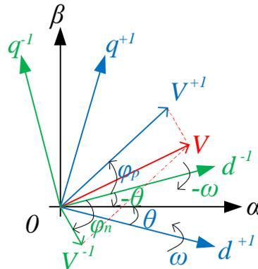
Using the Clarke transformation, the unbalanced voltage vector can be given as
