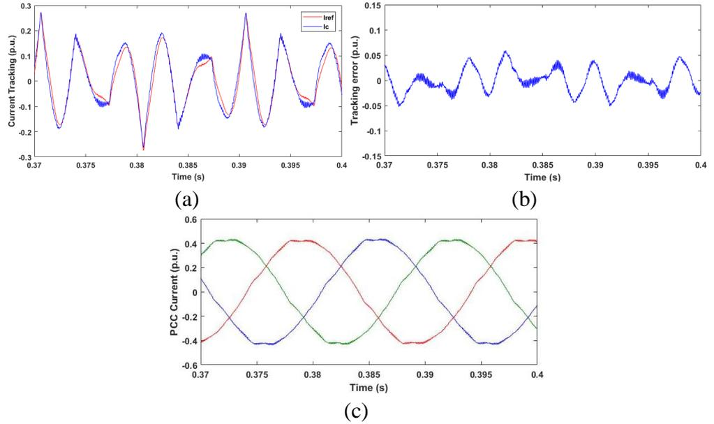
Fig. 3.17 (a) Simulated converter current reference tracking waveforms; (b) Reference tracking error; (c) Three phase source current at PCC with modification ( $\tau = 0.02$ )
