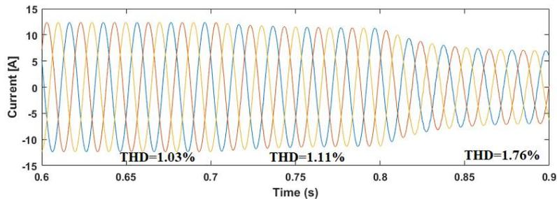
Fig. 3.11 LPF filtered result for 3-phase harmonics current
