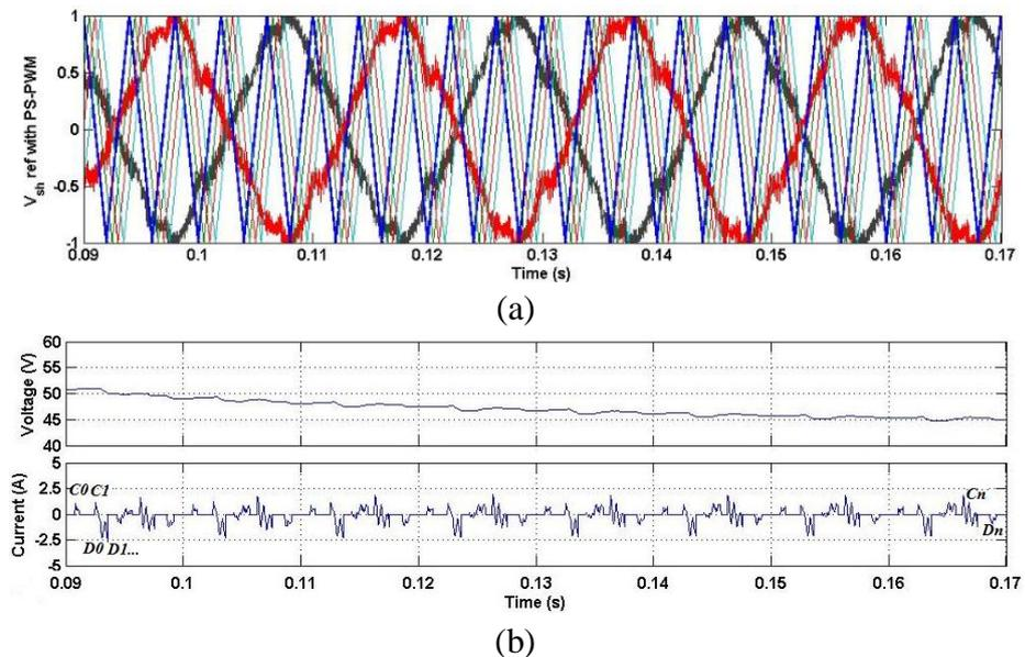
Fig. 3.20 (a) Voltage reference signal for MMFCC with conventional PS-PWM and (b) corresponding MMFCC-APC phase A intra-cluster upper SM flying capacitor  $C_{SM1a}$  actions in 4 cycles
