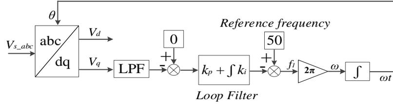
Fig. 1.16 SRF-PLL block diagram
