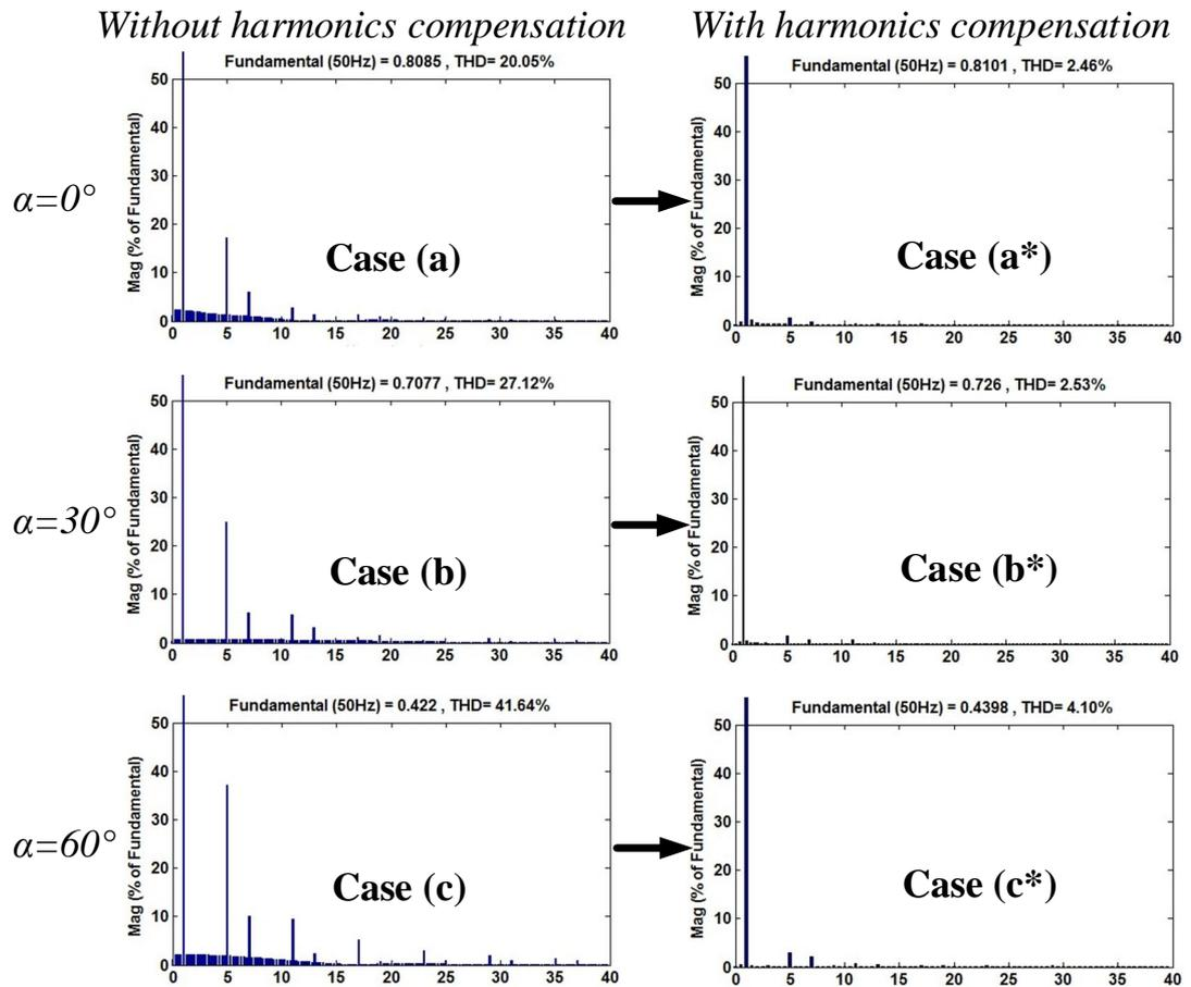
Fig. 3.27 Source harmonic current spectra for different simulation scenarios
