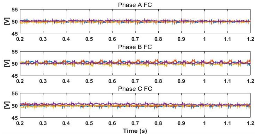
Fig. 3.23 SM FC voltages with CP PS-PWM
