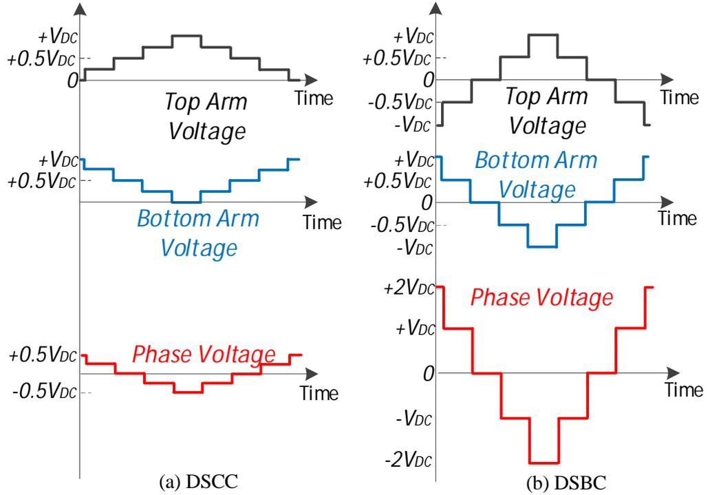
Fig. 2.9 Voltage waveforms of top, bottom arms and phase voltage for (a) DSCC and (b) DSBC
