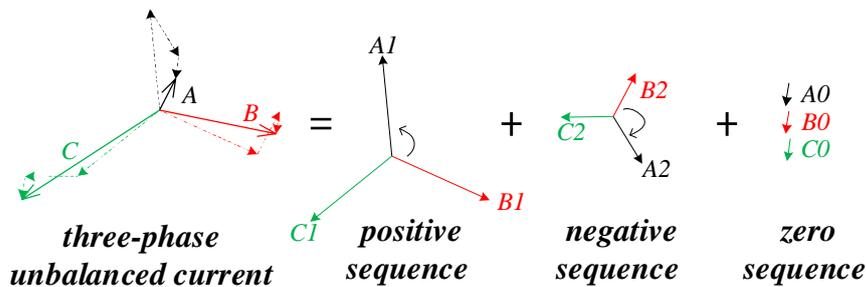
Fig. 4.5 Three-phase unbalanced current with its symmetrical components
