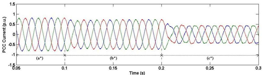
Fig. 3.26 Compensated PCC source current when  $\alpha$  changes from  $0^\circ$  to  $60^\circ$
