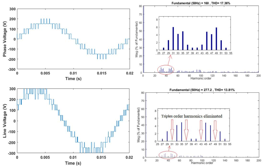
Fig. 2.19 5-level MMCC output phase voltage (upper) and line voltage (bottom) with their harmonics spectra for PD-PWM when  $f_s=1$  kHz
