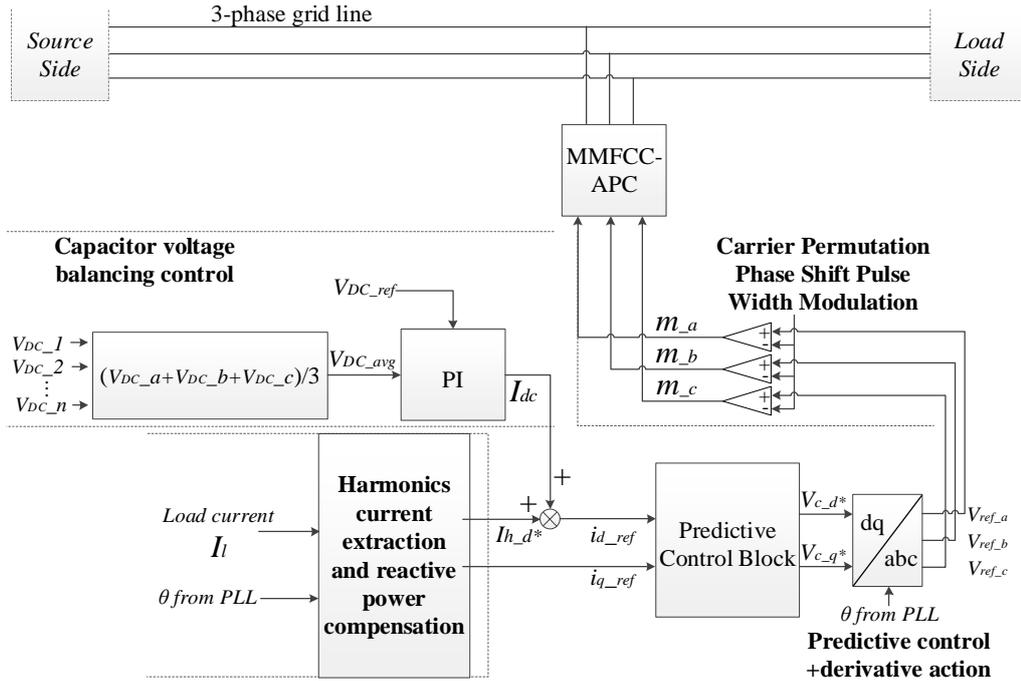
Fig. 3.13 Control schemes of the APC system
