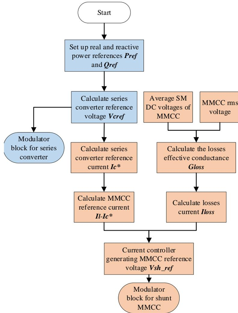
Fig. 6.16 Flowchart of MMCC-UPFC control schemes
