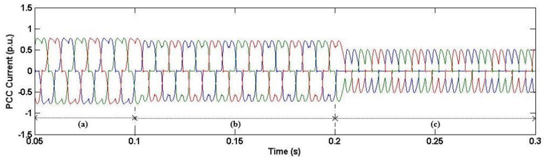
Fig. 3.25 Uncompensated PCC source current when  $\alpha$  changes from  $0^\circ$  to  $60^\circ$
