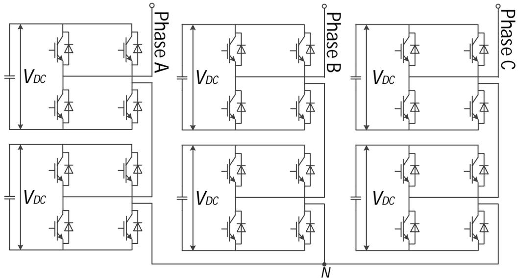
Fig. 1.12 3-phase 5-level CHB converter topology
