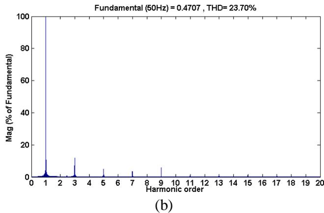
Fig. 3.4 (a) Desktop PC steady-state current waveform and (b) its harmonic spectrum
