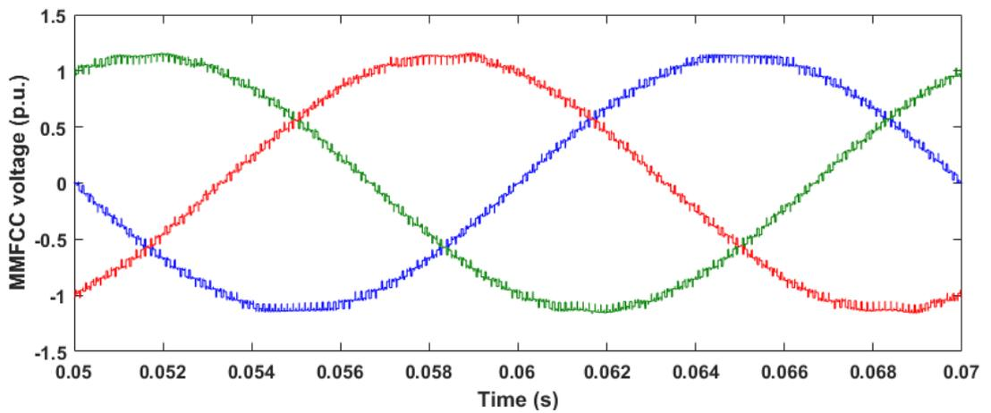
Fig. 6.21 3-phase MMFCC multilevel voltage waveform
