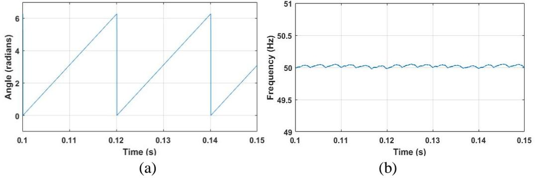
Fig. 1.17 SRF-PLL output (a) angle  $\theta=\omega t$  and (b) frequency  $f_1=50\text{Hz}$
