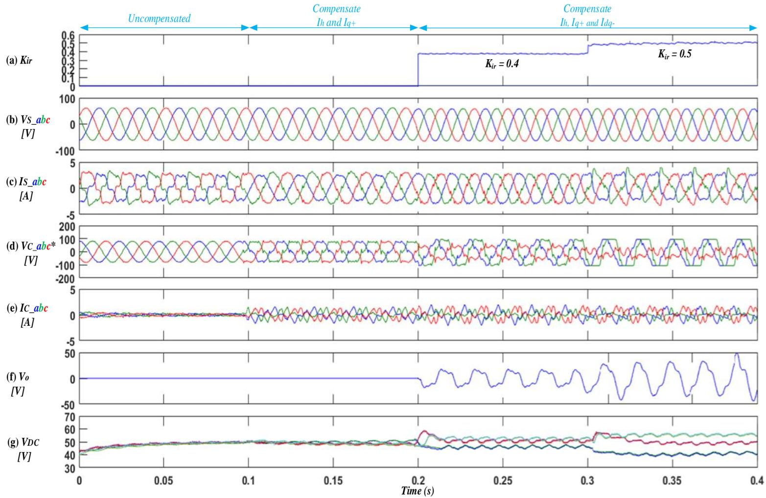
Fig. 5.20 SSBC Compensation of both load current harmonics and imbalance
