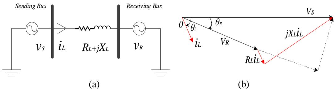
Fig. 6.2 (a) Single line diagram with two voltage source ends and (b) corresponding phasor diagram
