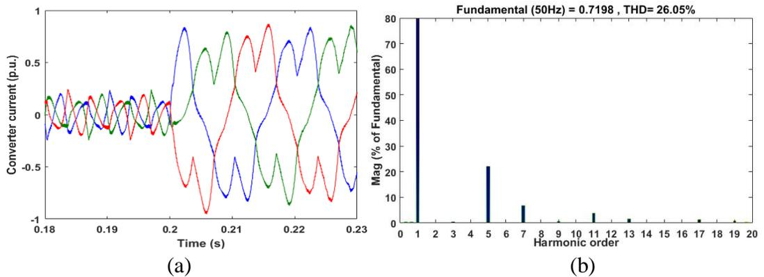
Fig. 3.34 (a) APC current waveforms (b) harmonic spectrum (during 0.21-0.23sec)
