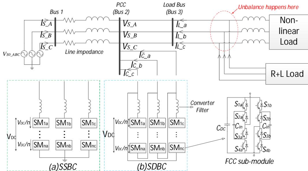
Fig. 4.14 3-phase MMFCC-APC system with (a) SSBC and (b) SDBC configuration
