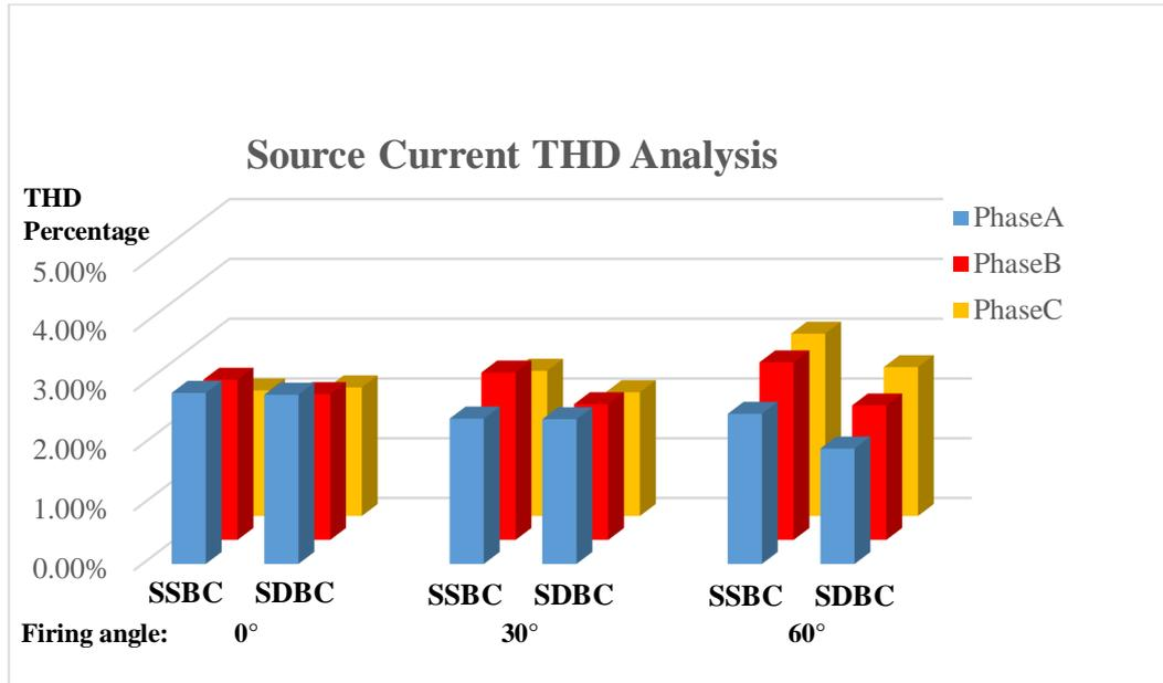
Fig. 4.28 The THDs of the 3-phase source current for Case B
