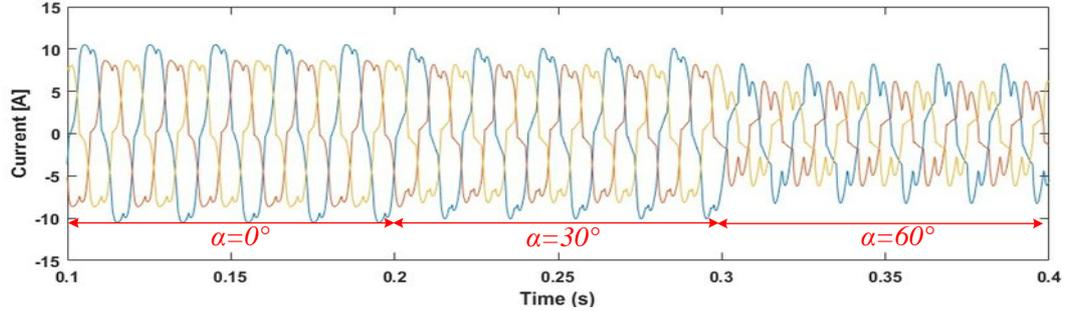
Fig. 4.2 AC current waveforms when  $\alpha$  changes from  $0^\circ$  to  $60^\circ$  for Case A
