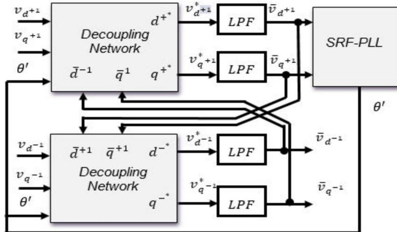
Fig. 1.19 Block diagram of Decoupled Double Synchronous Reference Frame-PLL
