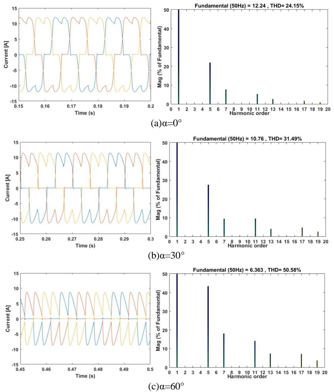
Fig. 3.8 AC current waveform and its harmonic spectrum when (a)  $\alpha=0^\circ$ ; (b)  $\alpha=30^\circ$ ; (c)  $\alpha=60^\circ$
