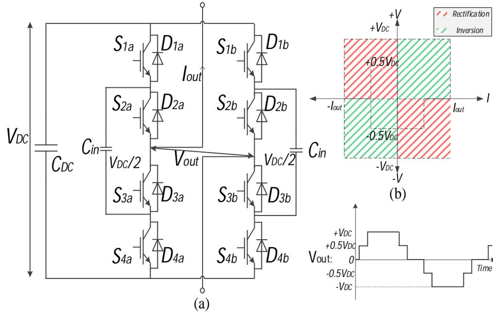
Fig. 2.4 (a) Full-bridge FCC SM circuit; (b) Operating quadrant
