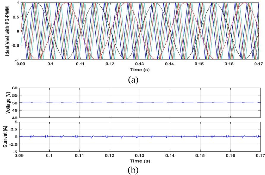
Fig. 3.19 (a) Ideal voltage reference signal for MMFCC with conventional PS-PWM and (b) corresponding MMFCC-APC phase A intra-cluster upper SM flying capacitor  $C_{SM1a}$  actions in 4 cycles
