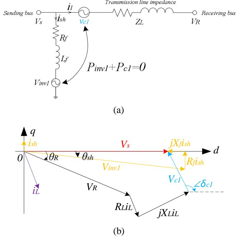
Fig. 6.9 UPFC (a) simplified circuit and (b) its phasor diagram
