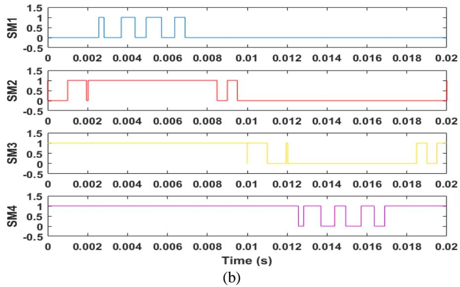
Fig. 2.18 Four phase disposed carriers for 5-level CHB-MMCC
