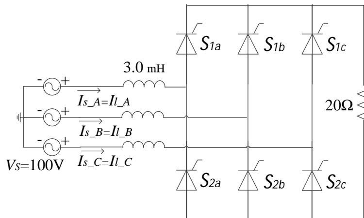
Fig. 3.7 3-phase thyristor controlled rectifier circuit
