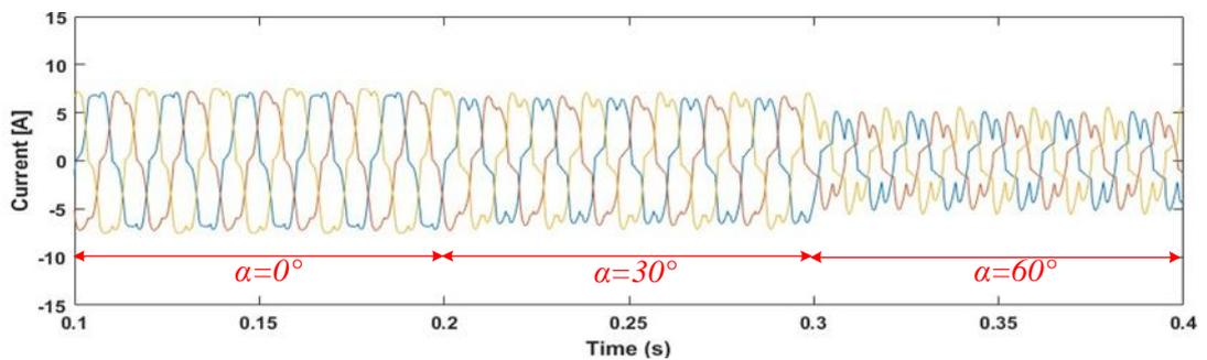
Fig. 4.4 AC current waveforms when  $\alpha$  changes from  $0^\circ$  to  $60^\circ$  for Case C
