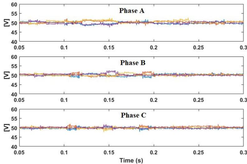
Fig. 3.31 Submodule inner flying capacitors voltage waveforms
