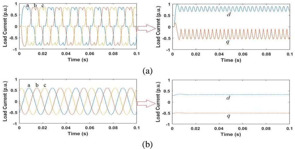
Fig. 3.9 Thyristor controlled rectifier load current from  $abc$  to  $dq$  transformation waveforms
