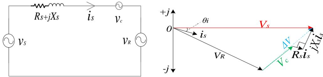
Fig. 1.7 (a) Simplified circuit of a balanced power network with SSSC connection and (b) the corresponding phasor diagram
