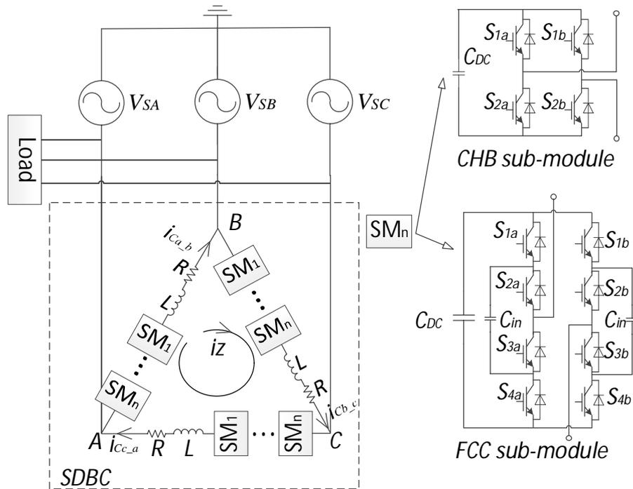
Fig. 2.7 Single delta bridge cell
