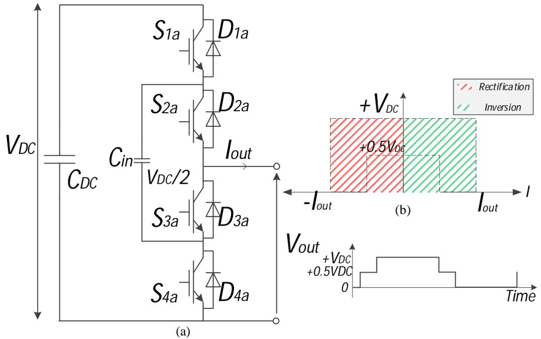
Fig. 2.3 (a) FC half-bridge SM circuit; (b) Operating quadrant
