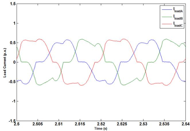
Fig. 5.16 3-phase load current
