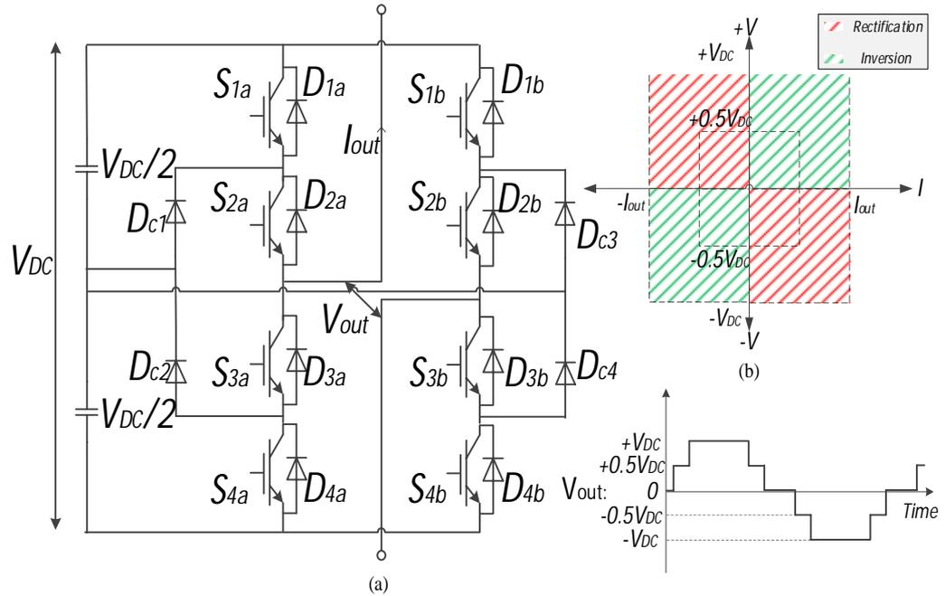
Fig. 2.5 (a) NPC SM circuit; (b) Operating quadrant
