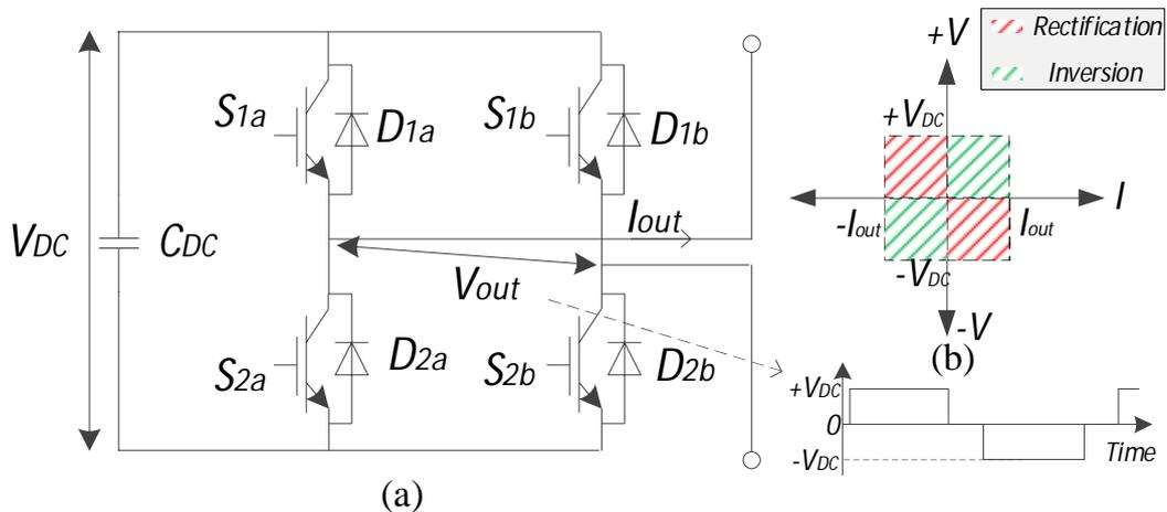
Fig. 2.2 (a) H-bridge SM circuit; (b) Operating quadrants
