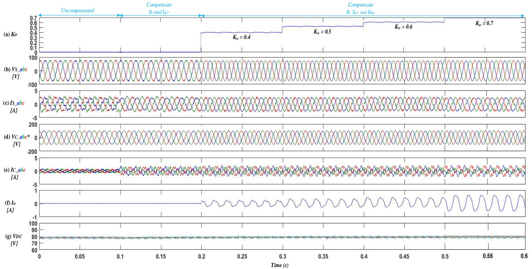
Fig. 5.22 SDBC Compensation of both load current harmonics and imbalance
