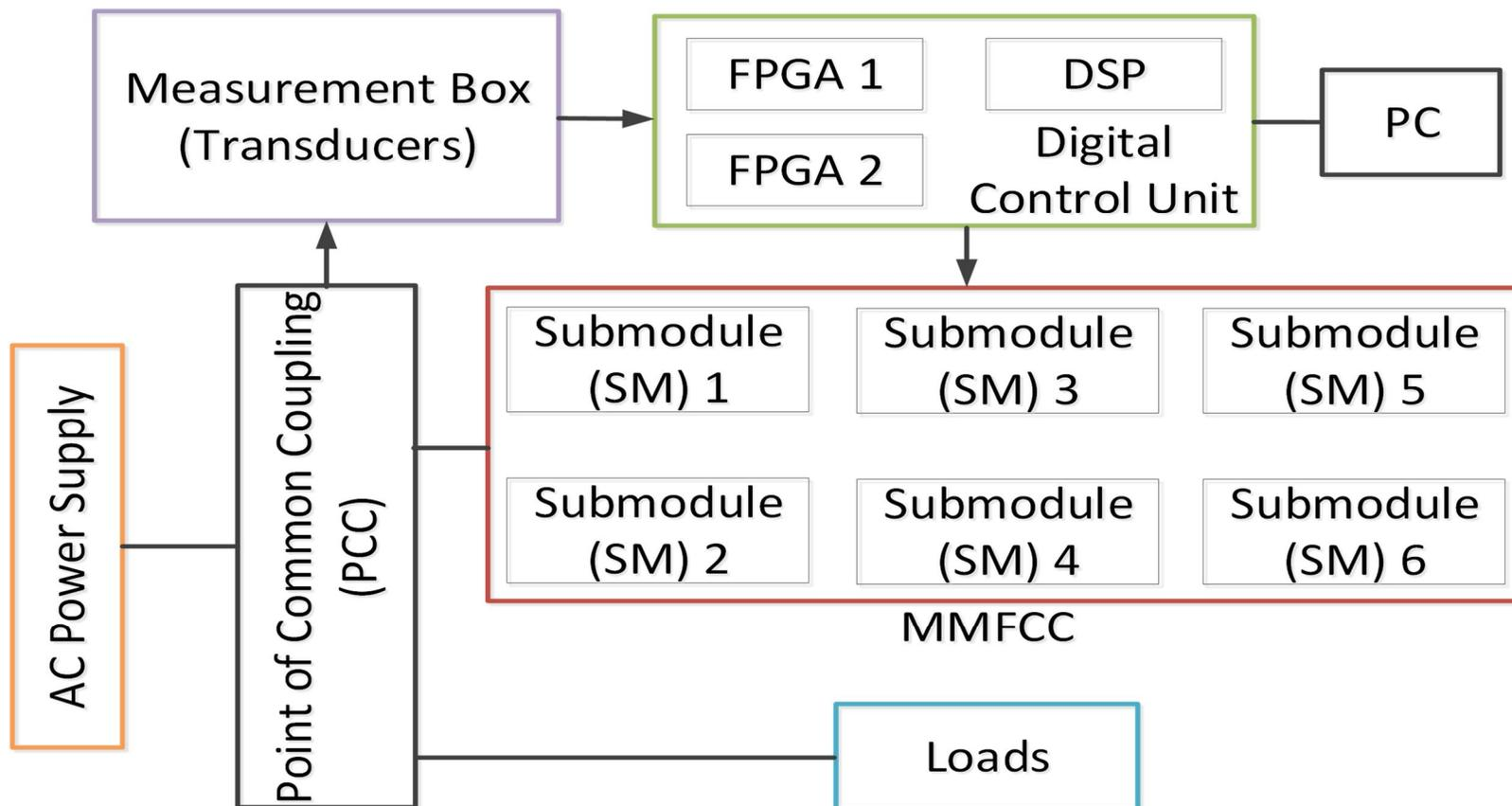
Fig. 5.1 Hardware block diagram
