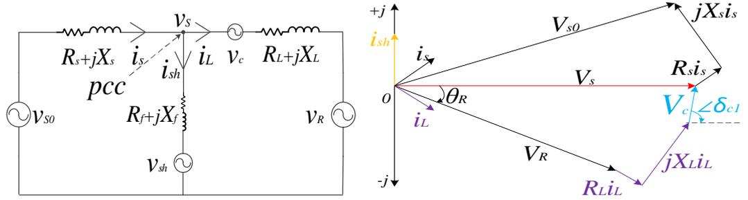
Fig. 1.9 (a) Simplified circuit of a balanced power network with UPFC system and (b) the corresponding phasor diagram
