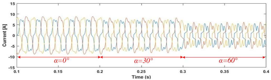
Fig. 4.3 AC current waveforms when  $\alpha$  changes from  $0^\circ$  to  $60^\circ$  for Case B
