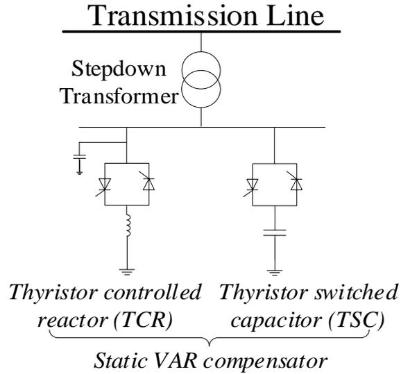
Fig. 1.1 Static VAR Compensator
