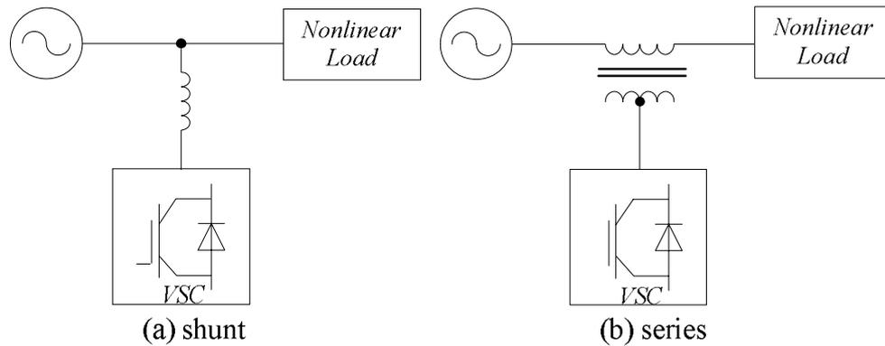
Fig. 1.10 Active Power Filter configurations
