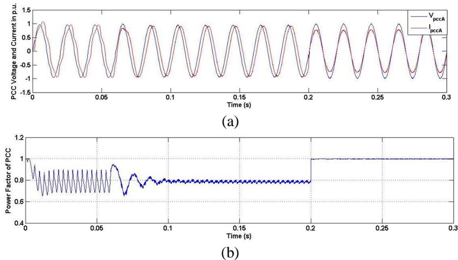
Fig. 3.33 (a) PCC voltage and current and (b) PCC power factor variation with both harmonics control and reactive power compensation
