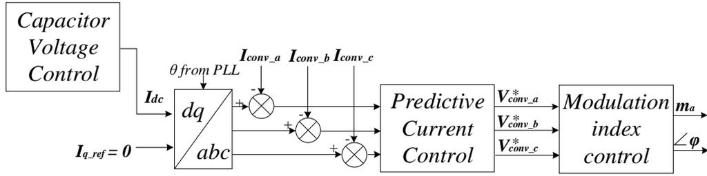
Fig. 5.13 Capacitor pre-charge control block
