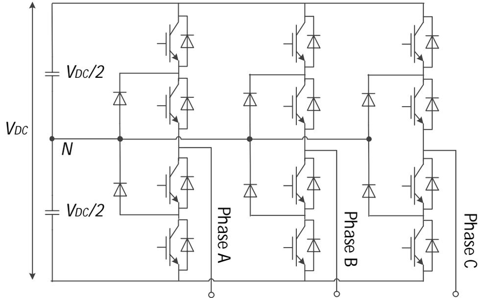
Fig. 1.11 3-phase 5-level NPC converter topology
