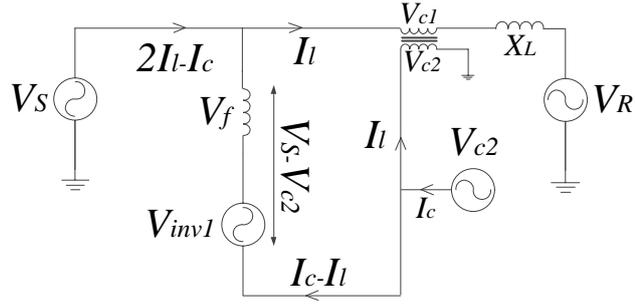
Fig. 6.12 MMCC-UPFC equivalent circuit
