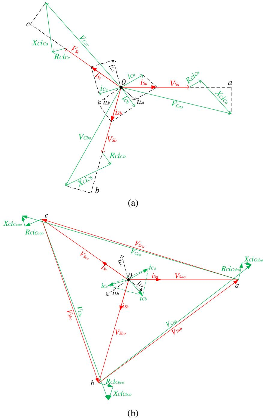
Fig. 4.15 phasor diagrams for 3-phase voltages and currents in controlled by MMCC-APC in (a) SSBC and (b) SDBC connection
