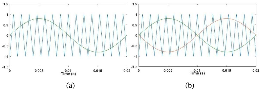
Fig. 2.13 (a) Bipolar PWM and (b) Unipolar PWM when  $M_a=0.8$ ,  $M_f=15$
