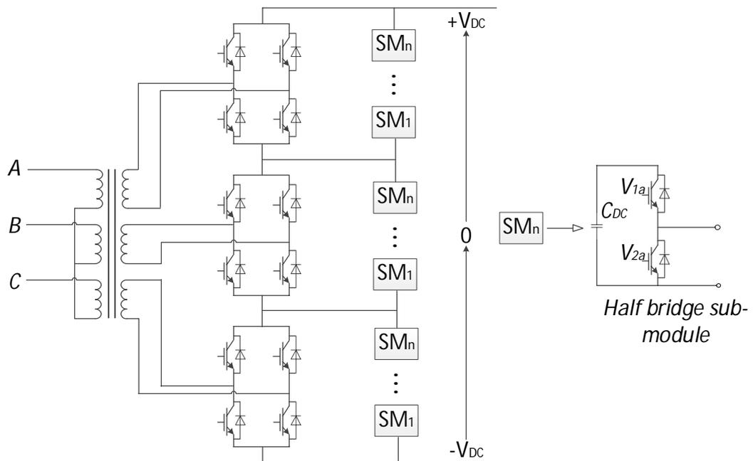
Fig. 2.11 Series Bridge Converter (SBC) schematic diagram
