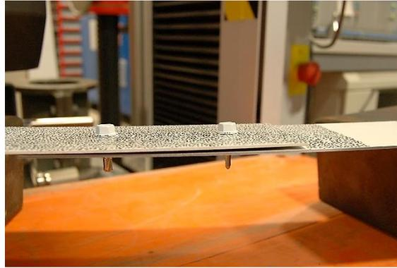
**Figure 6.13: Small gap between steel sheets of specimen SCS14-14**
