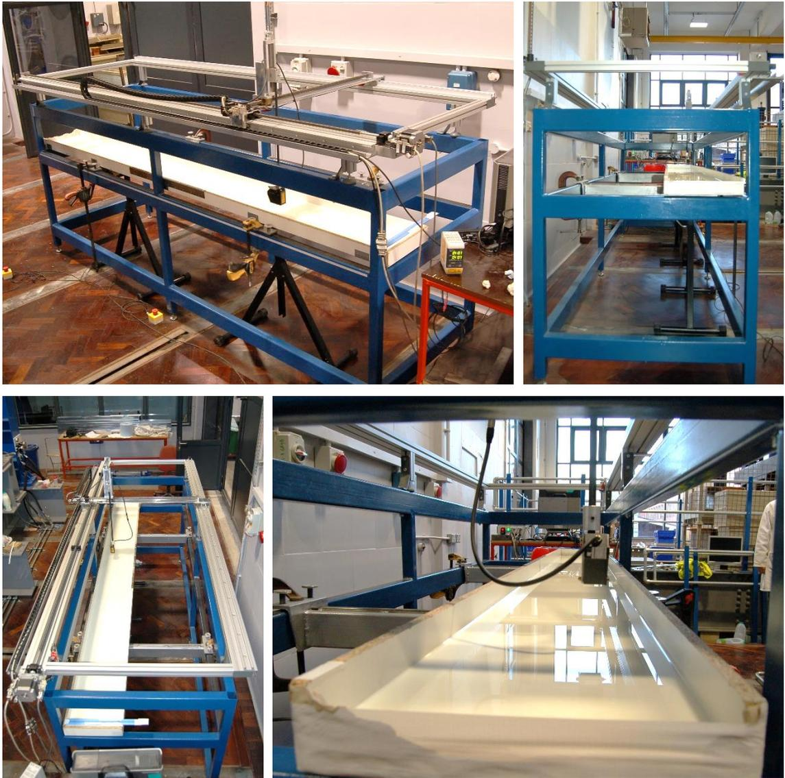
**Figure 5.59: Calibration of the imperfection measuring rig**
