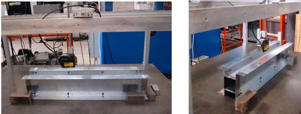
Figure 3.25: Measurement of the imperfections of built-up column 2
