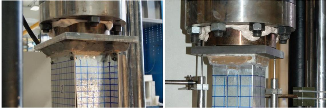
Figure 3.35: Plaster used to correct misalignment between the platen of the machine and the column end plate
