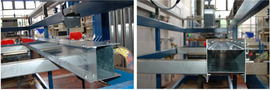
**Figure 5.21: Measurement of the imperfections of built-up column 1**
