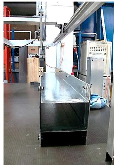
Figure 3.23: Measurement of the imperfections of built-up column 1
