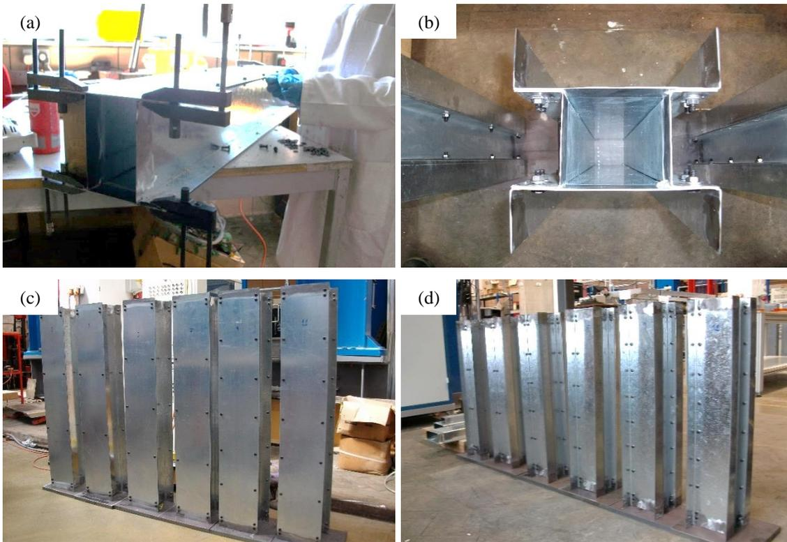
Figure 3.17: Images of built-up columns 1 and 2 during and after assembly
