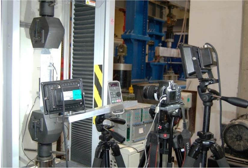
Figure 6.5: Camera and lamp arrangement for DIC
