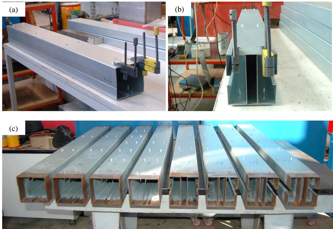
**Figure 3.19: Images of built-up columns 3 and 4 during and after assembly**
