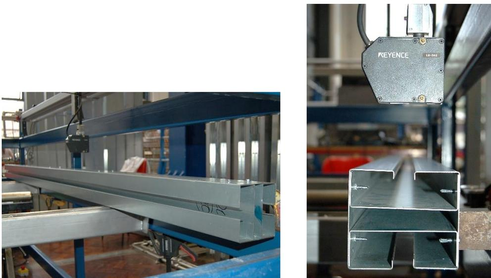
Figure 5.27: Measurement of the imperfections of built-up column 4
