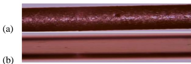
Figure 7-2. Images of (i) roughened and (ii) ‘smooth’ optical fibres recorded by the microscope (AZ100 multizoom, Nikon metrology, UK).
