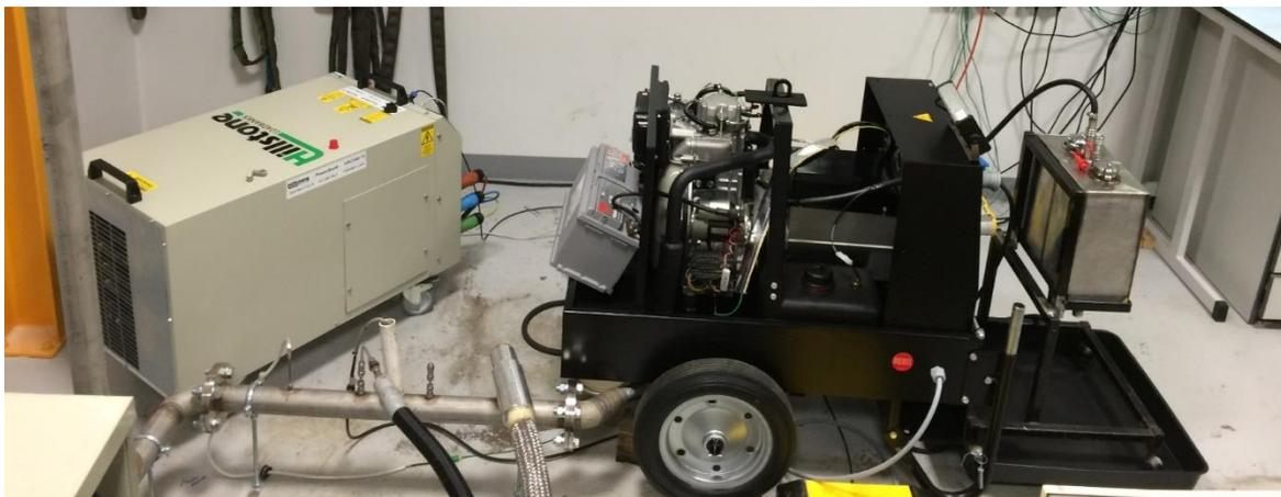
Figure 3-8 Engine generator setup used for char-slurry tests
