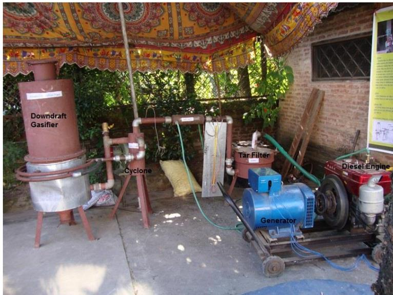
Figure 8-4 An example of a diesel generator converted to run on syngas.
