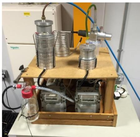
Figure 3-11 Andersen cascade impactor (cylinder on the left) and single stage filter (smaller cylinder right)
