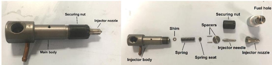
*Figure 3-9 Injector used in the diesel engine selected. a) Assembled injector, and b) disassembled injector. Note- an extra nozzle is shown in b) for views at two angles.*
