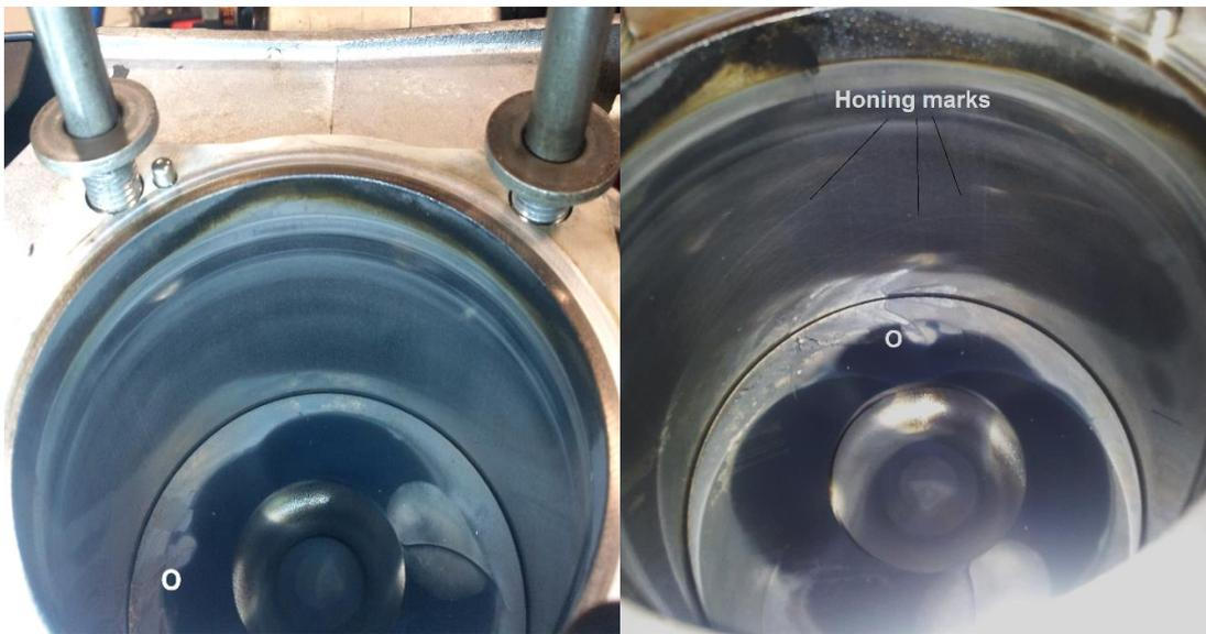
*Figure 7-4 Inspection of the internal surfaces of the engine cylinder after failure. O denotes a common point on the surface of the piston to show orientation.*
