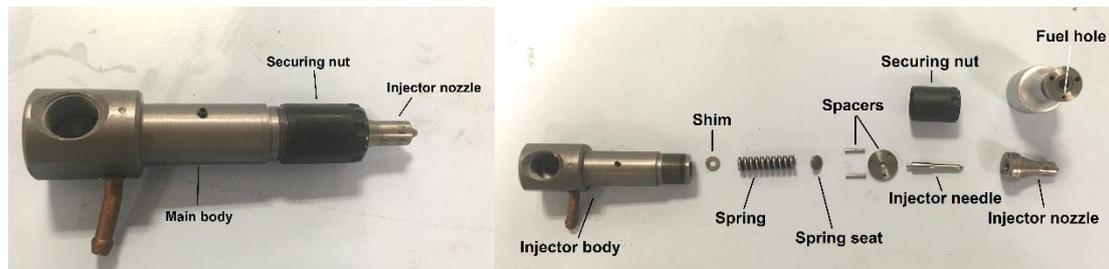
*Figure 3-9 Injector used in the diesel engine selected. a) Assembled injector, and b) disassembled injector. Note- an extra nozzle is shown in b) for views at two angles.*
