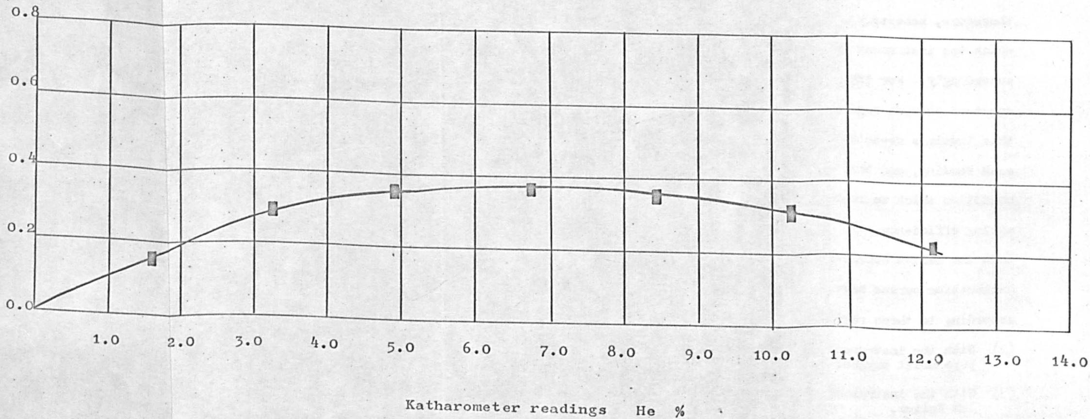
Fig. 4 Calibration of the Katharometer
