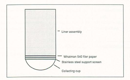
Figure 2.5 Centrifuge liner assemblies for extracting porewater from PFA (Modified after Edmunds and Bath (1976)
