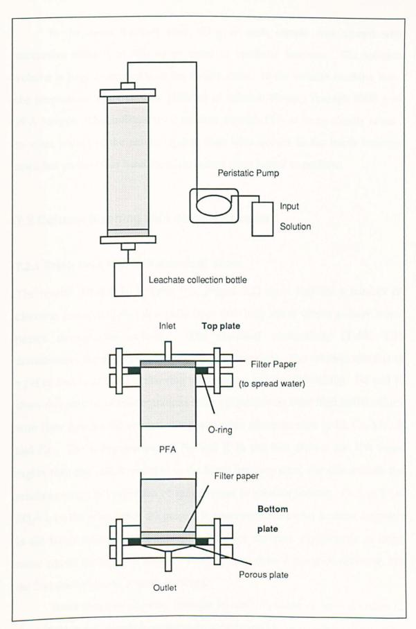
Figure 7.1 Set-up for column leaching tests in down flow configuration
