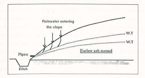
Figure 5.4 Schematic diagram for the infiltration of rainwater on the slope of the ash mound
