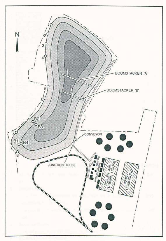
Figure 2.1 Drax Power station and the Barlow PFA disposal site (The numbers 1-8 denote locations of outlet pipes for leachate water samples and the B1-B4 represent the locations of PFA boreholes. Not in scale)
