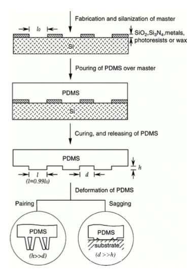
Figure 1.19. Schematic illustration of the procedure for casting PDMS replicas from a master having relief structures on its surface (Xia & Whitesides 1998).
