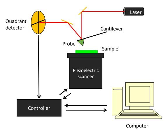
Figure 1.31. Schematic for AFM. (From MacGregor-Chatwin, 2014)
