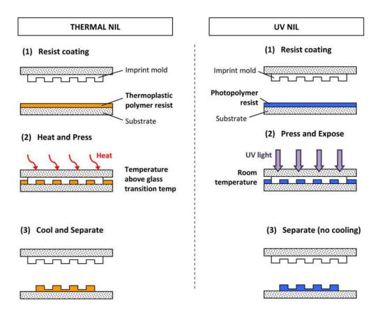
Figure 1.22. Schematic of thermal NIL and UV NIL processes (Kooy et al 2014)
