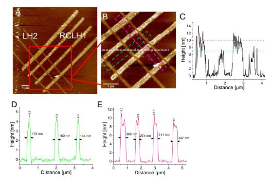
Figure 4.17. AFM images of the intersecting RCLH1 and LH2 nanolines created by successive local oxidations on a silicon surface.
