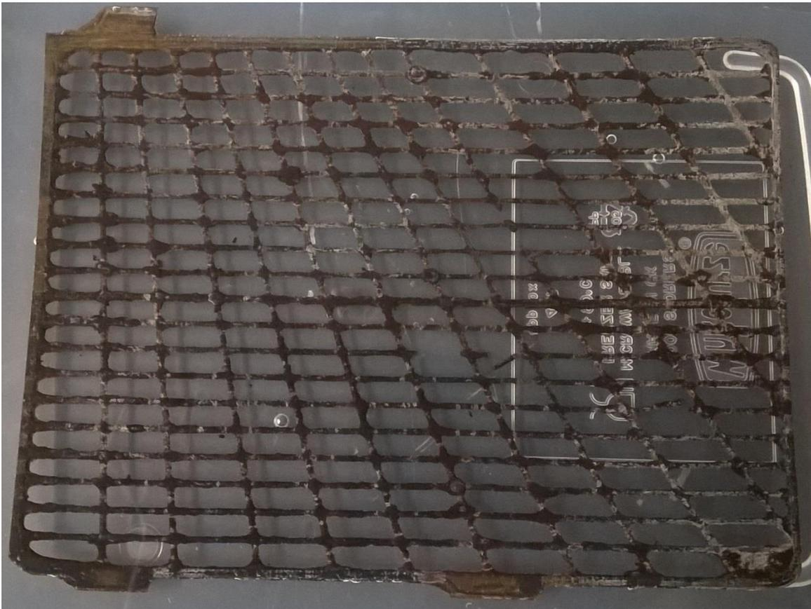
Figure 6.2 – Unpasted plate grid.
