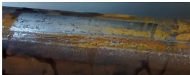
**Figure 6.9:** railhead wear track after 24 pendulum swings
