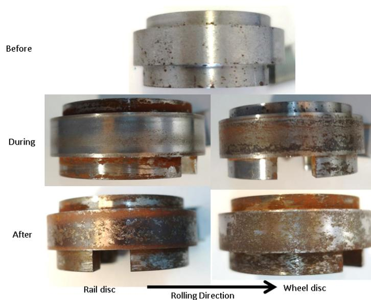
**Figure 7.8:** SUROS wheel and rail discs before, during and after testing
