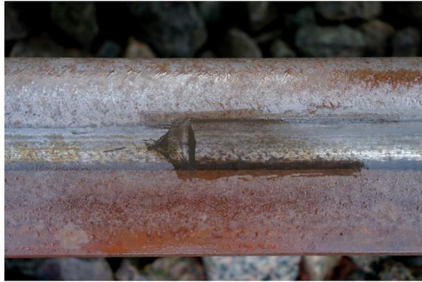
**Figure 4.18:** A paste formed on top of the railhead after artificial wetting
