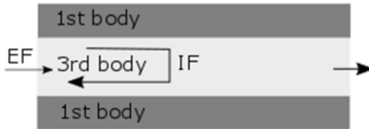
**Figure 2.10:** The third body flow, external flow (EF) and internal flow (IF)
