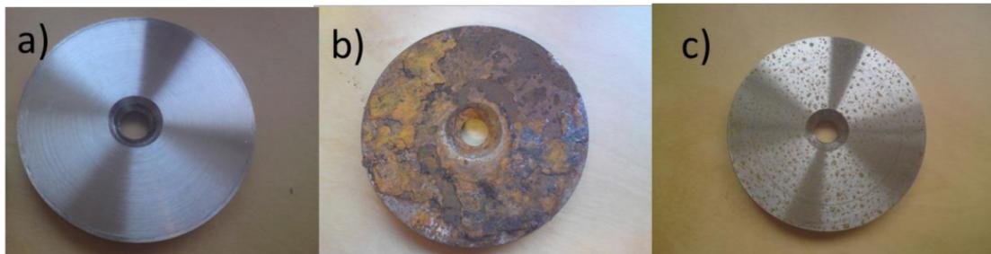
**Figure 2.12:** Oxidised rail discs; G0 (left), G1 (middle), G2 (right) [26]
