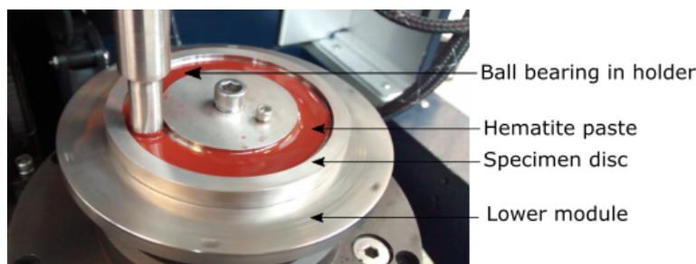
**Figure 6.17:** A “grooved” disc filled with hematite paste
