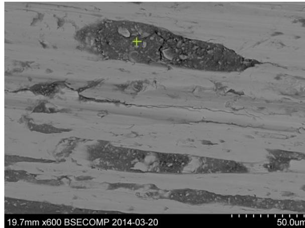
**Figure 2.20:** Backscattered electron SEM images of an oxide flake which shows atomic density. The oxide flake contains a higher percentage of oxygen which has a lower atomic number than iron, therefore showing up as a darker region on the image
