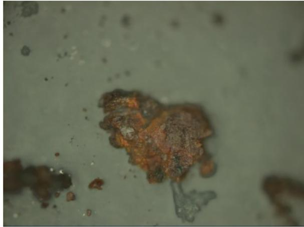
**Figure 2.22:** Optical microscopy of wear debris that appears to be the red oxide, hematite
