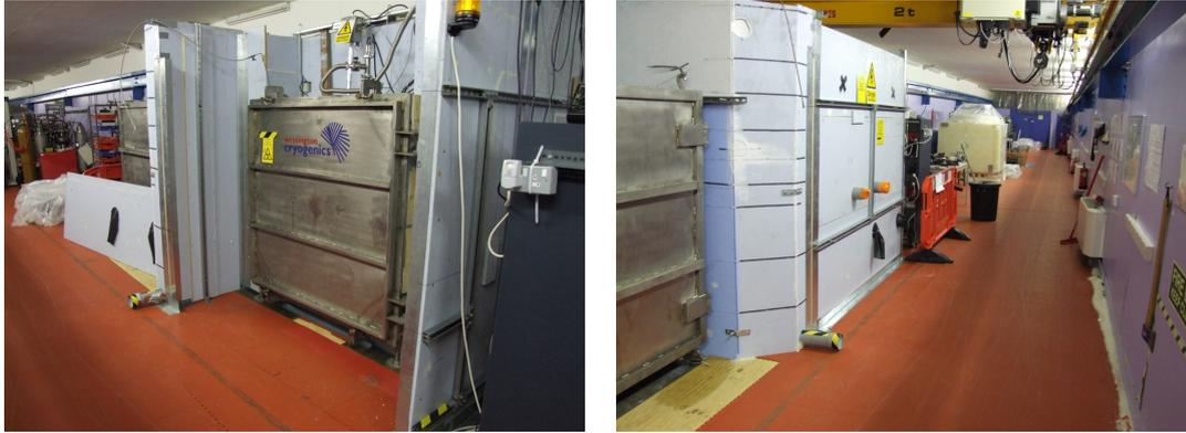
(a) With the front neutron shielding removed for access. (b) With the front neutron shielding constructed. Orange ports in the front are areas for insertion of neutron source.
