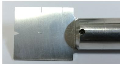
**Figure 3.6:** Photograph of the TRED apparatus beam mask. The mask contains two orifices, 200  $\mu\text{m}$  and 500  $\mu\text{m}$  in diameter.
