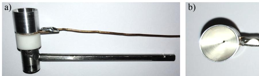
**Figure C.10:** Photograph of the TRED apparatus Faraday cup and beam stop assembly viewed from a) the side, and b) the top.
