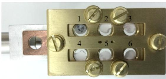
**Figure 3.24:** Photograph of the TRED apparatus sample holder, showing the polycrystalline platinum internal standard at position 1. The diffraction signal from the internal standard is routinely used to optimise the solenoid lens focusing.
