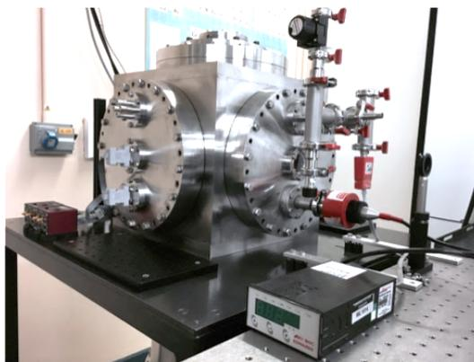
**Figure 8.6:** Photograph of the York ultrafast point-projection microscopy apparatus.
