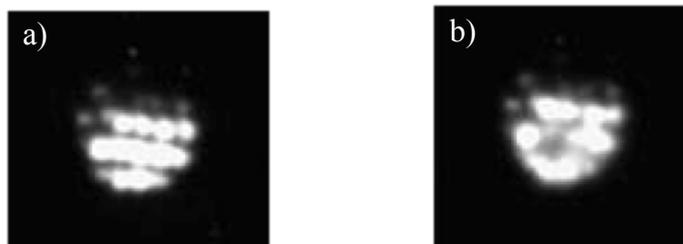
**Figure 3.22:** Image frame recorded during PIL time-zero determination experiments with a) poor, and b) optimum temporal overlap.
