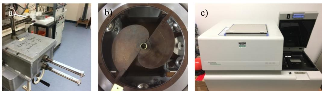
**Figure B.5:** Photographs of the York GED apparatus: a) the plate box, b) the rotating sector, and c) the flat-bed scanner. In the centre of the rotating sector, a beam stop collects unscattered electron, preventing detector damage. The edges of the beam-stop are coated with a thin layer of ZnS-based scintillator to facilitate the visual alignment of the electron beam.
