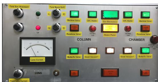
**Figure B.6:** Photograph of the York GED apparatus control panel.
