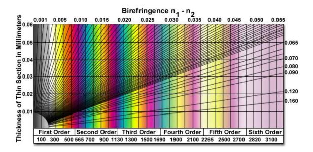
Figure 2.7. The interference colour chart. The interference colour can be correlated with the actual retardation (bottom horizontal axis), thickness (left hand vertical axis), and birefringence (top and right hand axes) of the sample. If two of the three variables are known, the remaining one can be determined by drawing a line from the lower left hand corner to the upper and right hand boundaries [138].
