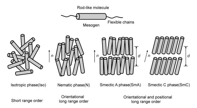
Figure 1.2. Schematic drawing of rod-like molecule and the organization of molecules in different liquid crystal phases. For clarity the alkyl chains are not shown in the models [11].
