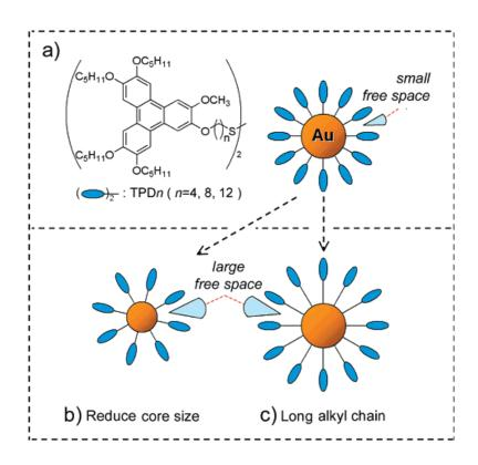
Figure 1.14. Three strategies to construct 1D arrangement of gold nanoparticles: (a) Synthesize molecules with triphenylene ligands (TPDn, n = 4, 8 or 12) and gold nanoparticles stabilized by TPDn; enlarge free space between triphenylene moieties: (b) reduce the core size; (c) or use long alkyl chain.
