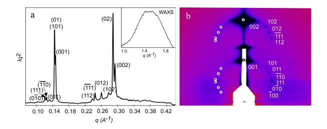
Figure 3.7. X-ray diffraction pattern of the triclinic phase of sample  $T-C_1(OC_{11}F_8)$  a) The 1D SAXS spectrum, converted from 2D powder SAXS pattern. The inset is the wide angle X-ray scattering feature. b) GISAXS pattern from an oriented thin film prepared on silicon substrate.
