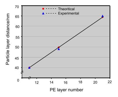
Figure 5.6. Relationship between the distance of the two gold nanoparticle layers and the number of polyelectrolyte layers used in between. Only sample with 11, 15 and 21 polyelectrolyte layers are described here.
