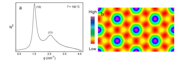
Figure 4.7. a) Powder Diffraction pattern of sample AuL3C12, and b) the reconstructed electron density map of the 2D hexagonal structure.
