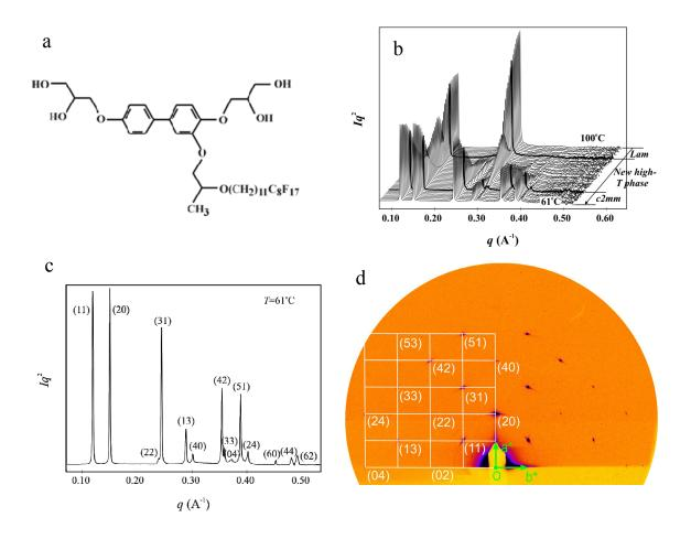
Figure 3.2. a) Molecular structure of compound T-C<sub>1</sub>(OC<sub>11</sub>F<sub>8</sub>). b) Powder diffractograms recorded by SAXS at continuous cooling run with cooling rate of 2 °C/min. c) SAXS pattern and d) GISAXS pattern of the 2D Col<sub>rec</sub>/c2mm phase recorded at 61 °C.
