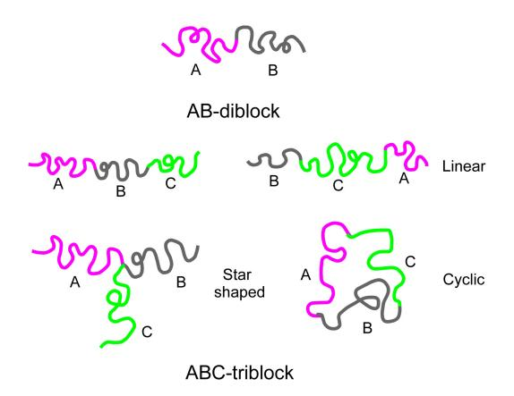
Figure 1.5. Comparison of diblock-copolymers and different types of triblock copolymers; only two of the three possible sequences for linear triblock copolymers are shown [33-35].
