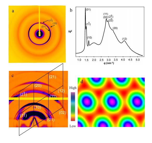
Figure 4.10. a) Small angle X-ray scattering pattern of sample AuCholC6 taken at 30 °C. b) 1D spectrum converted from a). c) GISAXS pattern from an oriented thin film. d) Reconstructed electron density map from experimental results using the first three low order reflections.
