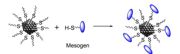
Figure 1.9. Schematic representation of the synthesis process of mesogen covered gold nanoparticles. The monolayer protected gold nanoparticle is functionalized *via* an exchange reaction [94].
