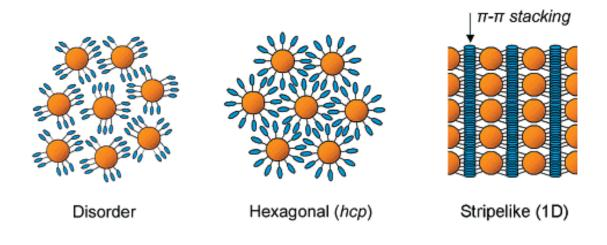
Figure 1.15. The possible arrangement of triphenylene functionalized gold nanoparticles depends on factors of  $\pi$ - $\pi$  interaction, space around triphenylenes on Au, and solvent polarity (ratio of methanol/toluene) [104].
