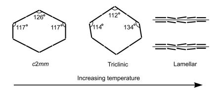
Figure 3.19. The change of cylinder cross section with the increasing of temperature.
