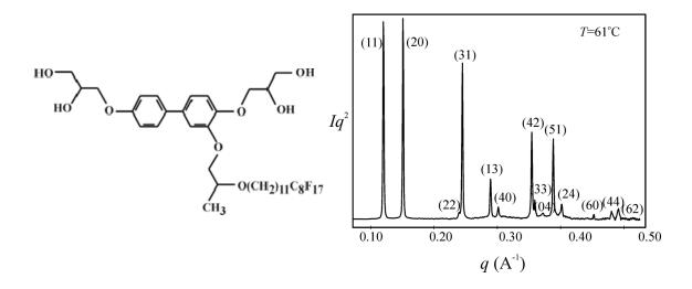
Figure A4. The molecular structure of compound  $T-C_1(OC_{11}F_8)$  and the small angle X-ray scattering pattern of the *c2mm* phase recorded at 61 °C.
