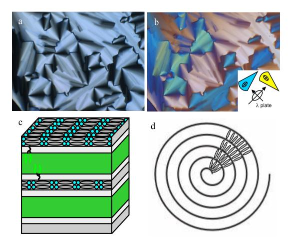
Figure 3.15. a) Texture of the lamellar smectic phase of sample  $T-C_3(C_{11}F_8)$  under crossed polarizers recorded at 140 °C. b) The same phase recorded at the same temperature with  $\lambda$ -plate retarder. The indicatrix orientation in the  $\lambda$ -plate and in the two types of fans is shown in the inset. c) The schematic drawing of lamellar smectic phase. d) The orientation of molecules in the smectic layer.
