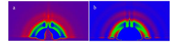
Figure 5.9. a) Experimental GISAXS pattern of sample with 21 polyelectrolyte layers. b) Simulated GISAXS pattern using IsGISAXS software.
