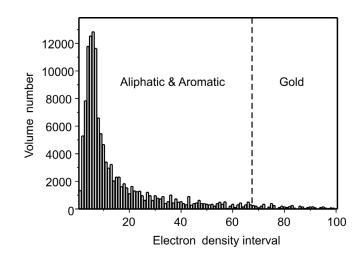
Figure 4.9. Volume number *vs.* electron density histogram of the face centre cubic phase. The dashed line indicates the boundary between high electron density gold core and low electron density organic components.
