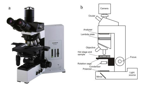
Figure 2.6. a) The polarized optical microscope used in this thesis (Olympus BX-50), and b) its schematic diagram [136].
