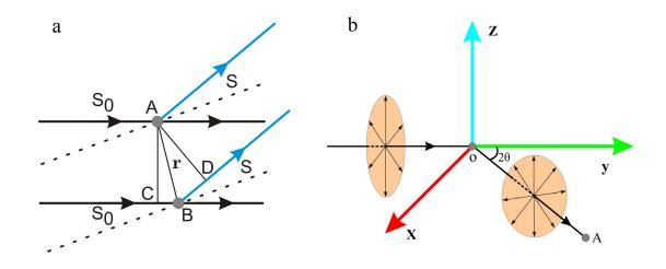
Figure 2.2. a) The incident beam  $S_{\theta}$  strikes on two scatterers separated by distance r, generating scattering beam S. The phase difference between two diffraction points can be expressed by  $r \cdot (S - S_0)$ . b) An electron located at origin O and the incident beam is along y axis. The scattered intensity at point A not only depends on the distance between it and the electron but also the scattering angle  $2\theta$ .
