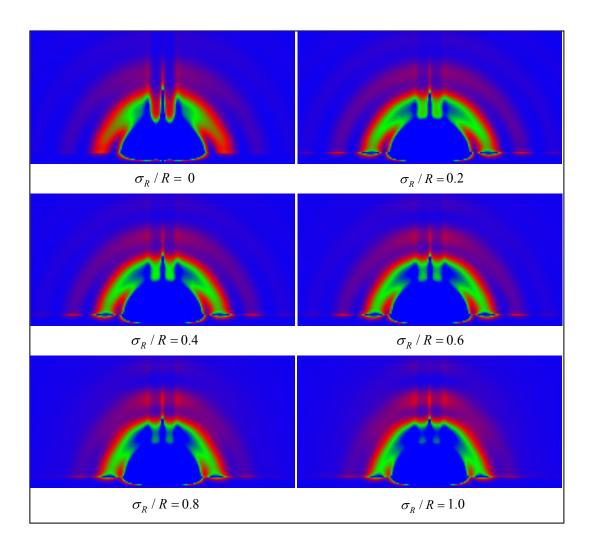
Figure 5.10. The effect of  $\sigma_R / R$  value on the simulated diffraction pattern.
