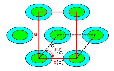
Figure 3.9. Schematic drawing of the relations between the rectangular columnar phase and the triclinic phase of sample  $T-C_1(OC_{11}F_8)$ .
