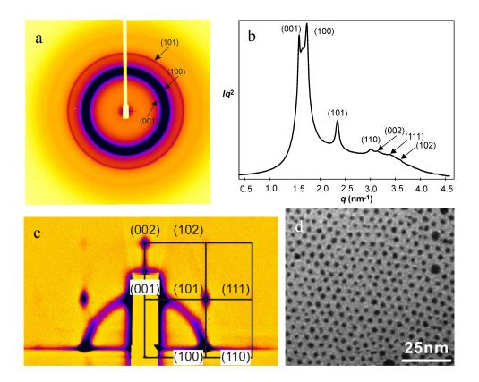
Figure 4.2. a) 2D powder SAXS pattern of sample AuL3 taken at 30 °C b) 1D spectrum converted from a). c) GISAXS pattern from an oriented thin film sample prepared on silicon substrate. d) TEM of a ca. 50 nm thick film in the *P6/mmm* phase of AuL3, viewed along [001] axis (Contributed by R. Zhang).
