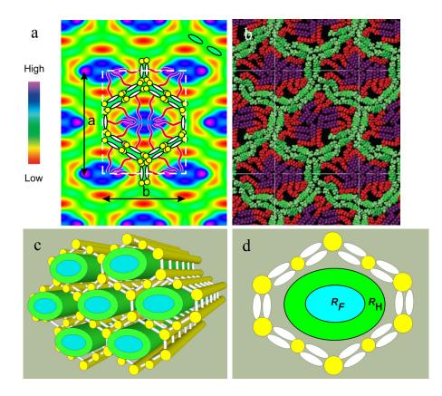
Figure 3.3. a) Reconstructed electron density map of the  $\text{Col}_{\text{rec}}/c2mm$  phase found in sample T-C<sub>1</sub>(OC<sub>11</sub>F<sub>8</sub>). The colour scale is shown on the left. b) Snapshot of molecular simulation. The blue/purple = perfluorinated end groups  $R_F$ , red = aliphatic chains  $R_H$ , green = biphenyl and diol groups. c) and d) sketch of the molecules organization in this mesophase.
