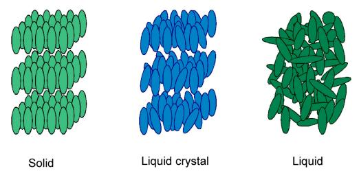
Figure 1.1. Schematic diagrams of solid, liquid crystal and liquid phases. For a typical liquid crystalline material, with increasing temperature the phase transition from solid to liquid occurs through an intermediate liquid crystalline phase (a smectic phase is shown as an example) [4].
