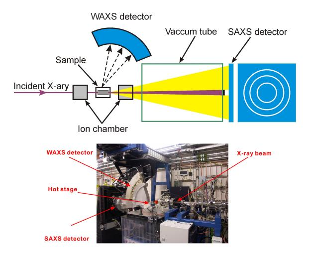
Figure 2.3. Schematically drawing and the real experimental set-up of Small Angle X-ray Scattering at station I22, Diamond, which is also equipped with a WAXS detector.
