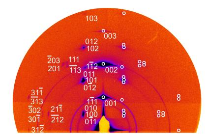
Figure 3.10. Grazing incidence small angle X-ray scattering pattern of the triclinic phase of sample T- $C_3(C_{11}F_8)$  recorded at 75 °C. The white circles indicate the simulated diffraction positions of all the observed reflections in the 2D pattern.
