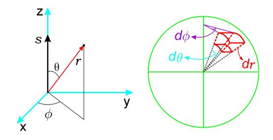
Figure A1. The polar coordinate system and the volume element of sphere
