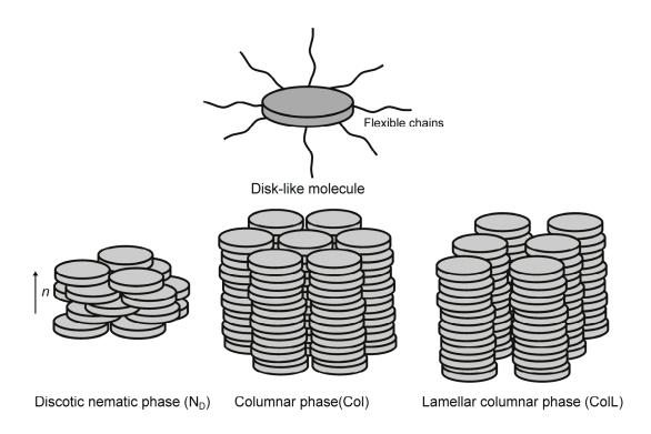
Figure 1.3. The schematic drawing of disk-like molecule and the organizations of molecules in some typical mesophases [4].
