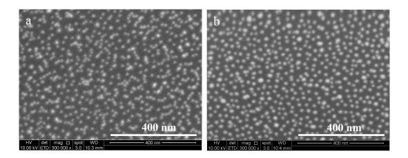
Figure 5.8. The SEM pictures of the double layered gold nanoparticle samples (Contributed by Dr F. Liu). a) Sample with 5 polyelectrolyte layers and b) sample with 15 polyelectrolyte layers in between. Although in both cases the local hexagonal shape formed by the gold nanoparticles is shown, it is more obvious for the sample with more polyelectrolyte layers.
