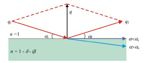
Figure 2.4. The grazing incidence X-ray scattering geometry [130].
