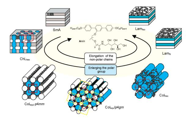
Figure 1.8. Schematic view of the phase sequence of the facial amphiphiles with lateral polyhydroxy groups as a function of the size of polar lateral and lipophilic terminal groups [56].
