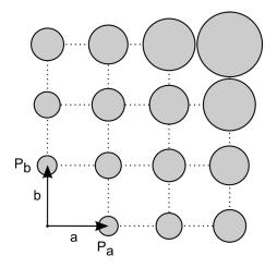
Figure 5.11. Schematic view of a paracrystal in two dimensions. Each circle represents the area where the probability of finding one particle is maximum [172].
