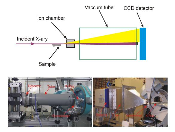
Figure 2.5. Sketch map (top) and the real experimental set-up for grazing incidence small angle X-ray scattering experiments at the XMaS, ESRF (bottom left) and I16, Diamond (bottom right).
