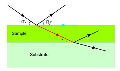
Figure 5.2. The schematic drawing of the path of X-ray beam goes through thin film sample on substrate.
