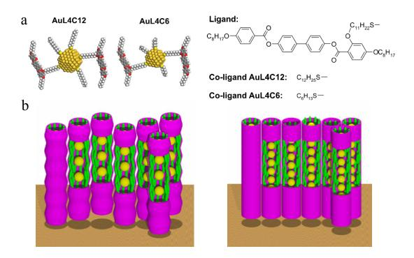
Figure 1.10. a) Models of functionalized gold nanoparticles and the chemical structure of mesogenic ligand and co-ligands. b) Structure models of the gold nanoparticle strings. Left: AuL4C12 which has long co-ligands. Right: AuL4C6 which has shorter co-ligands. The yellow balls and the green color represent gold string and mesogens respectively.
