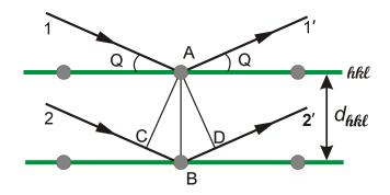
Figure 2.1. The incident X-ray beam scattered by a set of parallel lattice planes.
