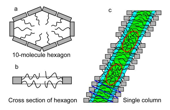
Figure 3.6. a) The 10-molecule composed hexagon in the monoclinic structure. b) The cross section of a single hexagon, which shows the sideway expanded lateral chains. c) Sketch of molecule arrangement during the formation of a single column.
