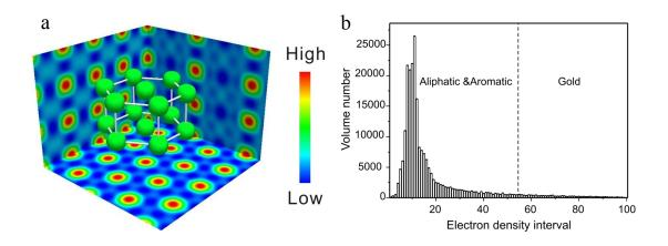
Figure 4.3. a) Reconstructed electron density maps of the *P6/mmm* phase in AuL3. b) The corresponding histogram of the electron density map. In this histogram the calculated electron density is divided into 100 segments between minimum and maximum values. The number of volume elements within each intensity interval is calculated as explained in chapter 2.
