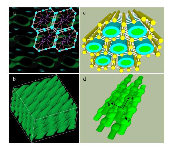
Figure 3.13. Reconstructed electron density map and proposed structure model of the triclinic phase of sample  $T-C_4F_{10}$ . a) The column cross sections and the molecule arrangement on the circumference of each cross section. b) The unevenly distribute electron density along column direction. c) and d) the corresponding model of the reconstructed electron density maps. The colour code used in these models is the same as in Figure 3.3.
