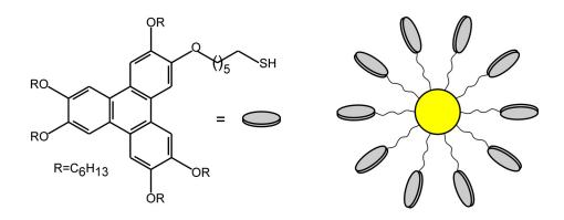
Figure 1.13. Chemical structures of a discotic molecule 6-{[3, 6, 7, 10, 11-pentakis (hexyloxy)-2-triphenylenyl] oxy}-1-hexanethiol and a schematic drawing of how they are attached to a gold nanoparticle.
