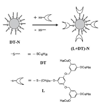
Figure 1.17. Schematic representation of exchange reaction yielding gold nanoparticles (N) covered with surface-protecting groups (dodecanethiol, DT) and dedrimers (L).
