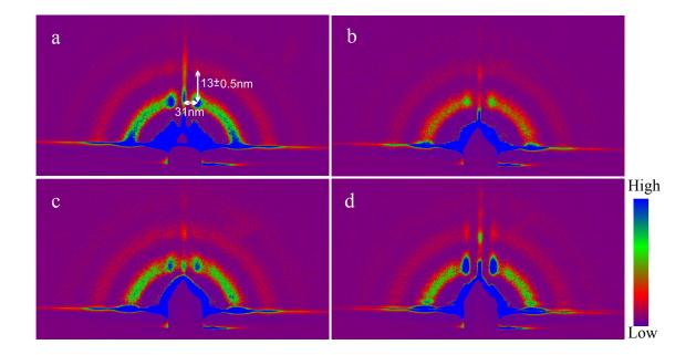
Figure 5.3. The GISAXS patterns of the samples with (a) 5, (b) 11, (c) 15 and (d) 21 polymer layers in between the two nanoparticle layers.
