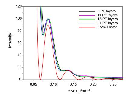
Figure 5.4. The one dimensional spectrum of the grazing incidence small angle X-ray scattering patterns, which are converted from GISAXS patterns corresponding to Figure 5.3. The theoretical calculation of a sphere form factor with the diameter of 6.5 nm is shown as red curve.
