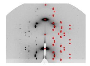
Figure A3. The simulated GISAXS diffraction pattern of the triclinic structure found in the sample T-C<sub>4</sub>F<sub>10</sub>
