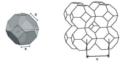
Figure 1.18. Left: The truncated octahedron with the polyhedron edge length of *e*. Rights: Body-centered cubic lattice of  $Im \bar{3}m$  symmetry composed of truncated octahedrons. The cubic lattice parameter is *a*.
