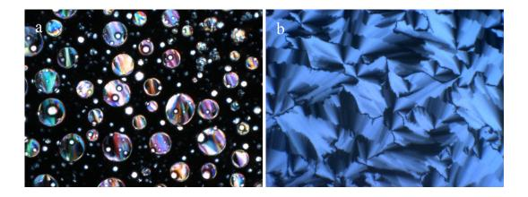
Figure 3.17. Texture of the lamellar phase of sample  $T-C_4F_{10}$  under crossed polarizers. a) Texture of lamellar isotropic phase recorded at 175 °C. b) Texture of lamellar smectic phase recorded at 130 °C.
