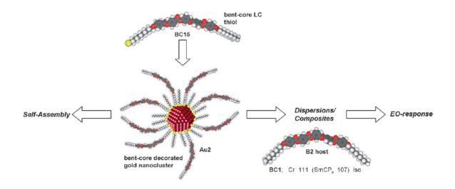
Figure 1.16. Schematic representation of the use of thiol-terminated bent-core compounds in the formation of bent-core functionalized gold nanoparticles, and the potential of using such nanoparticles in dispersions with bent-core LC hosts to alter the bent-core LC host's thermal properties and/or electro-optic response [111].
