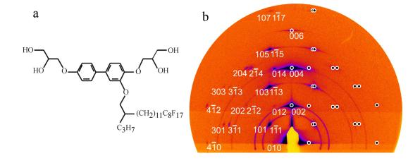
Figure 3.4. a) Molecular structure of compound  $T-C_3(C_{11}F_8)$ . b) Grazing incidence small angle X-ray scattering pattern recorded at 70 °C. The white circles show the simulated diffraction positions of the observed reflections on the 2D pattern.
