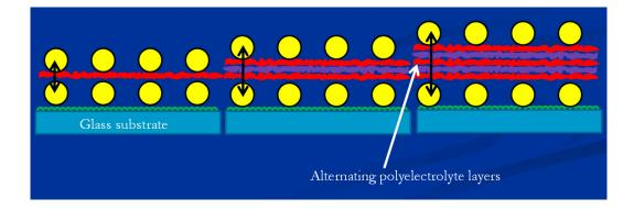
Figure 5.1. Simple schematic drawing of models of layered samples with different number of polyelectrolyte layers between two gold nanoparticle layers [166].
