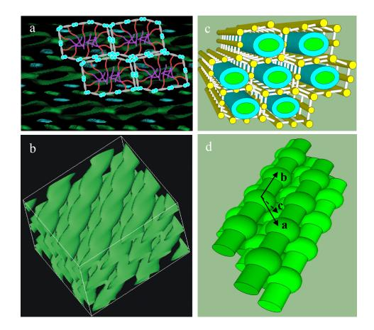
Figure 3.11. Reconstructed electron density map and proposed structure model of the triclinic phase of sample T-C<sub>3</sub>(C<sub>11</sub>F<sub>8</sub>). a) The column cross sections and the molecule arrangement on the circumference of each cross section. b) The unevenly distribute electron density along column direction. c) and d) the corresponding model of the reconstructed electron density maps. The colour code is the same as Figure 3.3.
