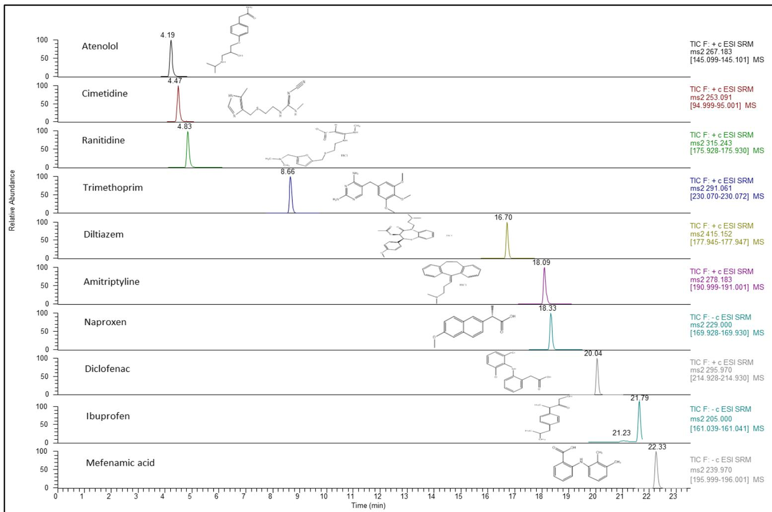
Figure 7.2 SRM chromatograms of targeted pharmaceuticals from an extract of sediment spiked at 20 ng g<sup>-1</sup>
