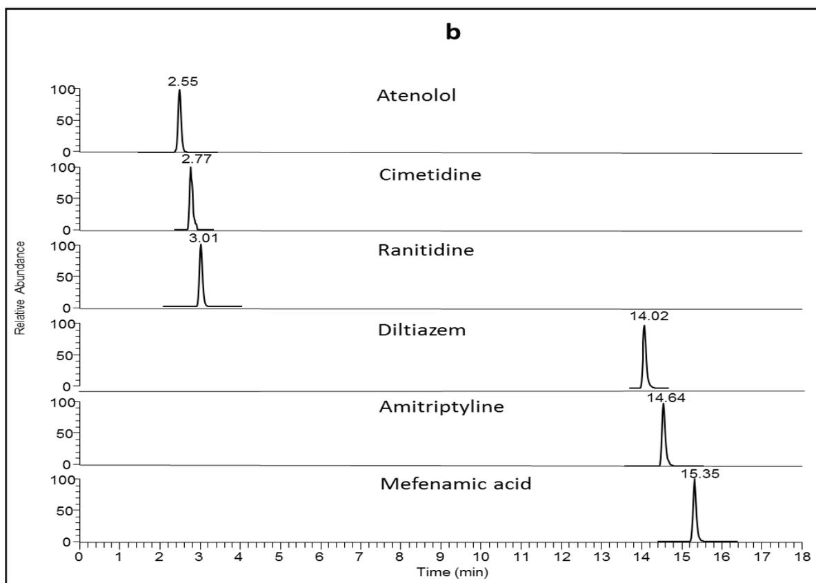
**Figure 4.1** Chromatogram of a mixture of the pharmaceuticals in methanol. Chromatographic conditions: Zorbax Eclipse XDB-C18 reverse-phase column (250 mm × 4 mm i.d., 5 μm); Mobile phase of 10mM ammonium acetate with acetic acid and ACN at pH= 4.8; flow rate 1.0 mL
