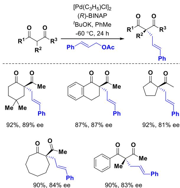
Scheme 2 – Scope of 1,3-diketone substrate in enantioselective allylation reaction.<sup>9</sup>
