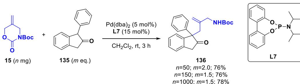
Scheme 68 – Pd-catalysed allylation of **135** with **15** proceeds well on small- and large-scale.
