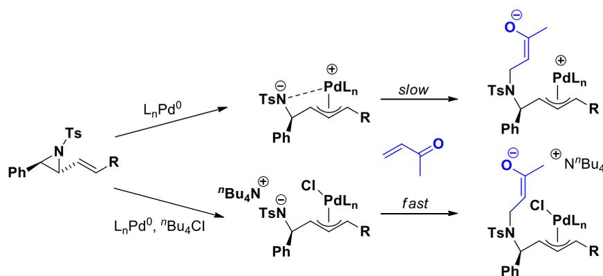
Scheme 19 – Enhanced reactivity with addition of tetra-*n*-butylammonium chloride.
