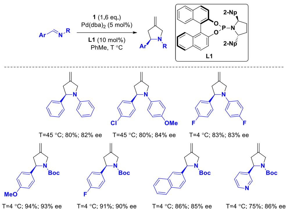
Scheme 10 – Application of **L1** allows the enantioselective synthesis of a variety of pyrrolidine products.
