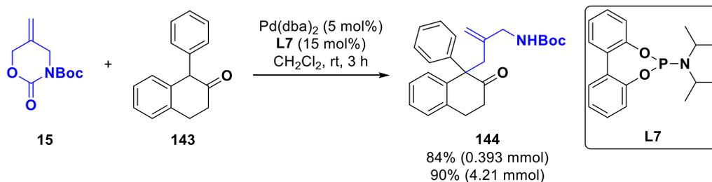
Scheme 72 – Performance of tetralone **143** in the Pd-catalysed allylation reaction.
