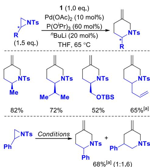
Scheme 13 – Reaction of Pd-TMM with a variety of 2-substituted aziridines. [a] Performed with racemic aziridine
