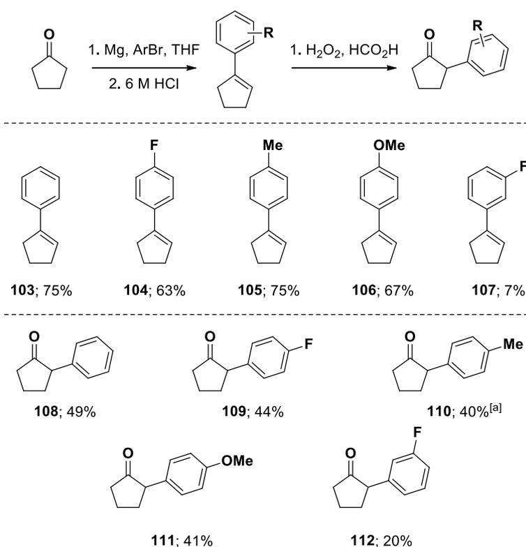
Scheme 59 – Synthesis of a range of 2-arylcyclopentanones. [a] Performed with 2.0 eq. of mCPBA.
