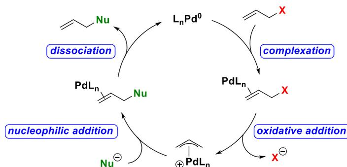
Figure 1 – General catalytic cycle for the Tsuji-Trost reaction.
