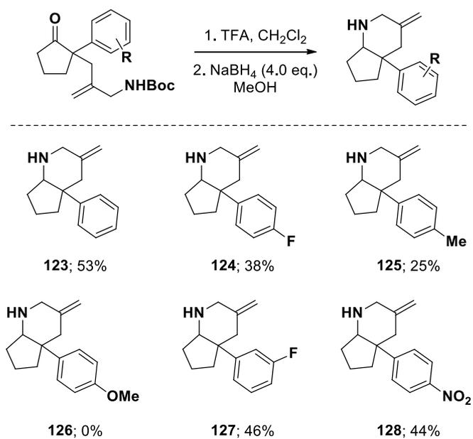
Scheme 65 – Preparation of piperidines **123-128** *via* reductive amination of allylated ketones **115-120**.
