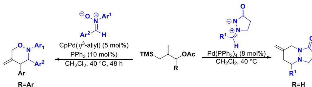
Scheme 12 – [3 + 3] cycloaddition of Pd-TMM with nitrones and azomethine imines.
