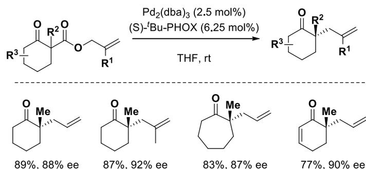
Scheme 5 – Palladium-catalysed allylation from  $\beta$ -ketoesters.<sup>10</sup>
