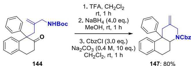
Scheme 74 – 3-step reductive amination-protection sequence for the synthesis of **147**.
