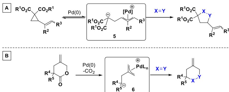
Scheme 15 – (A) Pd-catalysed reaction of vinylcyclopropanes with heterocumulenes *via* **5**. (B) Pd-catalysed reaction of  $\gamma$ -methylidene- $\delta$ -valerolactones with heterocumulenes *via* **6**.
