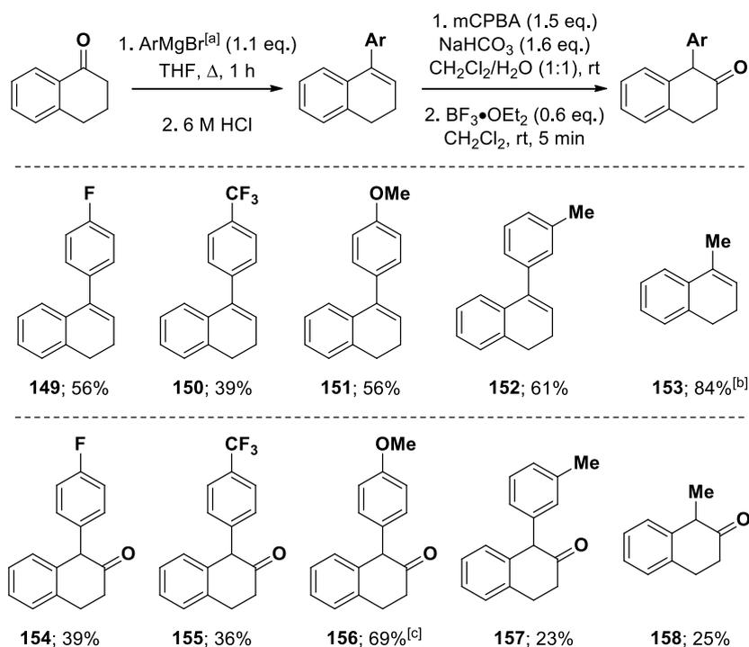
Scheme 76 – Synthesis of a range of 1-substituted-2-tetralones. [a] Grignard reagents prepared by stirring Mg (1.2 eq.) in THF with addition of aryl bromide (1.2 eq.) and  $\text{I}_2$  used as initiator. [b] Grignard prepared using MeI (1.6 eq.), Mg (1.5 eq.) in  $\text{Et}_2\text{O}$ . [c] Prepared using Oxone (8.0 eq.) and  $\text{NaHCO}_3$  (40.0 eq.).
