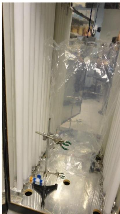
**Figure 65:** Teflon<sup>®</sup> reaction chamber (80 L).
