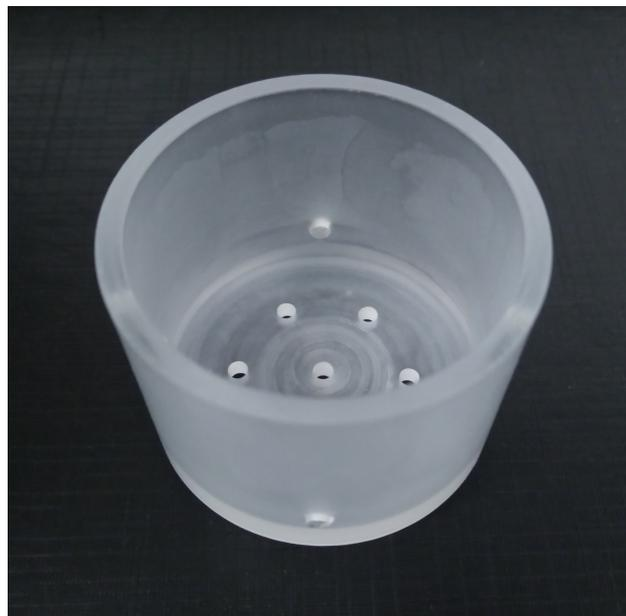
Figure 2.2. Plastic insert used for mechanical stress experiments. These inserts were specially designed for use with cells, with small holes in the base. They were developed to use in conjunction with 6 well plates.
