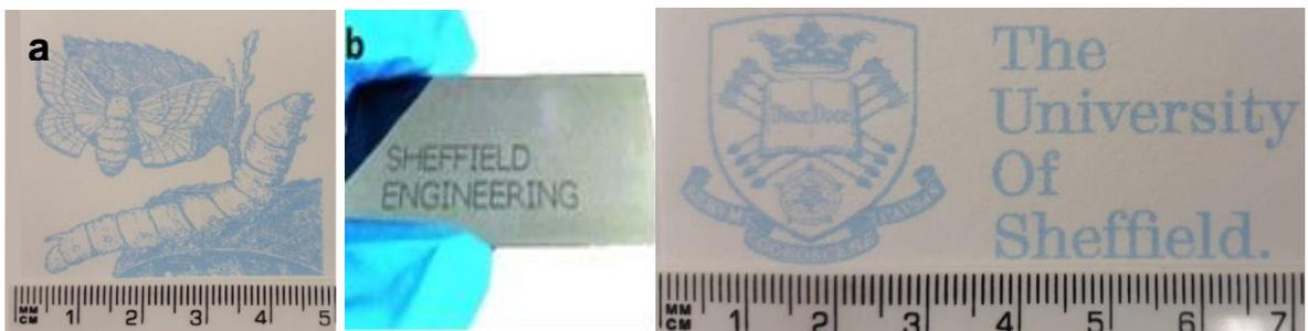
**Figure 3-18** Pattern directly printed using RSF solution, a) and c) complex bitmap images printed on paper with blended RSF inks (Coomassie blue mix with RSF solutions); b) ‘SHEFFIELD ENGINEERING’ letters printed on silicon wafer using 40 mg/ml RSF solution.
