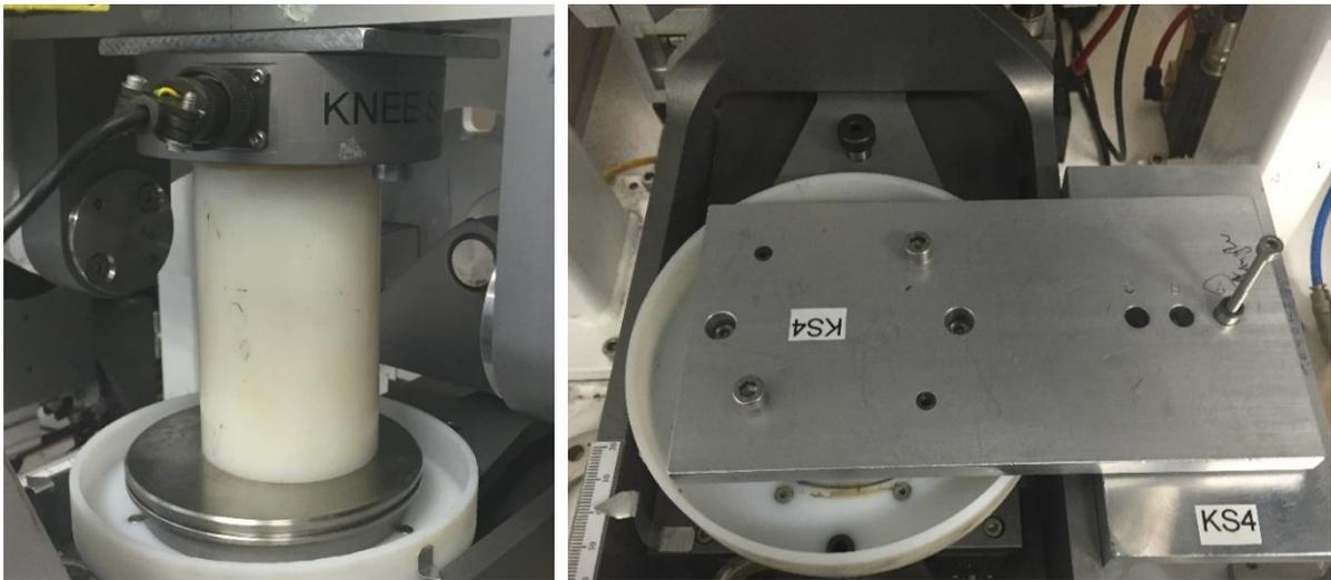
Figure 4.2 KS4 load and rotation/displacement calibration set up
