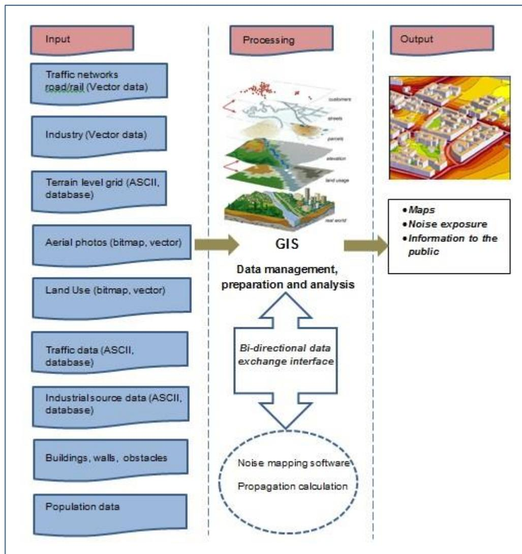
**Fig.2.3.** Overview of the noise mapping process (WG\_AEN, 2003, p53) with emphasis on the bi-directional data exchange during the processing stage.
