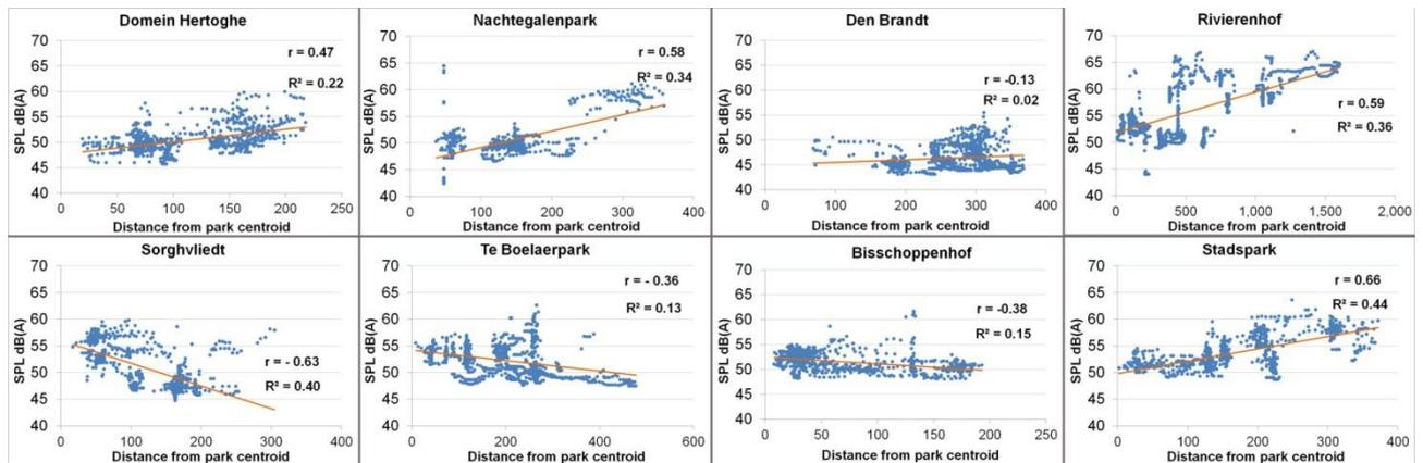
**Fig.6.11.** Relationship between the noise levels of the selected cluster points and the distance from the park centroid (p-value<0.001). The coefficient of determination ( $R^2$ ) and Pearson correlation coefficient ( $r$ ) are reported in each graph.
