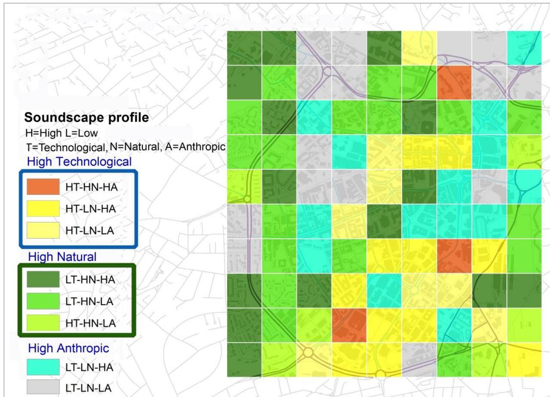
**Fig.8.7.** Representation of the eight “High” (H) and “Low” (L) profiles of the sound sources and arranging them into three larger groups based on the maximum levels per sound source within the study area.
