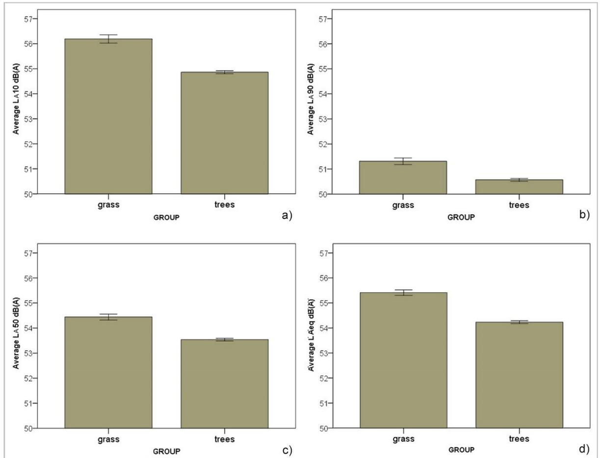
**Fig.6.13.** Average noise levels per index for the measurement points inside the tree and grass areas using error bars (95% confidence interval).
