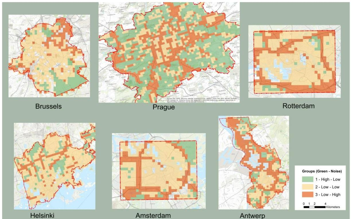
**Fig.4.12.** Spatial distribution of the three clusters representing the relationship between noise and green. Results are based on the k-means algorithm and the grouping analysis tool in ArcGIS. Basemap source: ESRI 2016d.
