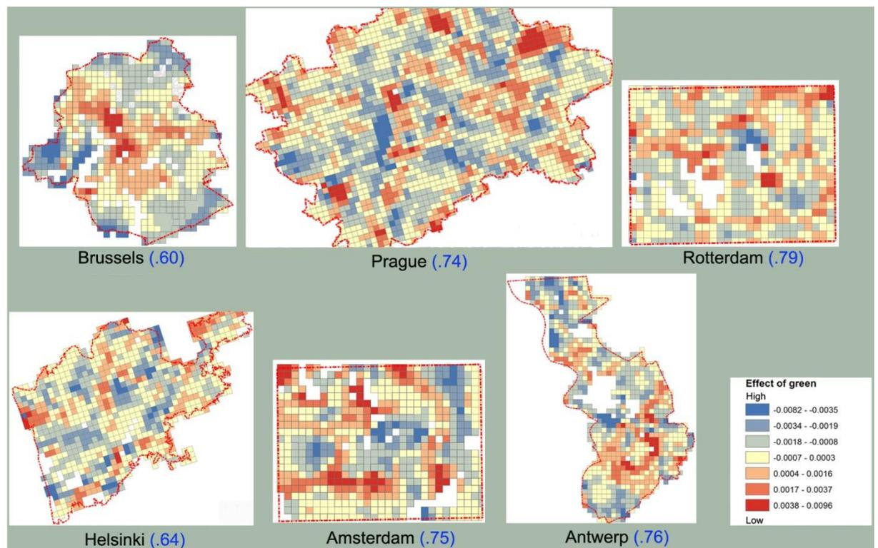
**Fig.4.9.** The effect of green ( $\Delta gsr$ ) on noise according to the results of the GWR model and the associated correlation coefficient ( $R^2$ ) for each city.
