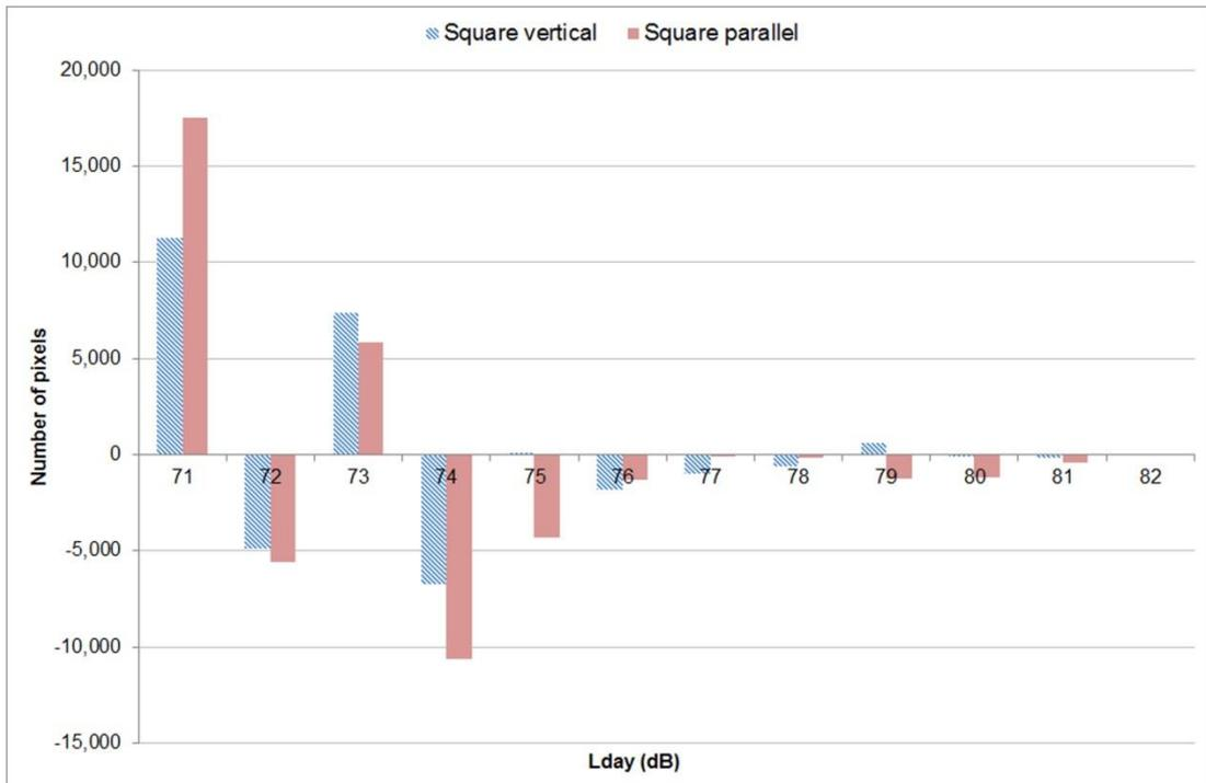
**Fig.3.8.** Comparison between the vertical and parallel to the inner roads green space arrangement for the square configuration as shown in Fig.3.6. The total number of pixels per noise band on the y axis is calculated by subtracting the ones in the rigid condition ( $G=1$ ) from the ones in the porous condition ( $G=0$ ).
