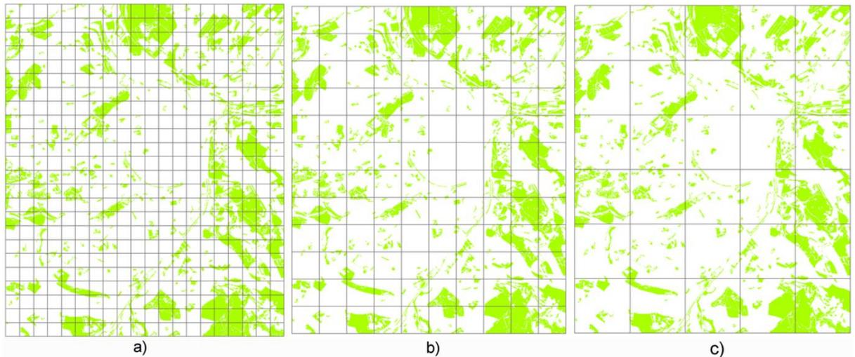
**Fig.5.3.** Possible grid sizes and respective coefficients of determination ( $R^2$ ) between green space ratio and noise levels ( $L_{den}$ ) tested in Sheffield: a) 250x250m -  $R^2=.07$ , b) 500x500m -  $R^2=.037$ , c) 1,000x1,000m -  $R^2=.285$ .
