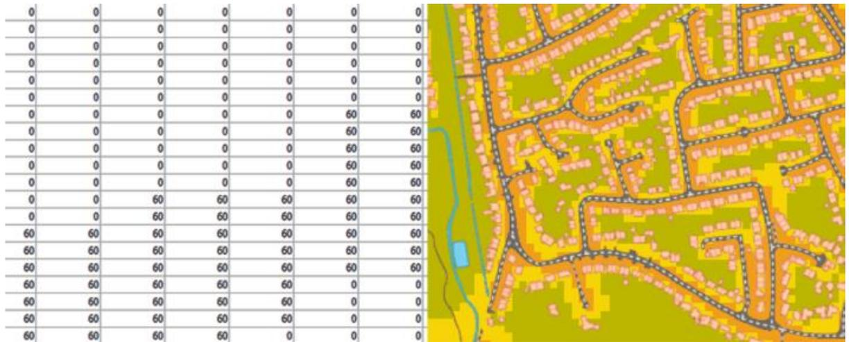
**Fig.5.5.** Matlab code results presenting the transformation from RGB pixel values in dB(A) levels.
