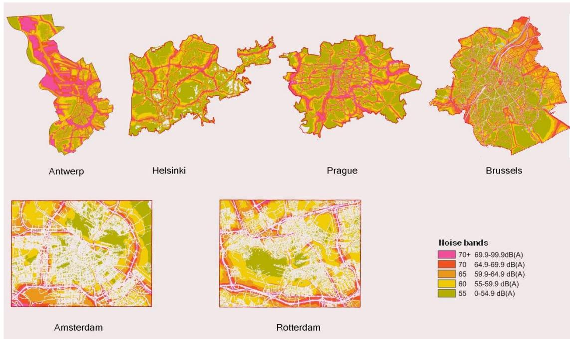
**Fig.4.3.** Representation of the noise maps for the six cities using a common noise band scale.
