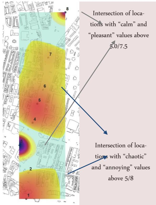
**Fig.8.10.** Spatial queries with combined results contributing to the recognition of “quiet” and “noisy” areas based on perceptual parameters assessed during the soundwalk.
