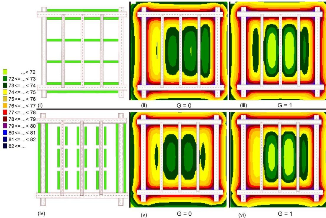
**Fig.3.6.** Noise propagation in a square form tested with different ground factors and green lanes placed in a vertical (ii,iii) and parallel arrangement (v, vi) to the inner roads.
