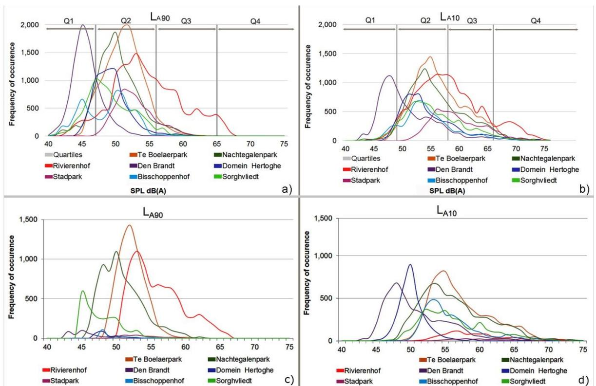
**Fig.6.9.** (a,b) Frequency of occurrence for  $L_{A90}$  and  $L_{A10}$  based on values per measurement point, (c,d) Frequency of occurrence for  $L_{A90}$  and  $L_{A10}$  based on the aggregated values per cell.
