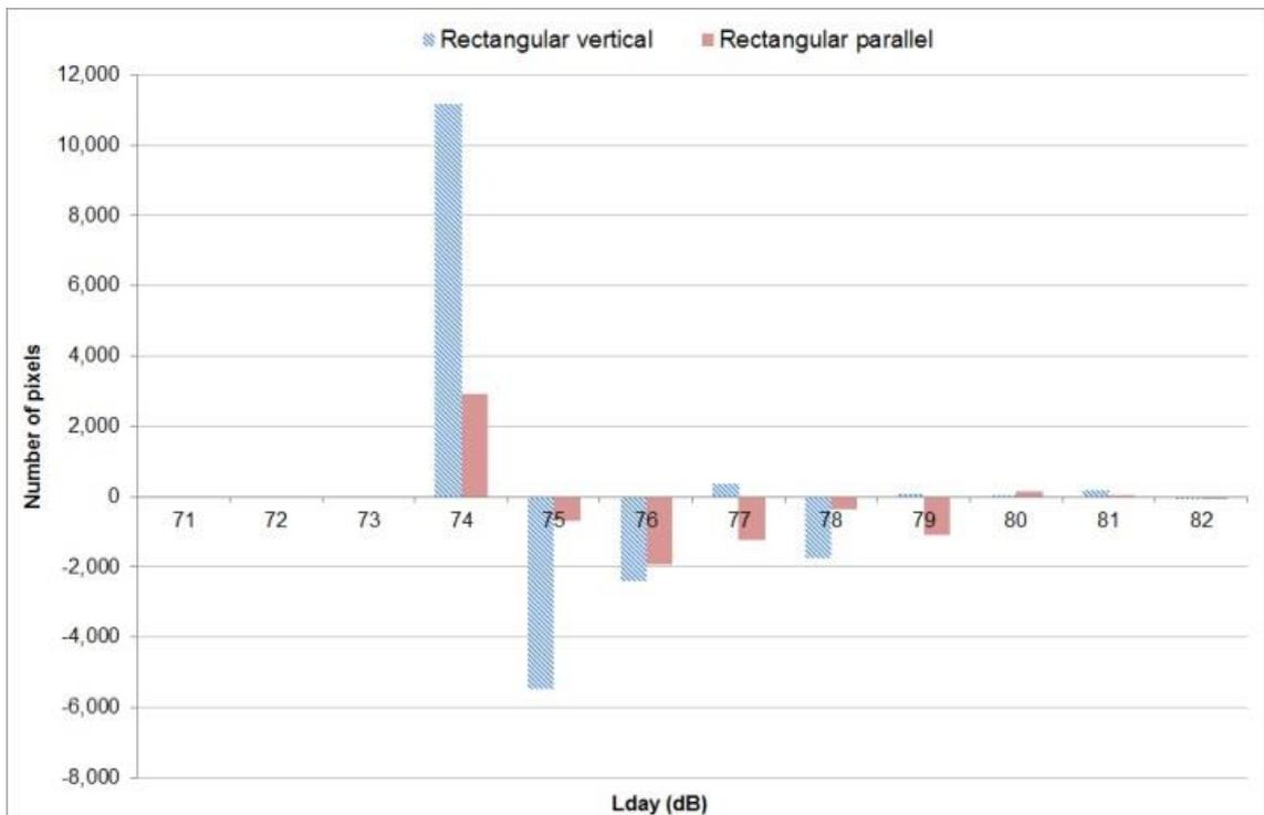
**Fig.3.9.** Comparison between the vertical and parallel to the inner road green space arrangement for the rectangular configuration as shown in Fig.3.7. The total number of pixels per noise band on the y axis is calculated by subtracting the ones in the rigid condition ( $G=1$ ) from the ones in the porous condition ( $G=0$ ).
