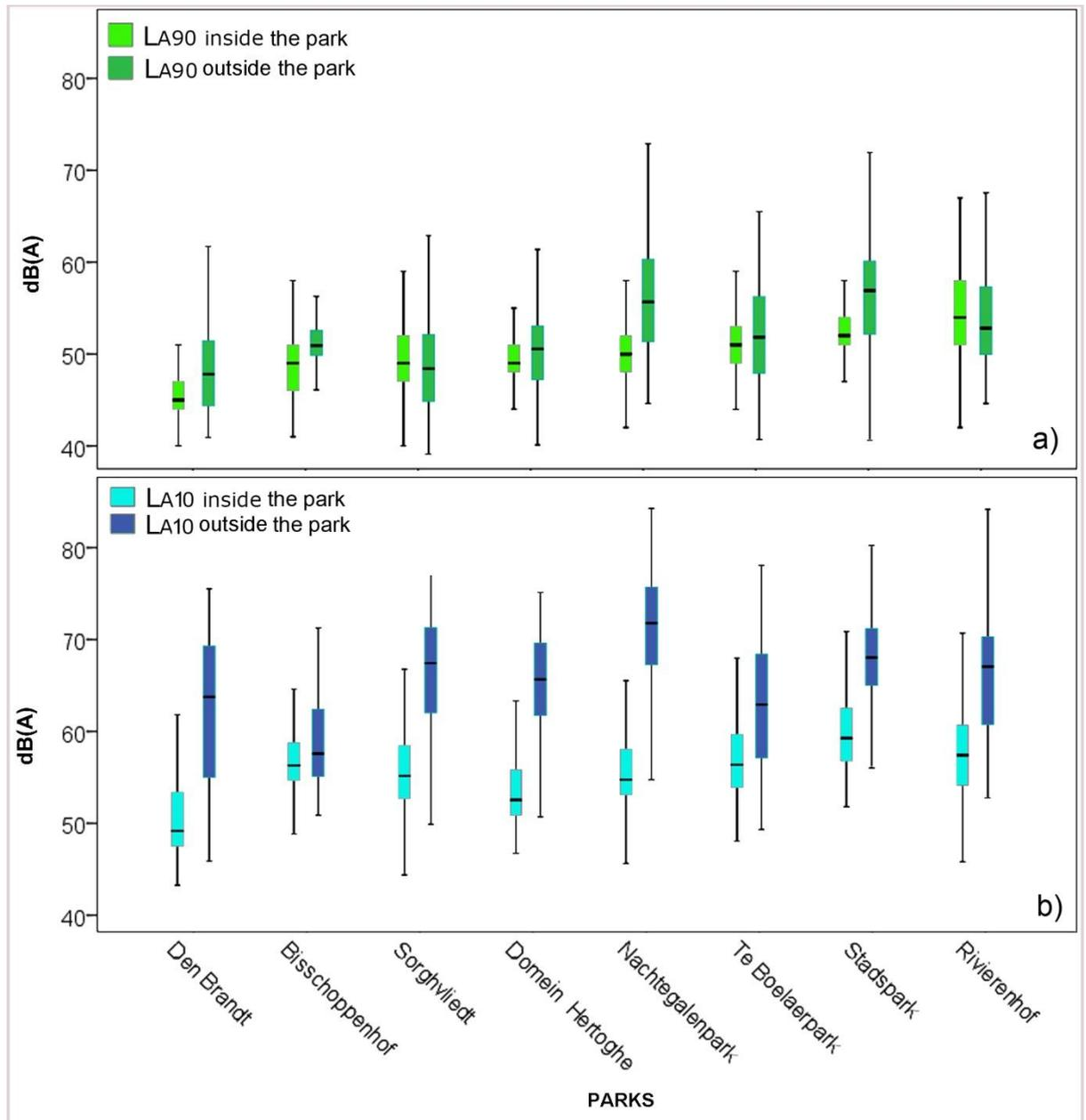
**Fig.6.10.** Box plots for (a)  $L_{A90}$  and (b)  $L_{A10}$  describing the sound environment inside and outside the eight parks. Results have been sorted in an ascending form for  $L_{A90}$  (inside).
