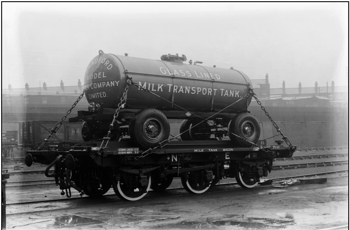
**Bradford Model Milk Company Limited 2,000-gallon demountable milk tank and flat-wagon, illustrating the arrangement pioneered by the Southern Railway and the London Co-operative Wholesale Society at the latter's Bruton dairy in 1931. Although undated, the wagon was probably constructed by the LNER c1934. Source: National Railway Museum DS130202-101926.**
