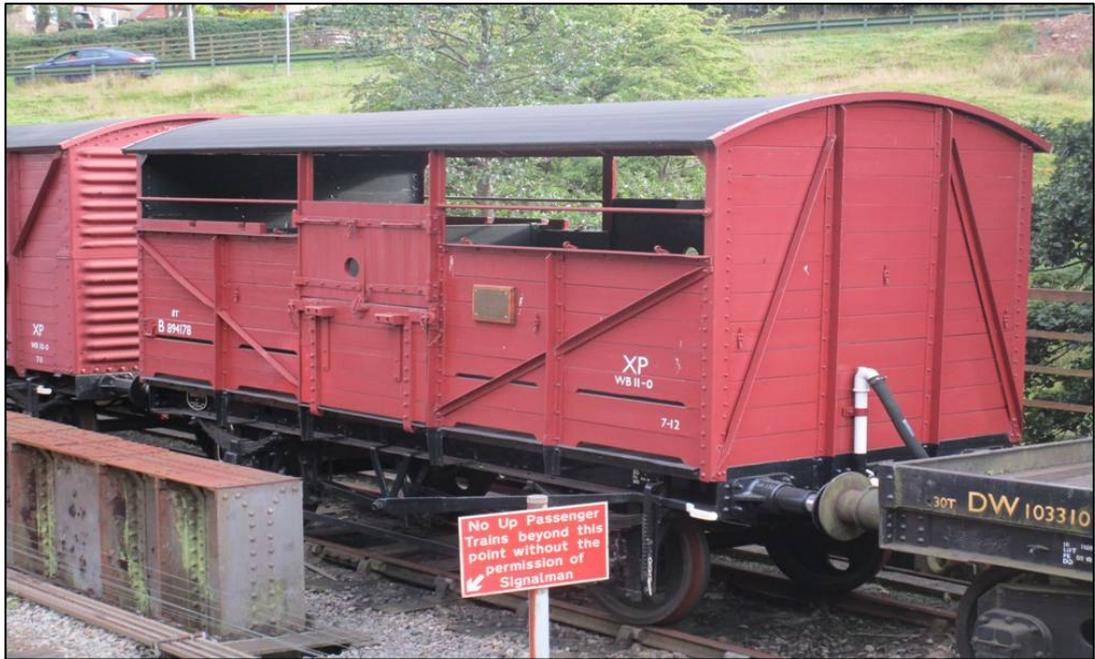
**The basic features of the British Railways 8-ton cattle wagon, such as this example at the North Yorkshire Moors Railway had changed little from the standard Railway Clearing House design. Each wagon could be split into compartments with dividers. Note the apertures for draining effluent and the outside structural members on the wagon ends, so-designed to prevent injury to animals. Author’s collection.**
