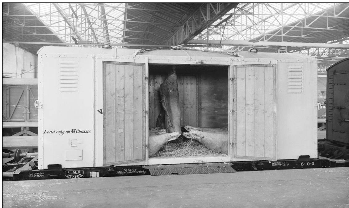
**Beef loaded in an LMS "M-type" ventilated container, 1936. The carcasses are protected by cloth sacking; also note the arrangement of carcasses on the floor, a practice which allowed full utilisation of wagon capacity, yet shows little consideration for hygiene beyond straw bedding. Source: National Railway Museum 1997-7409\_LMS\_7990.**
