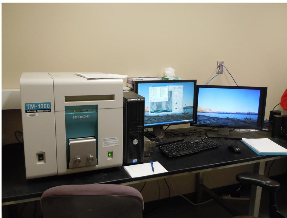
Figure 4.5. Variable-pressure Hitachi TM-1000 SEM equipped with an EDX detector (LACORE, University of Minnesota).
