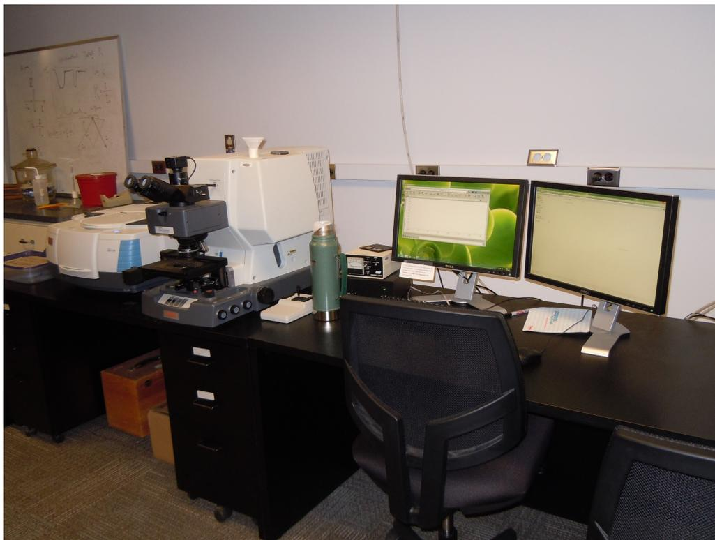
Figure 4.7. FTIRM. Nicolet Continuum microscope connected to a Nicolet Series II Magna-IR System 750 FTIR bench (Characterization Facility, University of Minnesota). The dewar flask contains liquid nitrogen for cooling the detector.
