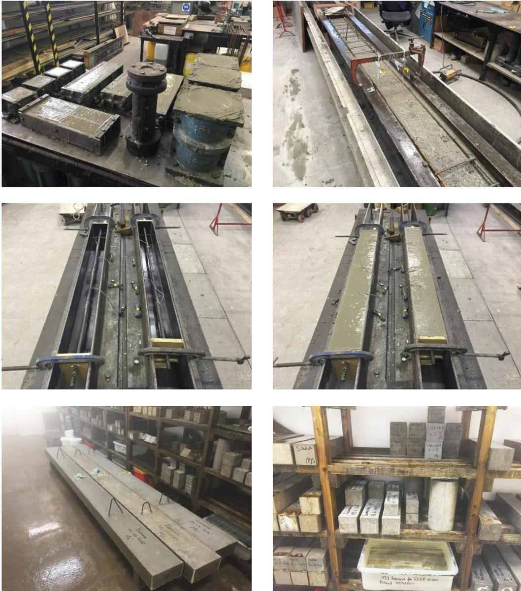
Figure 4-10 Casting and curing of specimens
