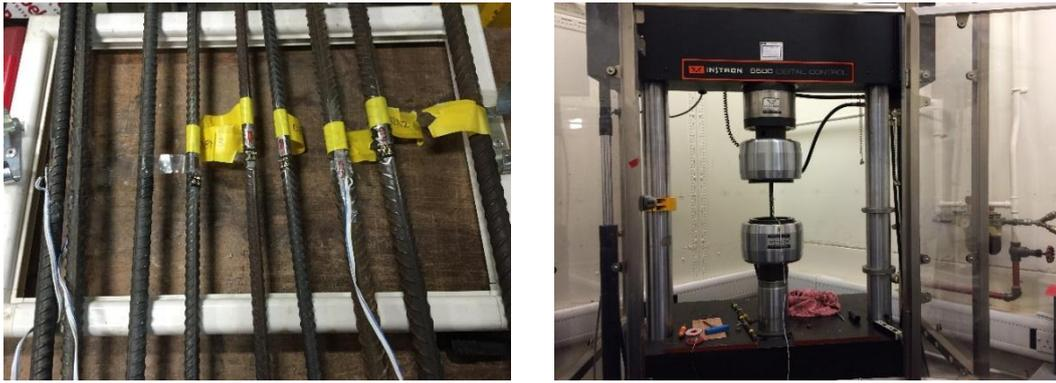
Figure 4-7 Uni-axial tensile test of steel bars
