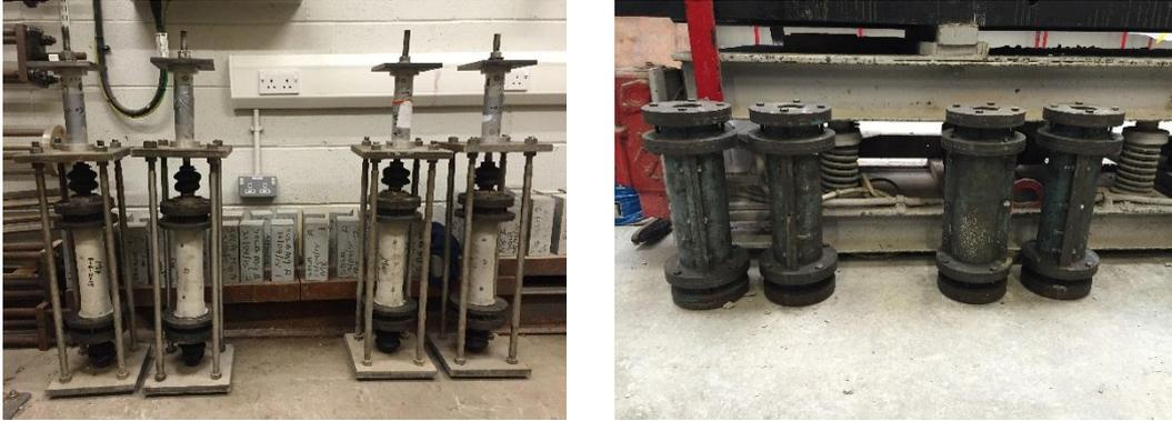
Figure 4-19 Tensile creep test
