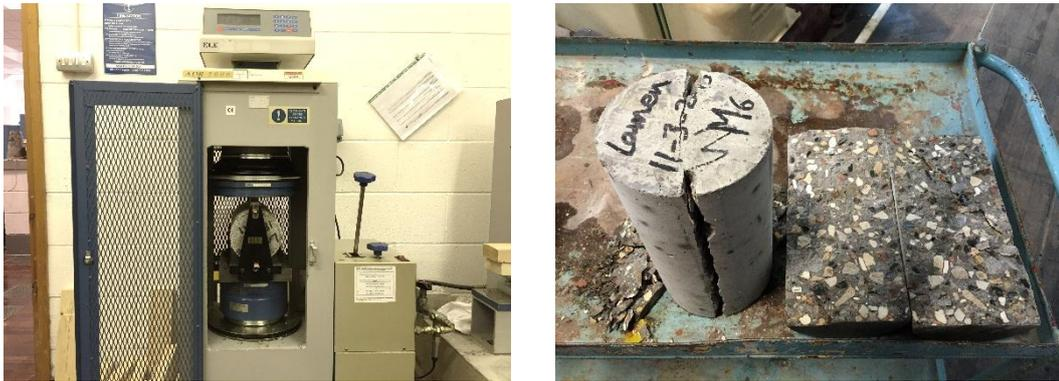
**Figure 4-12 Splitting tensile strength test**
