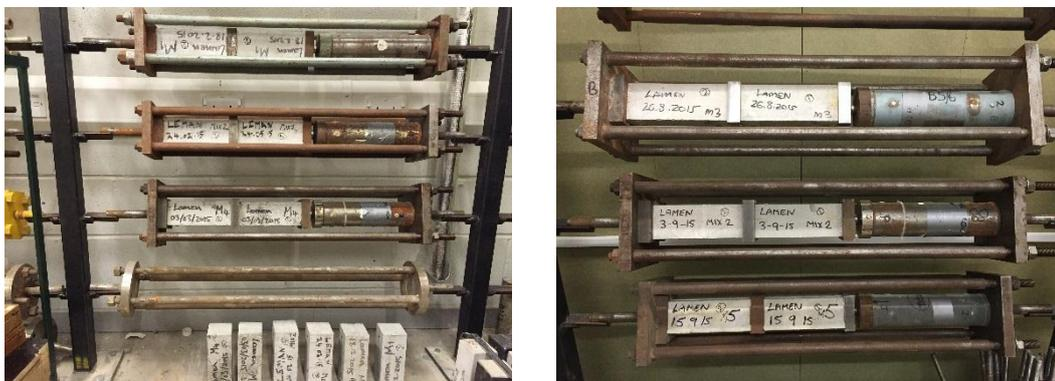
Figure 4-18 Compressive creep test
