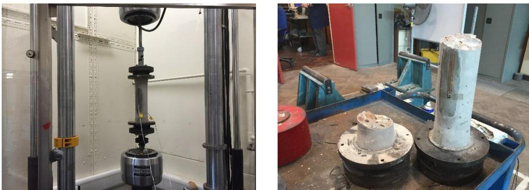
**Figure 4-13 Direct tensile strength test**
