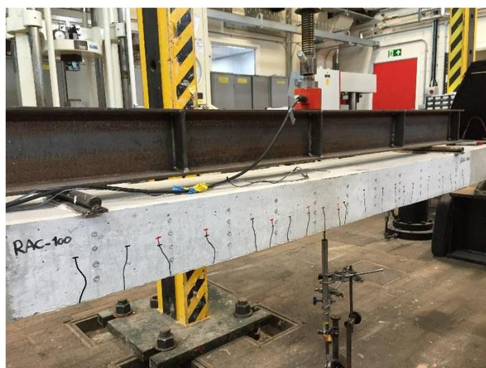
Figure 5-22 Effect of recycled aggregate on cracking pattern
