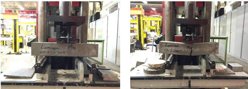
Figure 4-14 Flexural strength test
