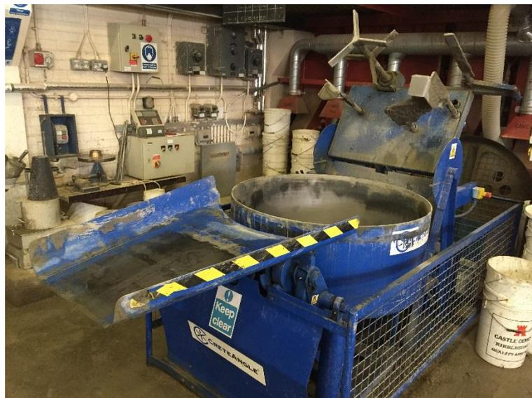
Figure 4-9 Mechanical drum mixer
