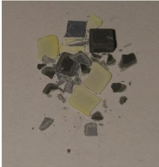
Figure 42: Oxidized specimen of the alloy MG1 at 1200 °C, after its removal from the sample holder
