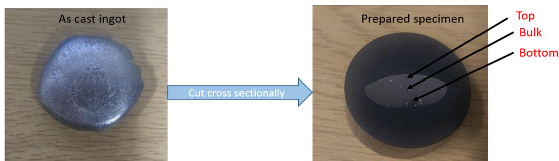
Figure 31: a labelled diagram showing where the samples have been obtained
