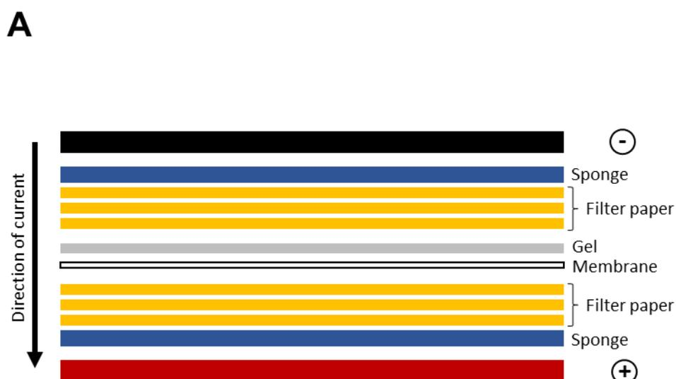
**Figure 2.9: Schematic of the transfer stack in which protein was transferred from the gel onto the PVDF membrane**
