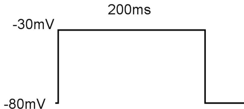
**Figure 2.10: Schematic of the square wave pulse used in patch clamp experiments**
