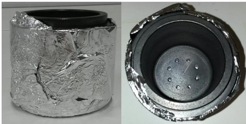
**Figure 108:** Aluminium foil wrapped around a graphite liner for “waste” aluminium anode electrochemical experiments.
