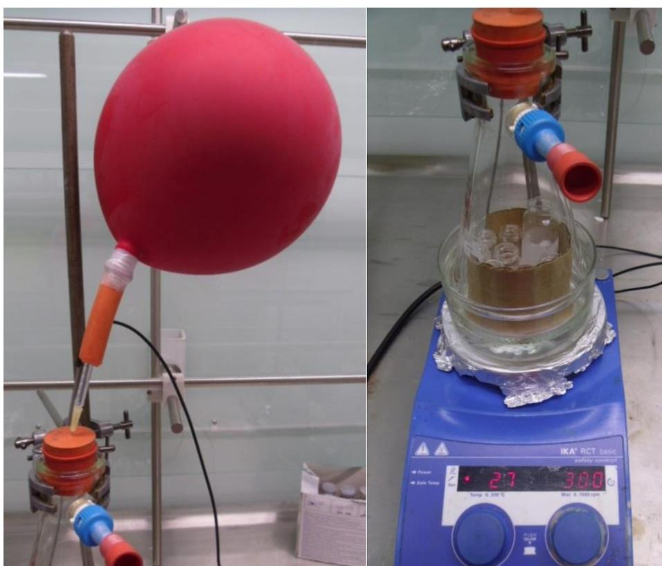
**Figure 27:** Experimental setup for testing chromium(III) salophen catalysts in converting epoxides to cyclic carbonates.
