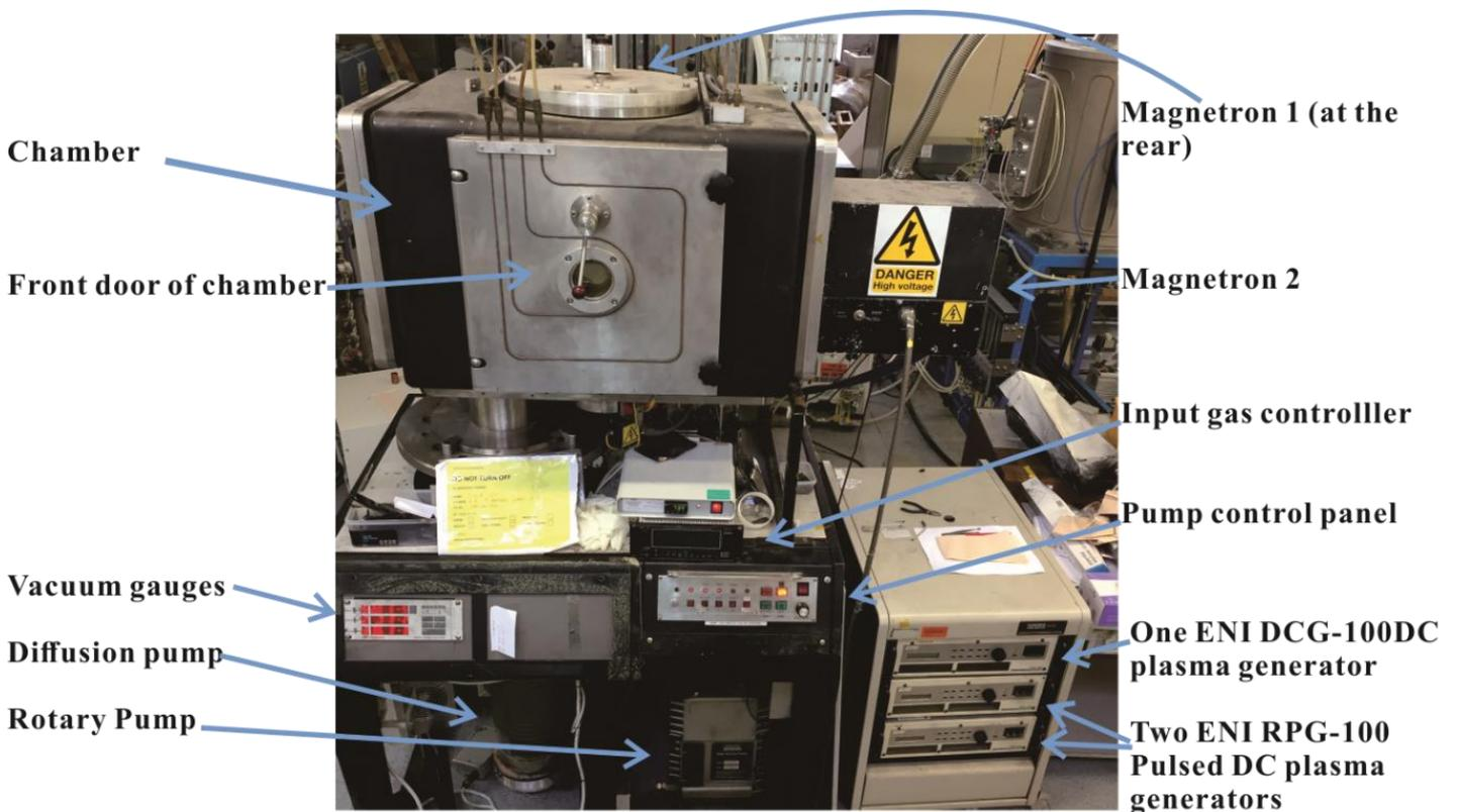
*Figure 4.2 The Nordiko unbalanced magnetron sputtering*
