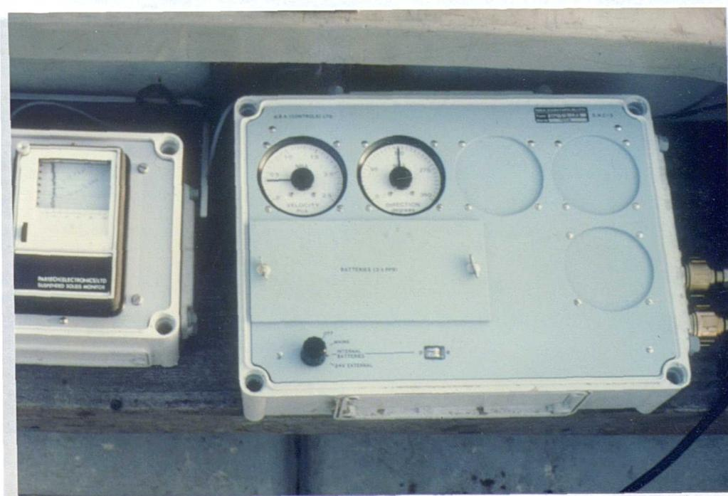
Plate 2.3 Current Meter Recording Equipment -
