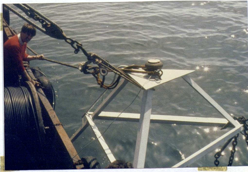
Plate 2.1 Installation of Wave Recorder.
