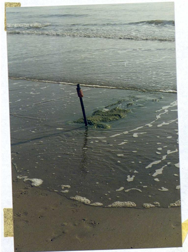
Plate 2.7 Tracer Sand after the Passage of the First Few Waves Following Injection.
