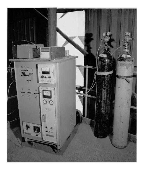
PLATE 17 - LAND electrochemical probe-analyser used for determination of NO and  $SO_2$  concentrations at the base of chimney
