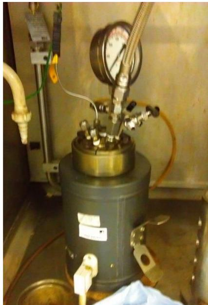
**Figure 3.1.** Reactor used for high pressure thermal hydrolysis of food waste and microalgae.
