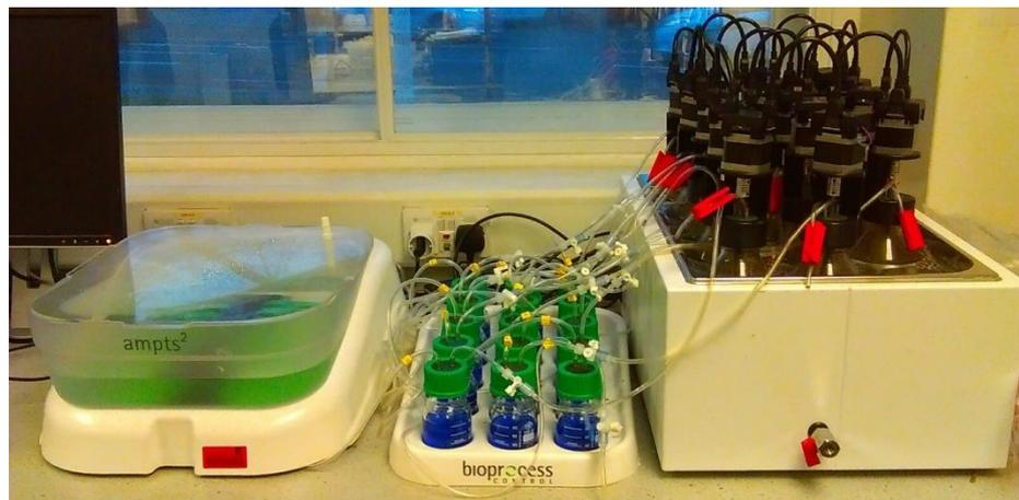
**Figure 3.3.** Fermentations ran in semi-continuous stirred reactors using a AMPTS II equipment (Bioprocess Control Sweden AB).
