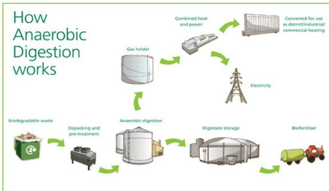
**Figure 2.10.** Process flow diagram for anaerobic digestion with food waste (WRAP, 2013).
