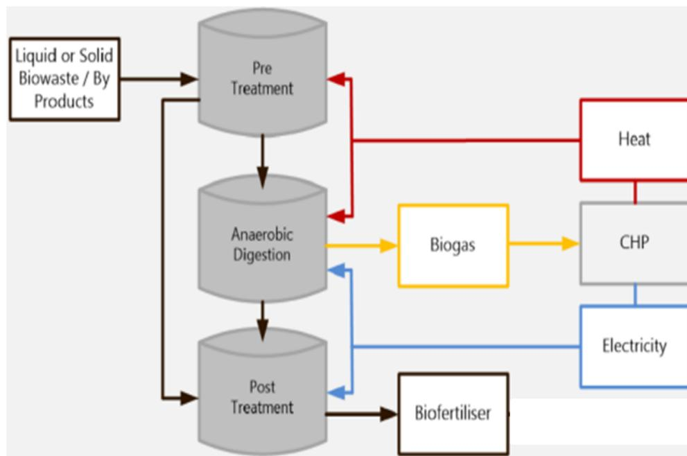
**Figure 2.9.** Process scheme to produce energy from waste activated sludge. (DEFRA, 2012b).
