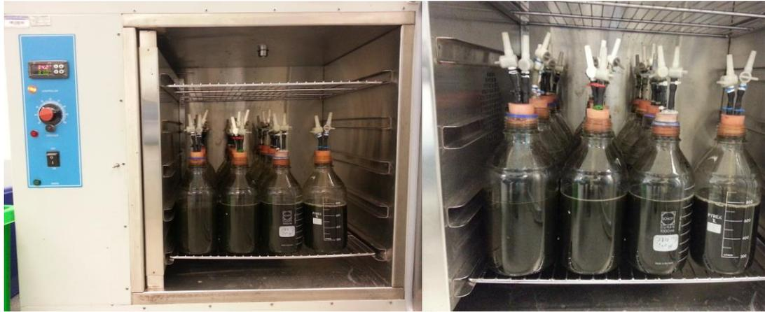
**Figure 3.2.** Reactors used in the mixed anaerobic fermentation of WAS and different organic substrates.
