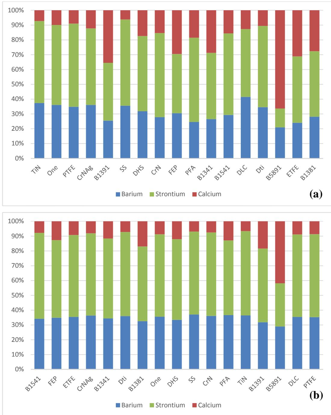
**Figure 5.12. Mole percentage of calcium, barium and strontium existing on the surface as scale deposits in the *deposition* process: (a) Laminar and (b) Turbulent flow conditions.**
