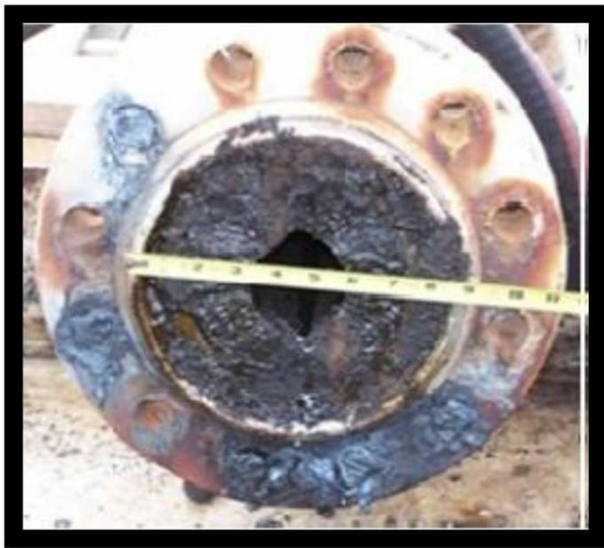
**Figure 1.2. Flowline clogged by scale [6].**
