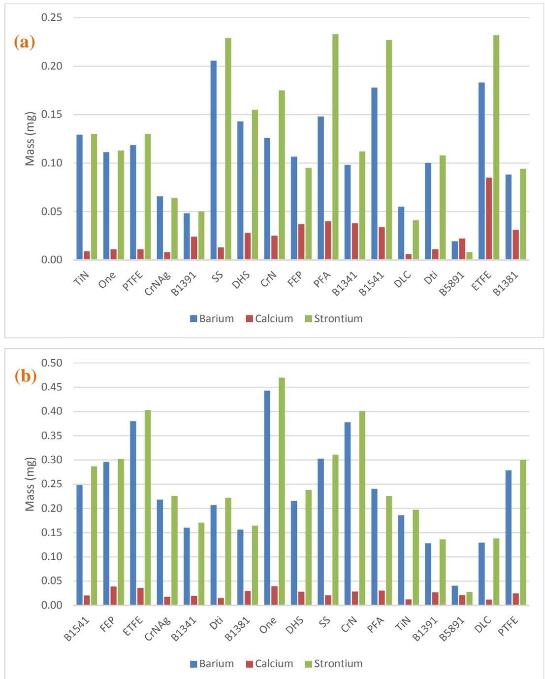
**Figure 5.10. ICP results of the scale deposits in the *deposition* tests presented in mass gain: (a) Laminar and (b) Turbulent flow conditions.**
