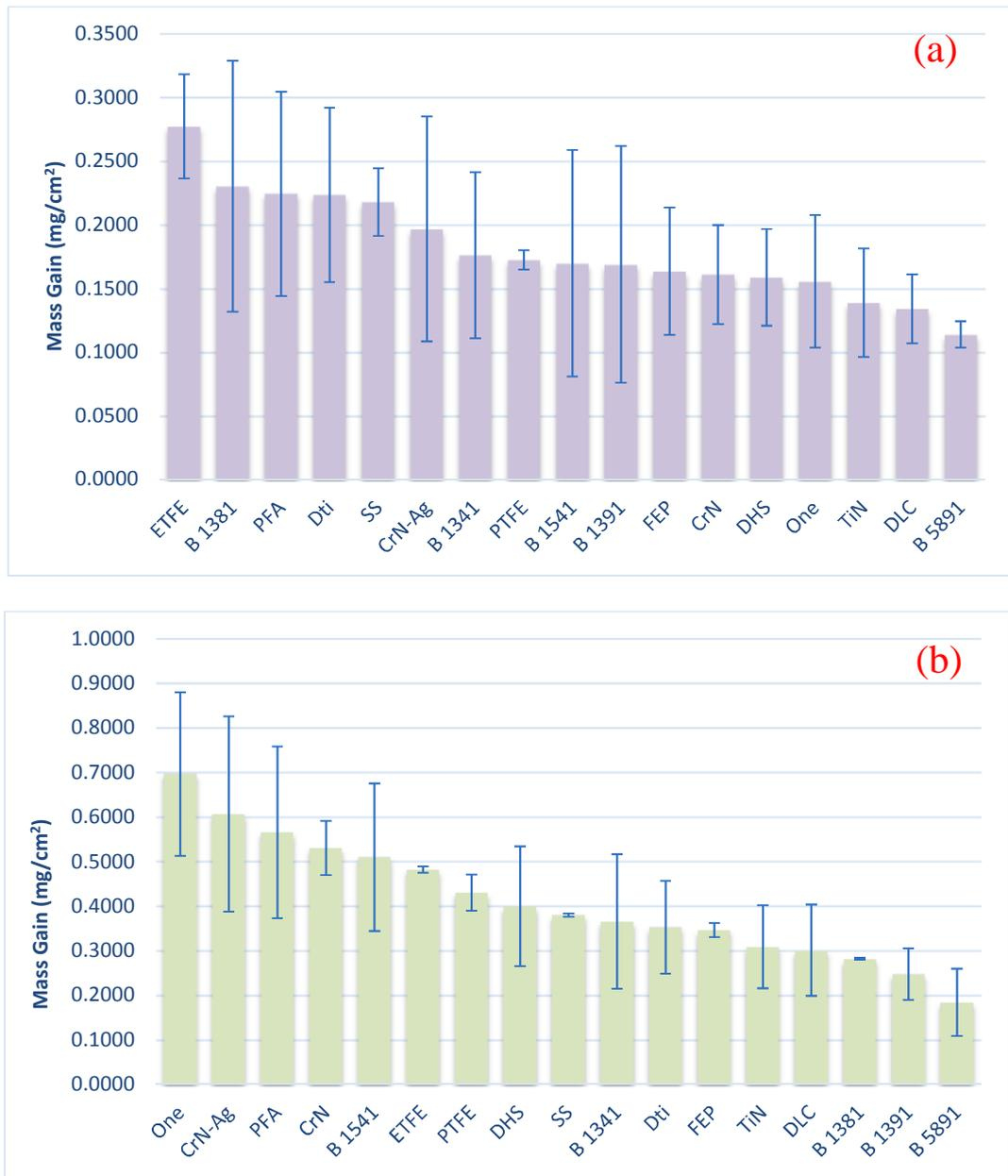
**Figure 5.1. Scale deposits formed on different modified substrates in the deposition tests, where the focus is on heterogeneous nucleation and crystal growth, in (a) laminar and (b) turbulent conditions.**
