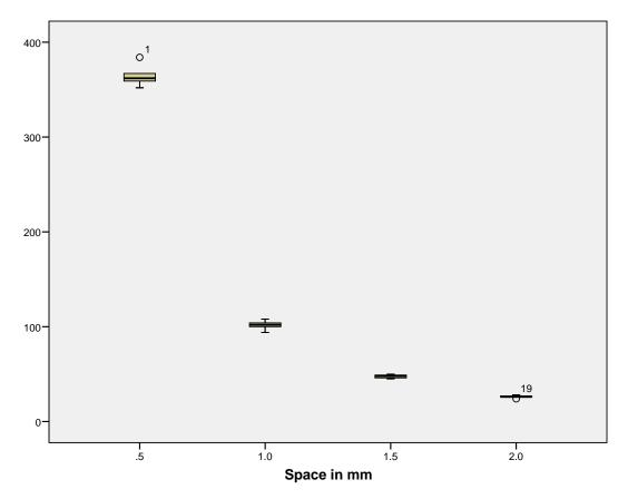
Figure 66 Box plot of results space under the impression tray against pressure
