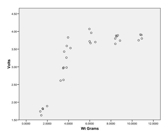
Figure 19 scatter plot of weight versus output of pressure sensor
