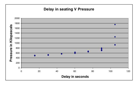
Figure 35 All the results from the 'delay' experiment; delay versus pressure
