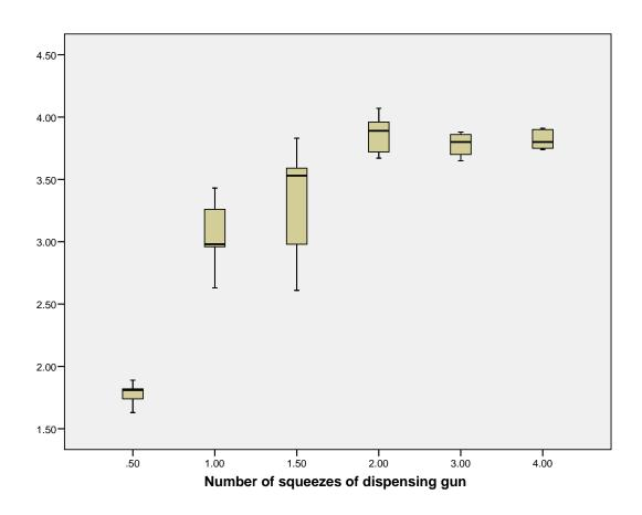
Figure 24 Box and whisker plot of voltage output from the pressure sensor versus number of pull of dispensing gun trigger
