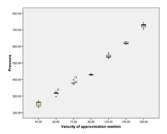
Figure 63 Box plot of results for the medium bodied regular set silicone; velocity against pressure
