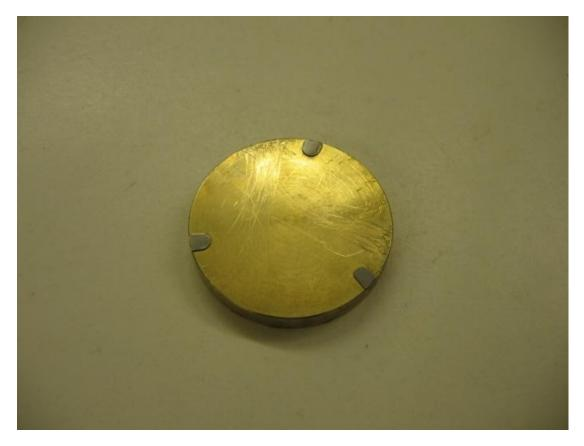
Figure 34 The 'impression tray' for the 'delay' experiment, note the steel spacers.
