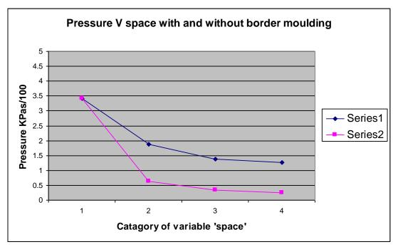
Figure 69 Series 1 is results from impressions with border adaptation to create peripheral gap of 0.5mm; series 2 is with an unrestricted periphery.
