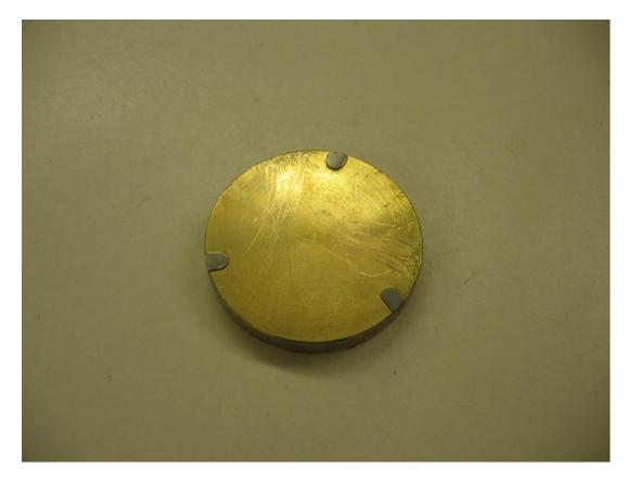
Figure 3 An 'impression tray' used to carry impression material note the stainless steel 'spacers' made from engineers' 'feeler gauges'.
