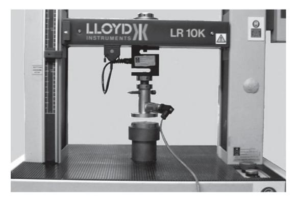
Figure 27 Lloyd Universal Testing Machine with brass discs and sensors attached.
