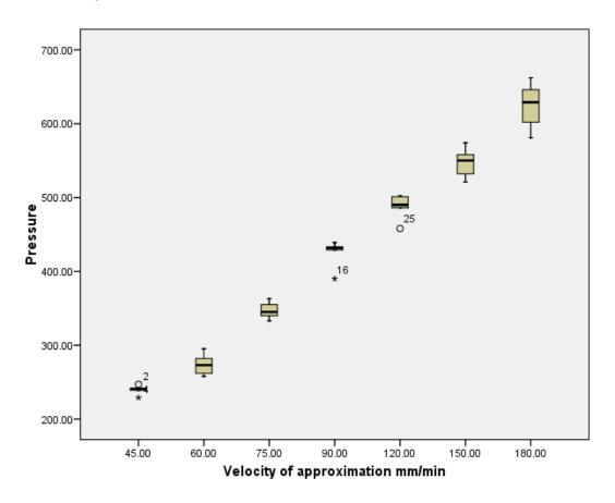
Figure 64 Box plot of results for the light bodied fast set silicone; velocity against pressure
