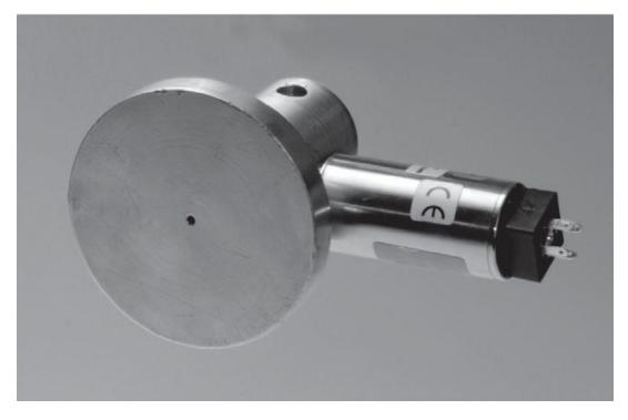
Figure 26 Sensor attached to brass disc with 2mm hole at centre.
