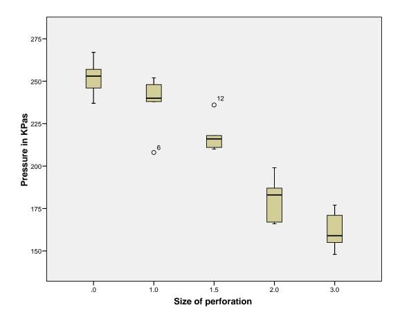
Figure 60 Box plots of results for the size of a perforation
