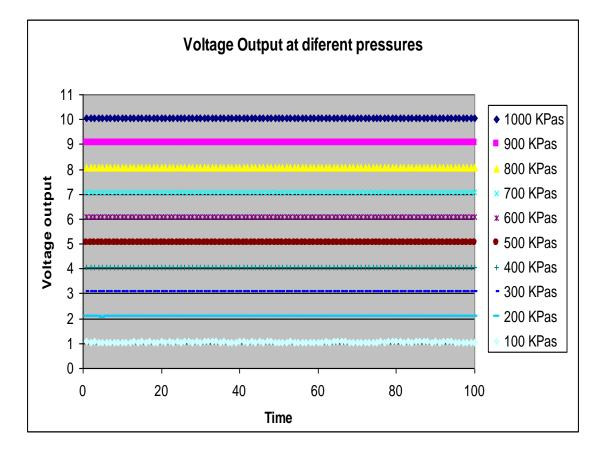
Figure 10 Output from sensor at 10 nominal pressures.
