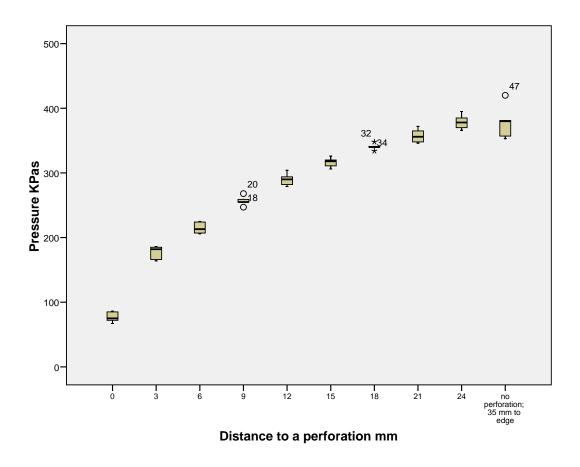
Figure 42 Box plot of results for the 'distance to a perforation' experiment
