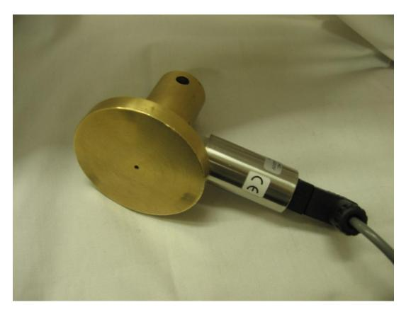
Figure 44 standard impressed disc with sensor attached
