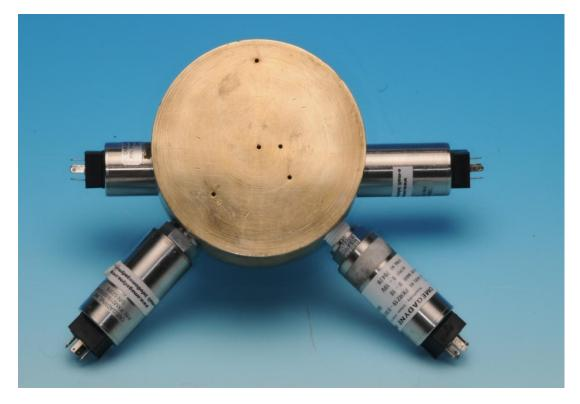
Figure 37 disc used for the experiment to investigate the position of the pressure sensor within the impression
