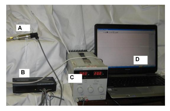
Figure 73 the pressure sensing equipment
