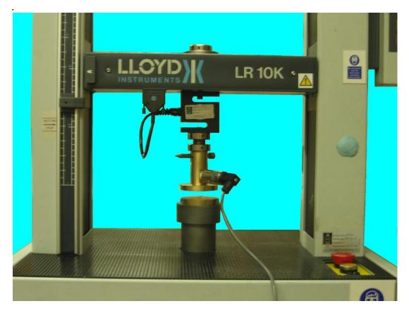
Figure 4 the Lloyd machine with the brass discs mounted
