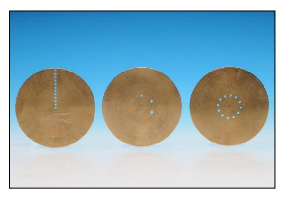
Figure 52 The disc for the distance study is on the left the disc for the size study is in the centre and the number study on the right.
