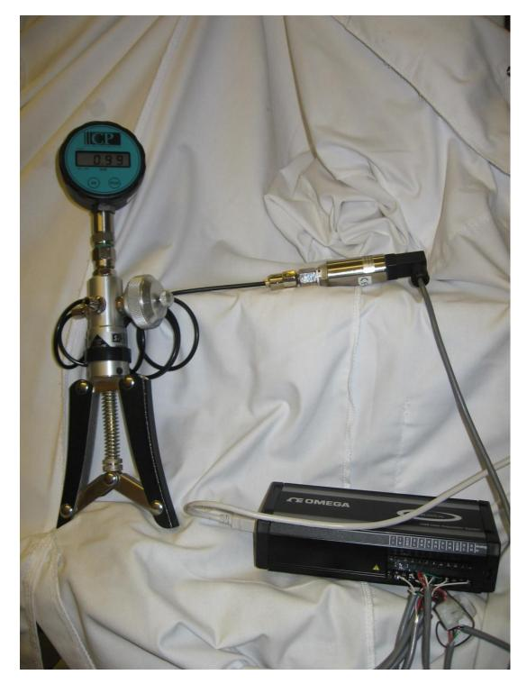
Figure 9 Combined pressure gauge and pneumatic hand pump used to hold the sensor at standard pressures for the precision data collection.
