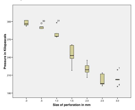
Figure 50 Box plots of results for the perforation size experiment
