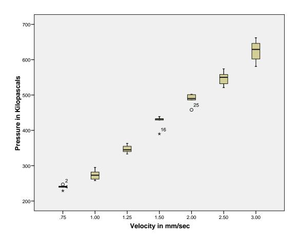
Figure 31 Box and Whisker plot of velocity versus pressure
