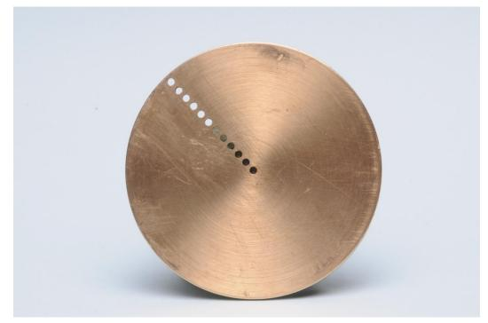
Figure 41 The 'impression tray' for the distance to a perforation experiment
