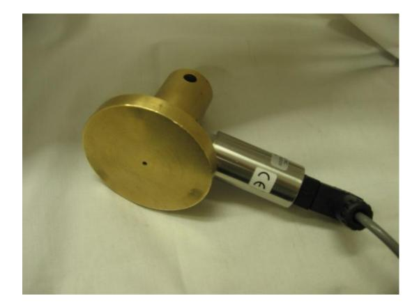
Figure 33 The disc used for the 'delay' impressions with the pressure sensor attached.
