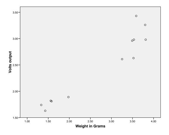
Figure 20 Scatter Plot of weight versus output voltage where there was no overflow of silicone.
