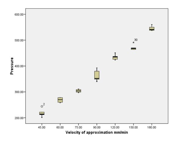
Figure 62 Box plot of results for the light bodied regular set silicone; velocity against pressure
