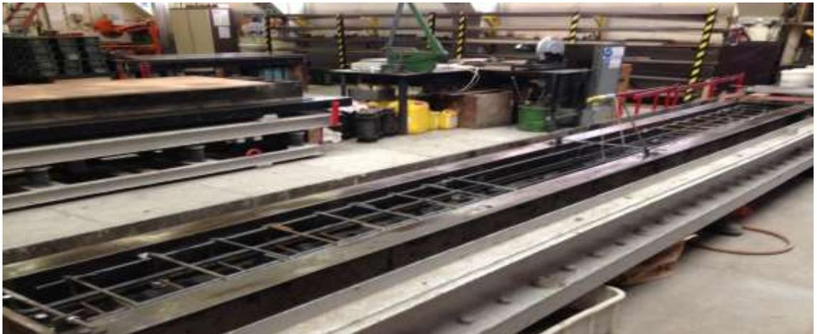
Figure 3-3: Steel formwork with reinforcement cage
