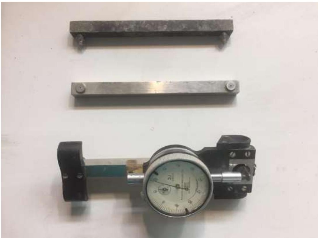
Figure 3-12: 150 mm of DEMECs gauge, calibrated bar and fitting bar
