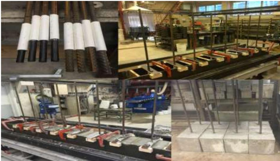
Figure 3-15: Preparation of pull-out specimen
