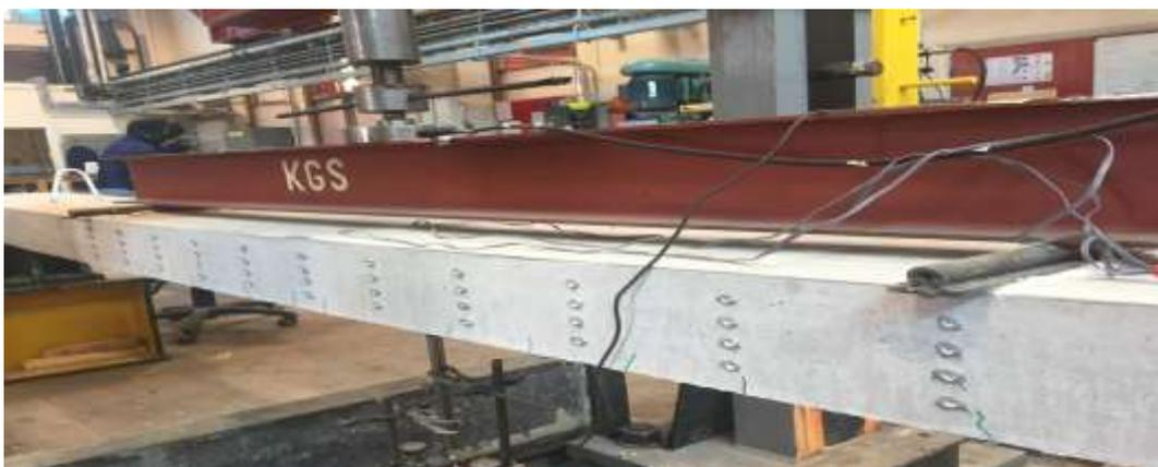
Figure 3-8: DEMEC point layout
