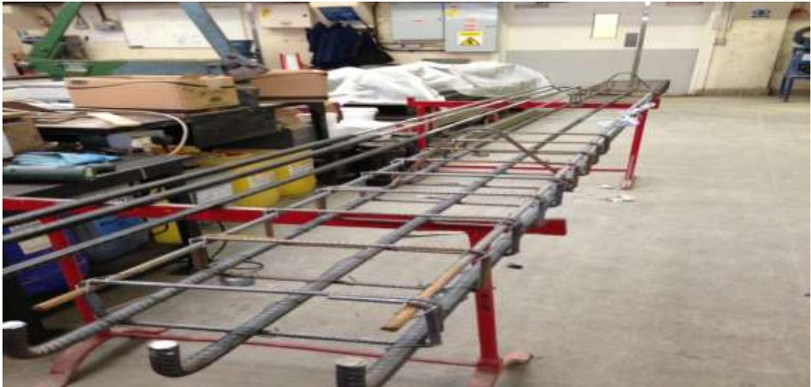
Figure 3-4: Steel reinforcement beam cage
