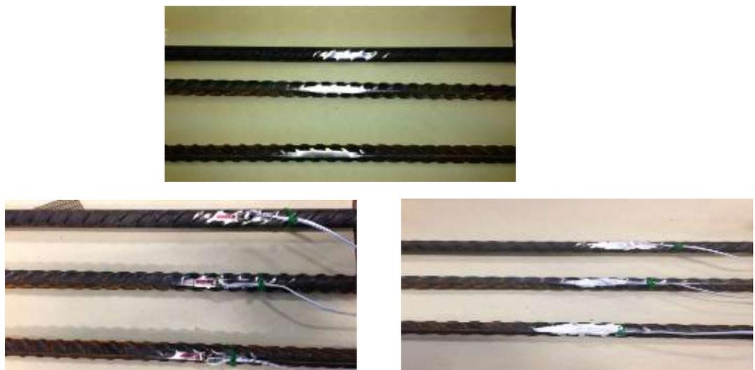
Figure 3-7: Strain gauges installation
