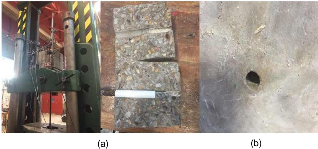
Figure 4-3: Failure mode through pull-out test a) Bonded samples, b) Unbonded samples
