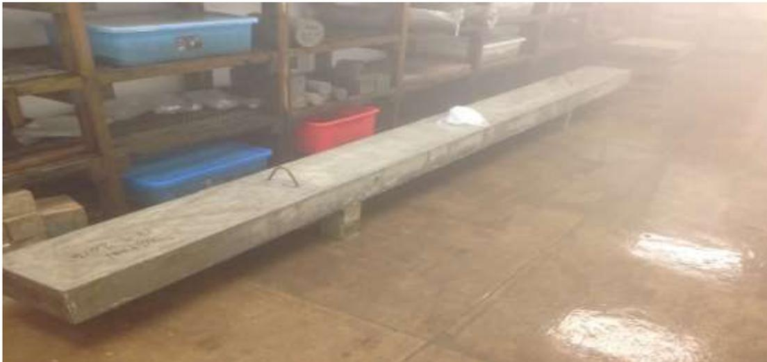
Figure 3-6 Beam in the curing room
