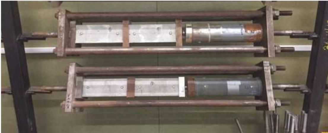
Figure 3-13: Creep rig test
