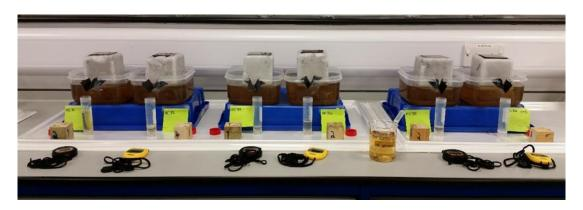
**Figure 5.5** Experiment set-up of surface peat samples to measure *K* using the modified cube method.
