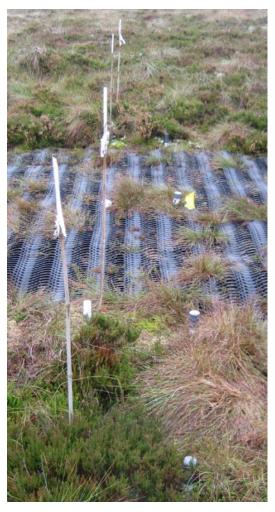
**Figure 6.3** Dipwells and crest-stage tubes installed in the field along transects across the track (plastic mesh).
