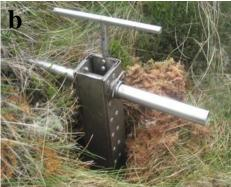
**Figure 5.3** a) Insertion of corer with three fixed sides into peat, surface was cleared of vegetation and compression was minimal. b) Corer with fourth side in place prior to core extraction.
