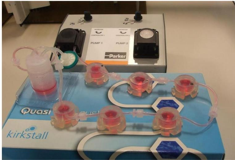
Figure 2.1: The Quasi-vivo® bioreactor set-up.
