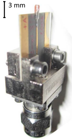
Figure 6.3: A photograph of the loop target attached to a circuit board with SMA connection.
