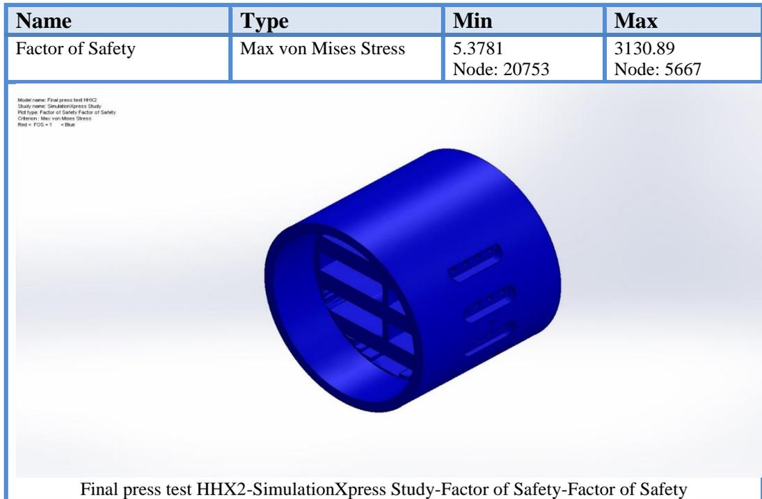
**Figure A3-7:** Simulation of factor of safety of the hot heat exchanger at 400°C, done by the SolidWorks
