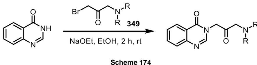
To prepare the starting bromo ketones **349**, the corresponding  $\beta$ -amino ketone was anticipated to be brominated on the least hindered part of the ketone. The  $\beta$ -amino ketone bearing the dimethyl amine substituent **350** was obtained commercially whilst two more examples were prepared using Azizi's method.<sup>162</sup> Accordingly, the conjugate
