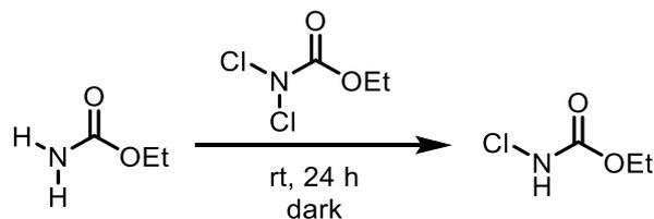
Urethane (4.57 g, 51.3 mmol, 1.0 eq.) and *N,N*-dichlorourethane (6.0 mL, 51.3 mmol, 1.0 eq.) were combined and stirred at rt in the absence of light for 18 h. The title compound was obtained as a yellow/green oil (12.6 g, 99%).  $^1\text{H}$  NMR (400 MHz,  $\text{CDCl}_3$ )  $\delta$  6.54 (s, 1H), 4.24 (q,  $J = 7.0$  Hz, 2H), 1.30 (t,  $J = 7.0$  Hz, 3H).  $^{13}\text{C}$  NMR (101 MHz,  $\text{CDCl}_3$ )  $\delta$  157.5 (-), 64.2 (-), 14.9 (+).
