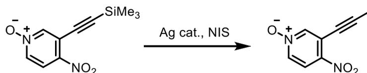
4-Nitro-3-[(trimethylsilyl)ethynyl] pyridine 1-oxide **141** (0.300 g, 1.27 mmol, 1.0 eq.) and silver fluoride (0.161 g, 0.050 mmol, 0.05 eq.) were dissolved in DMF (5 mL) in a flask wrapped in aluminium foil. A solution of *N*-iodosuccinimide (0.286 g, 1.27 mmol, 1.0 eq.) in DMF (5 mL) was added and the reaction mixture was stirred at ambient temperature under a stream of N<sub>2</sub> for 5 h. The solvent was removed under reduced pressure and the
