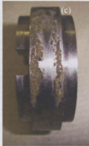
Figure 4.22 Leaf layers after (a) a dry test and (b) a wet test and (c) the hard layer left after a wet test. Figure 4.23 shows the indentations produced during the hardness test on the leaf layer. Some times during the hardness testing cracks appeared. It is because the layer areas are fragile. When the load was applied, cracking was generated in the axial direction.
