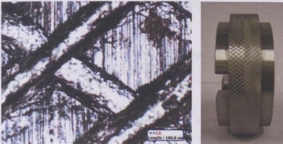
Figure 6.2 Textured disc ( $R_a 9.89 \mu\text{m}$ ).
