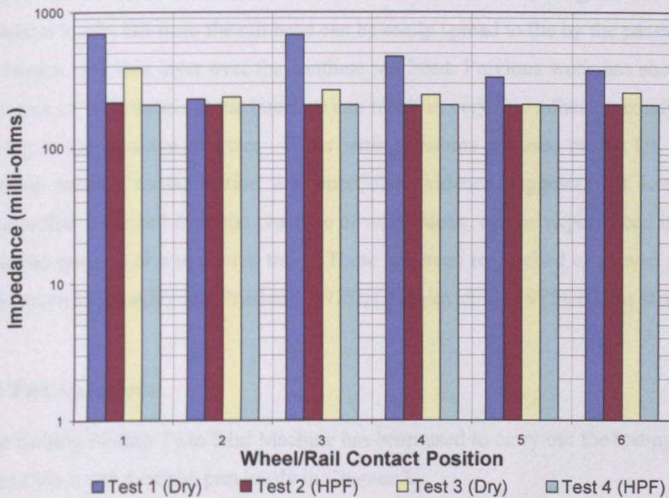
Figure 5.12 Measured static impedance values for dry and HPF conditions wheel/rail disc.
