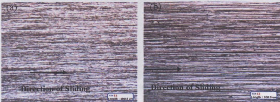
Figure 4.25 (a) Rail and (b) Wheel Surfaces after Oil Tests.
