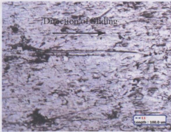
Figure 4.26 Wheel disc surface damage due to the interaction with dry leaves.
