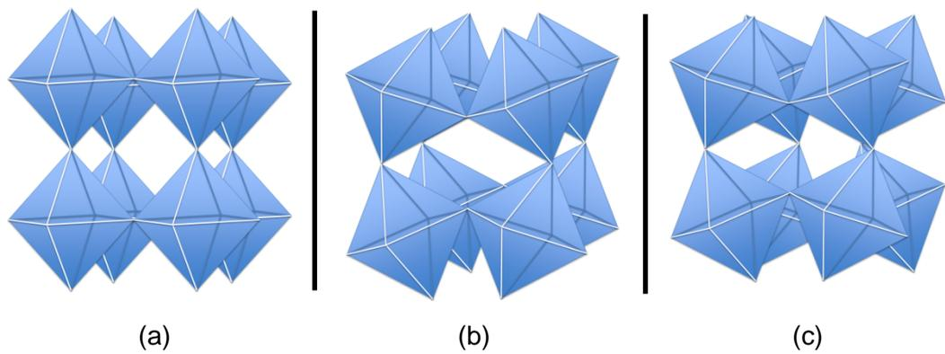
**Figure 1-8 The octahedra tilt in 3 variations. a) No tilt b) In phase tilt c) anti-phase tilt. No tilts are observed on the y and z axis in this illustration.**
