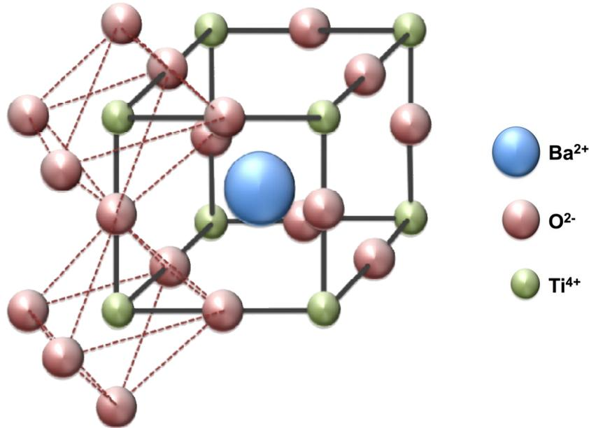
Figure 1-6 BaTiO<sub>3</sub> unit cell with the B site ion at the origin, showing the oxygen octahedral cage in 3 dimensions
