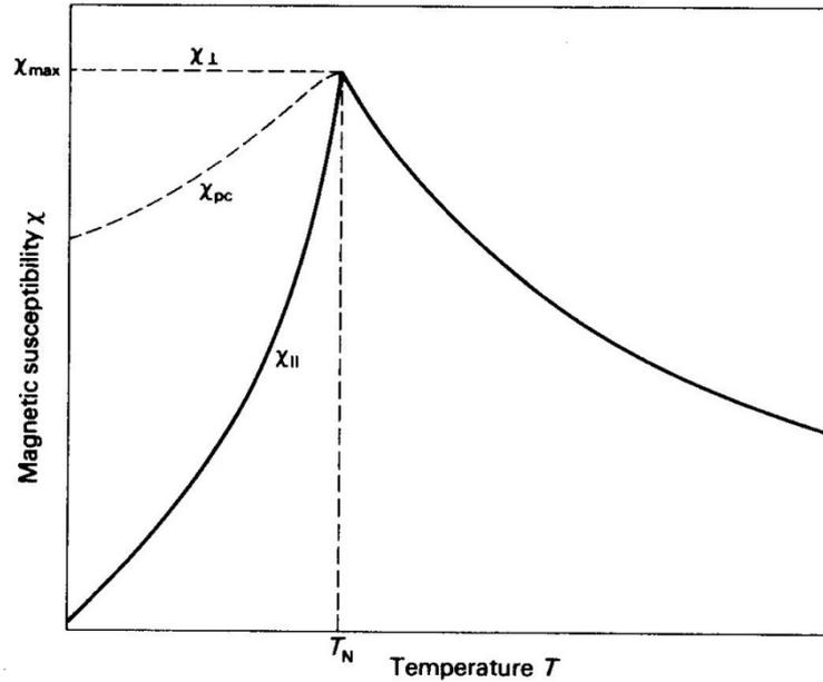
Figure 1-32 Expected susceptibility of a simple antiferromagnetic single crystal with applied field parallel (||) and perpendicular ( $\perp$ ) to spin alignment, and polycrystal (pc) (Crangle, 1977. p.69).
