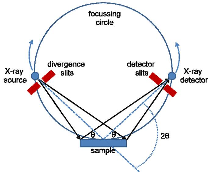
**Figure 2-5 Schematic of Bragg-Brentano geometry for powder XRD.**
