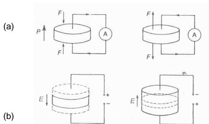
**Figure 1-16 Illustration of the a) Direct and b) Converse piezoelectric effect (Moulson, 2003. p.340)**
