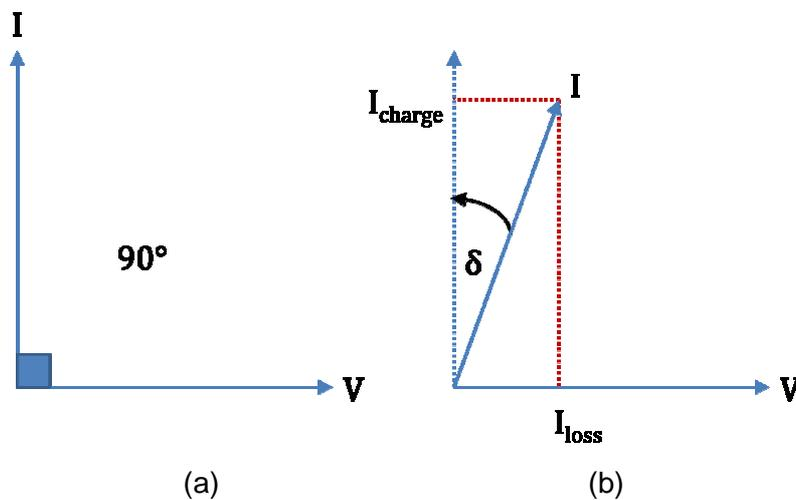
Figure 1-11 Phasor diagram for (a) an ideal dielectric and (b) a real dielectric exhibiting a dielectric loss
