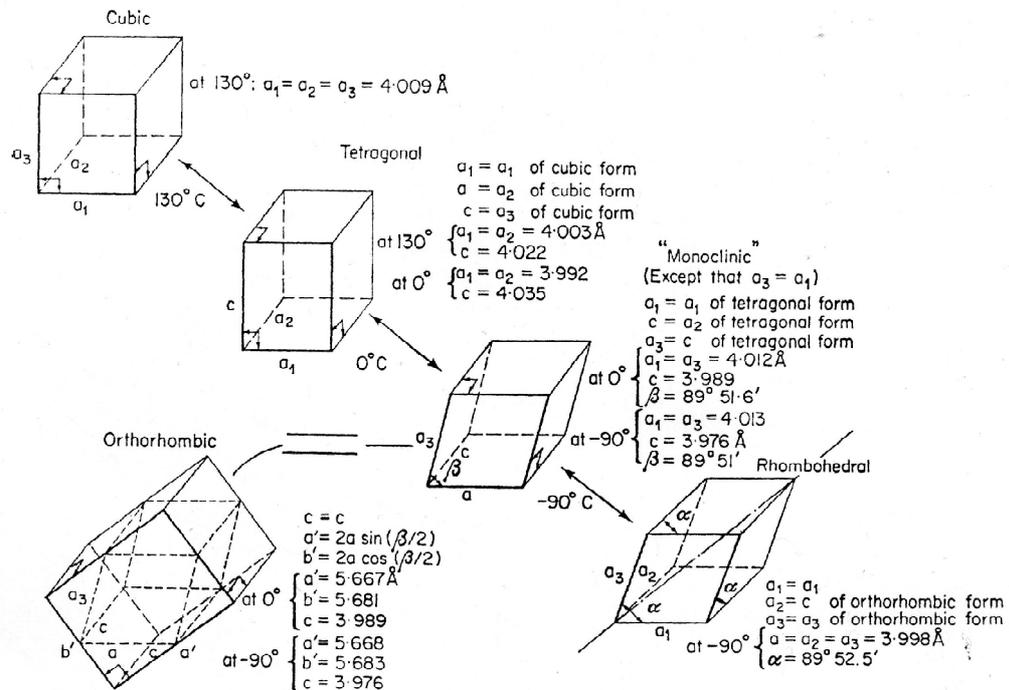
Figure 1-15 Illustration of the phase changes of barium titanate as a function of temperature, from non-polar cubic, through polar tetragonal, orthorhombic and rhombohedral structures. (Jaffe, 1971. p. 54)
