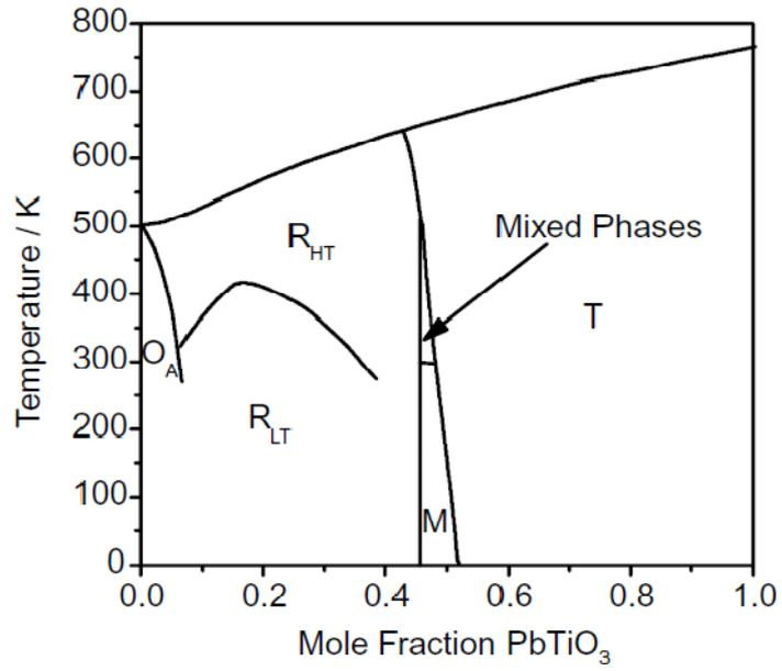
Figure 1-19 Phase diagram of the  $\text{Pb}(\text{Zr}_x\text{Ti}_{1-x})\text{O}_3$  system from Noheda et al, 1999 (Bell, 2006).
