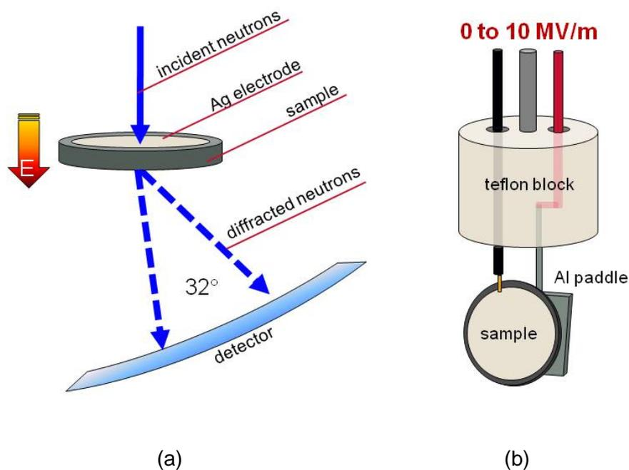
Figure 3-7 (a) Schematic of the experimental geometry and (b) modified sample stick with sample for the E2 instrument at HMI, Berlin, Germany.
