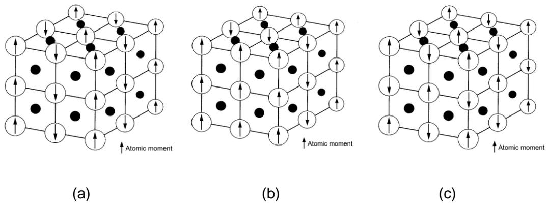
Figure 1-33 Antiferromagnetic groups a) C-type b) A-type and c) G-type (adapted from Crangle, 1977).
