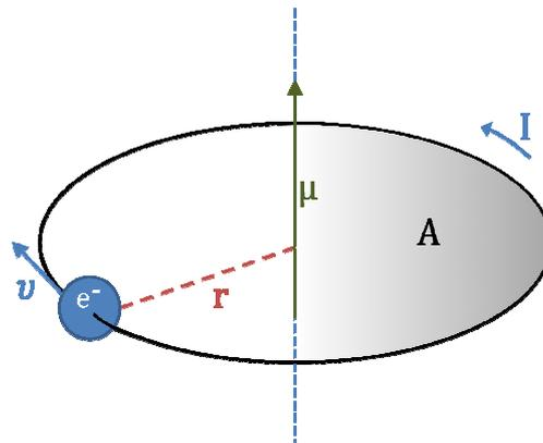
**Figure 1-22 Illustration equating current (I) in a loop of area (A) to an electron orbit with radius (r) and velocity (v) to form a magnetic moment (μ).**
