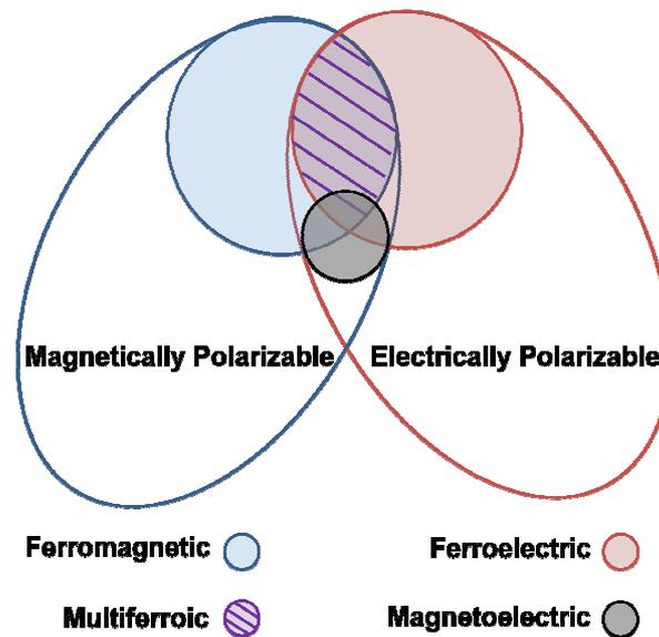
**Figure 1-36 The relationship between magnetolectric and multiferroic materials (Reprinted by permission from Macmillan Publishers Ltd; Nature. (Eerenstein, 2006).**
