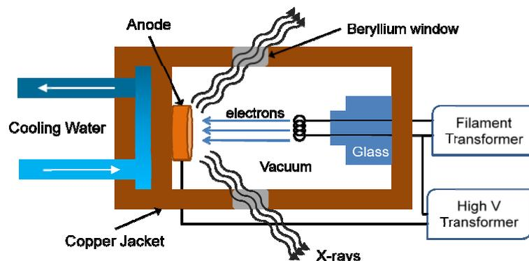
Figure 2-3 Schematic of an X-ray tube (adapted from Cullity, 2007).
