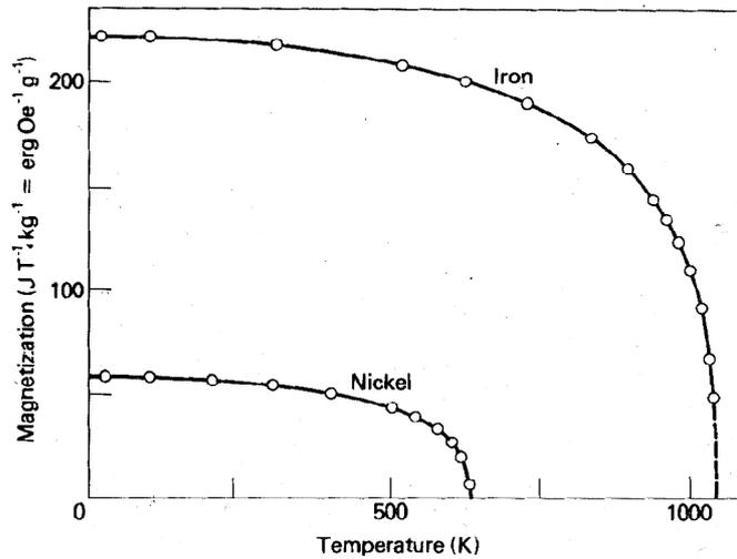
**Figure 1-24 Spontaneous magnetization values as a function of temperature for iron and nickel (Crangle, 1977.)**
