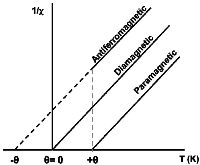
Figure 1-23 Plot of the inverse of volume susceptibility as a function of temperature. The x intercept value defines the type of magnetism present in the sample (adapted from Blundell, 2001. p. 93)
