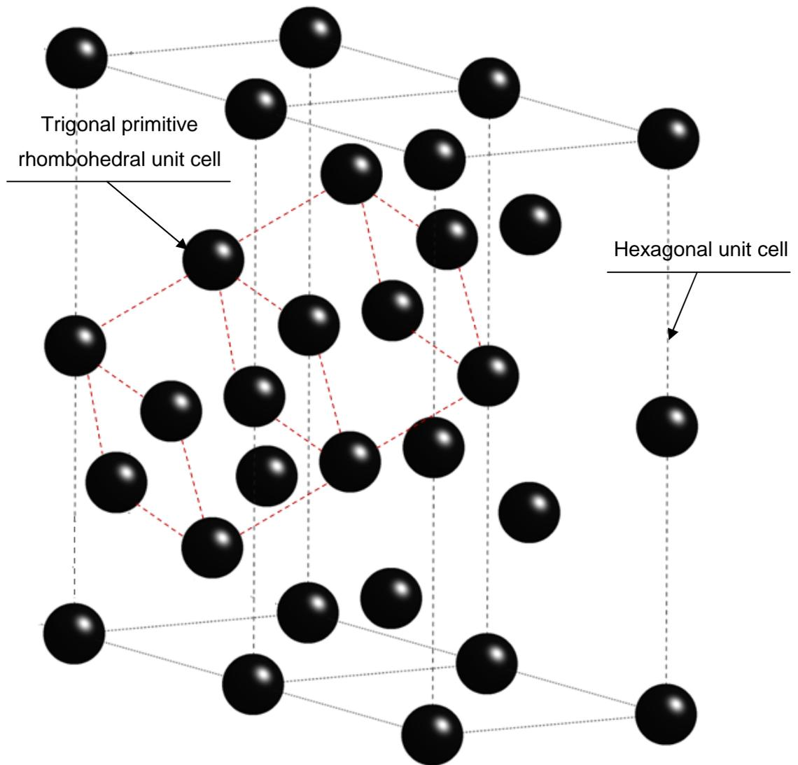
Figure 1-9 An example of the rhombohedral lattice system whereby the atoms can arrange to be grouped in the hexagonal or trigonal (within) crystal system.
