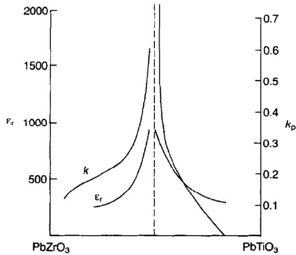
Figure 1-21 Coupling Coefficient ( $k_p$ ) and permittivity values across the PZT compositional range (Moulson, 2003. p. 356)
