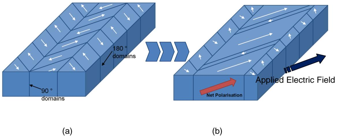
**Figure 1-13 Schematic of a) domain configuration in barium titanate below  $T_c$  and b) the effect on domains with applied electric field.**
