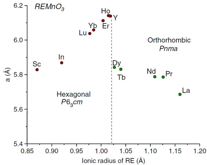
**Figure 1-39 Structure of  $REMnO_3$  as a function of RE ionic radius.**
