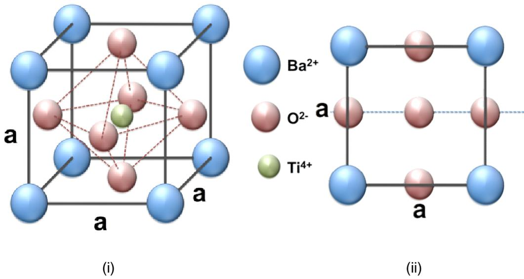
Figure 1-5 Cubic structure of BaTiO<sub>3</sub> (i) in 3d and (ii) projected along the [100] above T<sub>c</sub>
