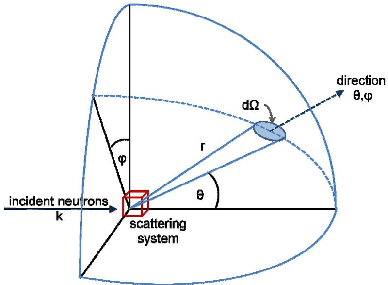
Figure 2-8 Geometry of scattering experiment (adapted from Squires, 1978. p.5.)
