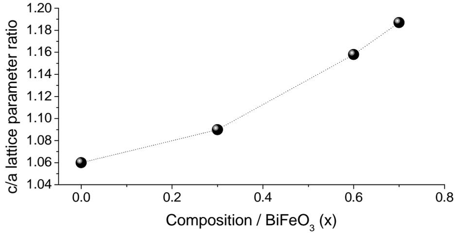
Figure 1-43 Plot of c/a lattice parameter ratios with increased additions of bismuth ferrite to the solid solution (values taken from Sai Sunder, 1995).
