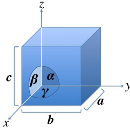
Figure 1-1 A unit cell with the Cartesian axis' (x,y,z), lattice vectors (a,b,c) and angles between them ( $\alpha,\beta,\gamma$ ) (recreated from Callister, 2000 p.38)
