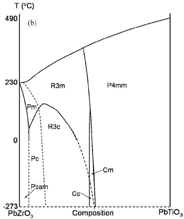
Figure 1-20 Phase diagram of the  $\text{Pb}(\text{Zr}_x\text{Ti}_{1-x})\text{O}_3$  system proposed by Woodward et al (2005).
