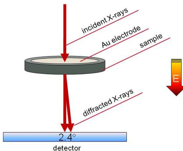
**Figure 3-8 Schematic of the experimental geometry on the E2 synchrotron instrument at the ESRF, Grenoble, France.**
