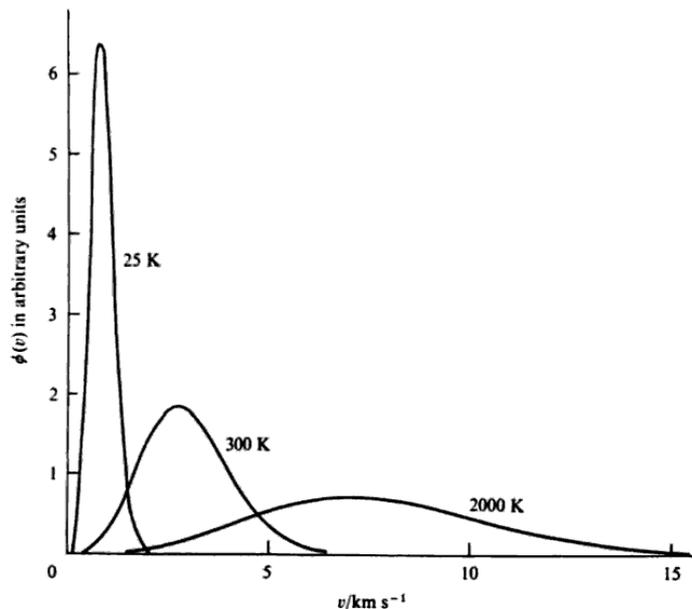
Figure 2-10 Neutron flux distribution as a function of velocity for  $T = 25, 300$  and  $2000$  K (Squires, 1978. p. 4).
