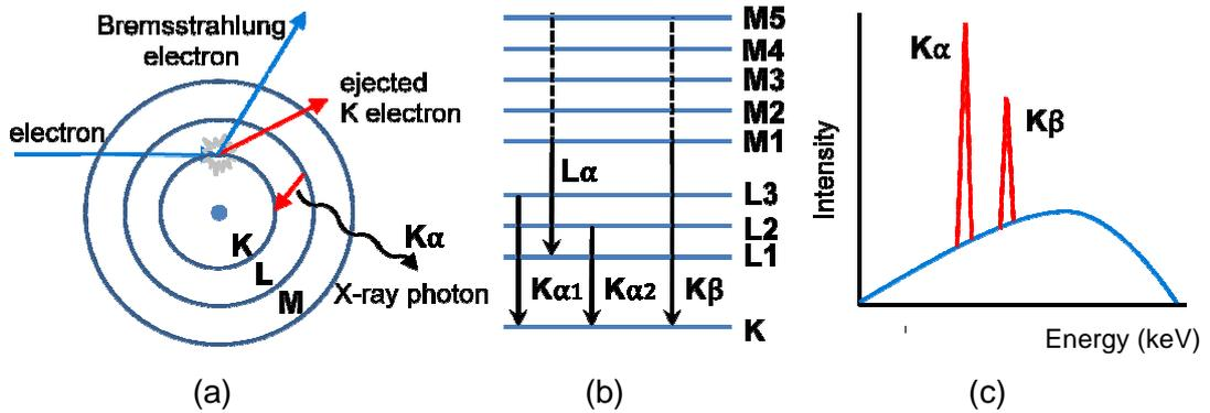
**Figure 2-4** Illustration of the production of the characteristic X-ray spectrum from a) electron interaction, b) the relative shell energy c) and the profile superimposed over the continuous spectrum.
