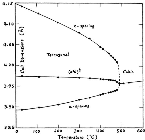
**Figure 1-17 Lattice parameters as a function of temperature for lead titanate sintered powder from X-ray diffraction data (Shirane, 1950).**
