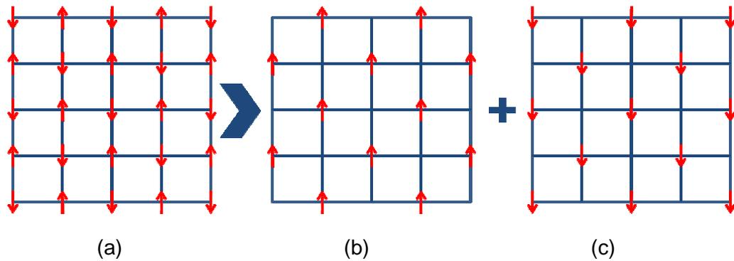
Figure 1-29 Two sublattices having moments opposite to each other from b)  $H \uparrow$  and c)  $H_m \downarrow$  for example, to create a) an antiferromagnetic lattice. (adapted from Blundell, 2001. p. 92)
