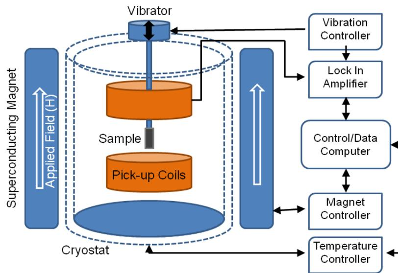
Figure 2-1 Schematic of a vibrating sample magnetometer
