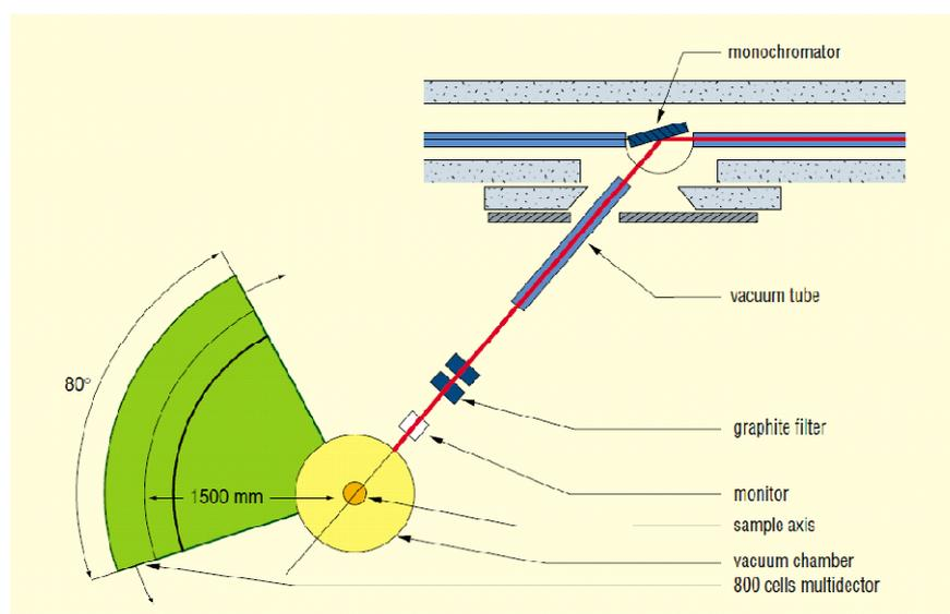
**Figure 3-3 Schematic of the G4.1 constant wavelength diffractometer at LLB (André, 2003)**
