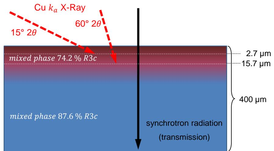
**Figure 4-11 Graphic illustrating the penetration of X-ray radiation normal to the sample surface.**
