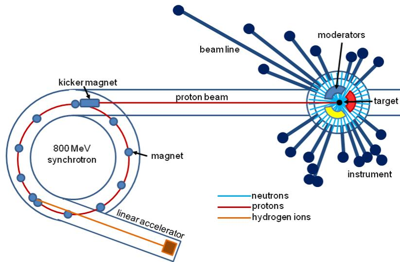
**Figure 2-11 Illustration of ISIS neutron spallation source (adapted from Bennington, 2006. p.11)**
