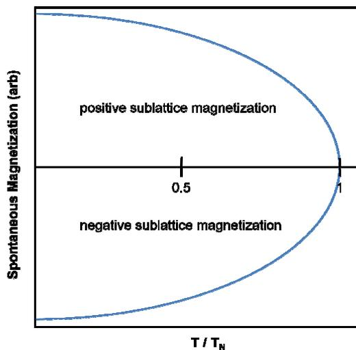
Figure 1-30 Spontaneous magnetization of the sublattices in a simple antiferromagnet (adapted from Crangle, 1977. p. 63)
