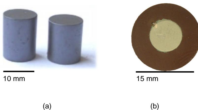
**Figure 4-1 Photographs of bulk polycrystalline ceramics in a) cylindrical form and b) disc (pellet) form. The disc is shown with a small silver electrode for electrical measurements.**
