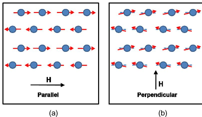
Figure 1-31 Application of a) parallel and b) perpendicular magnetic fields ( $H$ ) to a simple antiferromagnetic material (adapted from Cragle, 1977).
