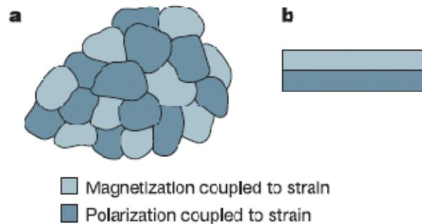
**Figure 1-37 Magnetolectric strain coupling by mixing two phases of piezomagnetic and piezoelectric material as a) a mixture of grains or b) as composite layers (Reprinted by permission from Macmillan Publishers Ltd; Nature. (Eerenstein, 2006).**
