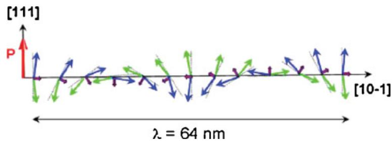
**Figure 1-42 Schematic representation of the spin cycloid. Canted antiferromagnetic spins (blue and green) give rise to a net magnetic moment (purple) that is averaged out to zero due to the incommensurate modulation. The spins are contained within the plane defined by the polarization vector (red) and the cycloidal propagation vector (black) (Lebeugle, 2008).**
