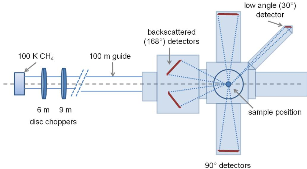
**Figure 3-4 Schematic of the high resolution neutron powder (HRPD) diffractometer at ISIS, Oxford, UK.**
