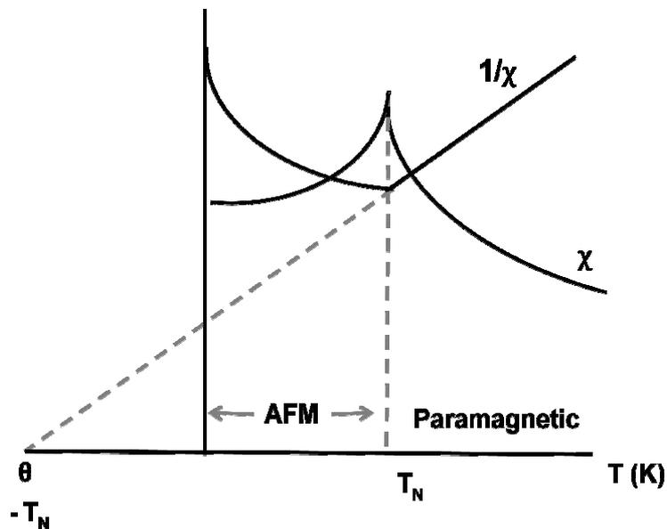
Figure 1-28 An illustration of magnetic susceptibility as a function of temperature for an antiferromagnetic material (adapted from Cullity, 1972. p.156)
