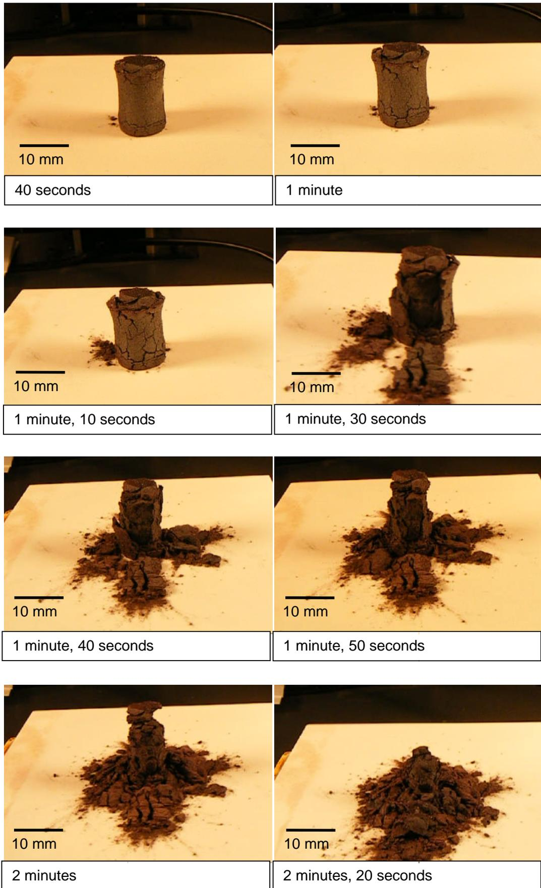
**Figure 4-2 A series of screen shots taken from a video recording over 2.5 minutes of a BFPT 7030 10 mm dia. cylinder cooling from 1100 °C after sinter.**
