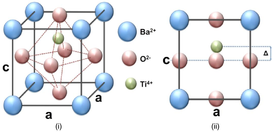
Figure 1-4 Perovskite structure of BaTiO<sub>3</sub> (i) in 3d and (ii) projected along the [100] exhibiting the non-symmetric position (exaggerated) of the B ion (Ti) below T<sub>c</sub>
