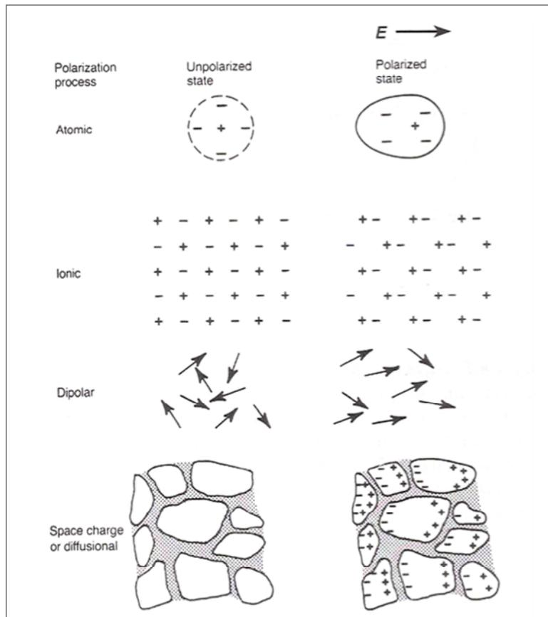
**Figure 1-10 The 4 mechanisms of polarization; atomic, ionic, dipolar and diffusional (Moulson, 2003)**
