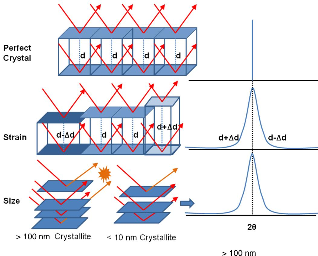
**Figure 2-6 Illustration of peak broadening in a diffractogram from strain and crystallite size. X-rays (red) diffract from unit cell planes (blue) in phase to form constructive interference peaks or destructive interference annihilation (orange).**
