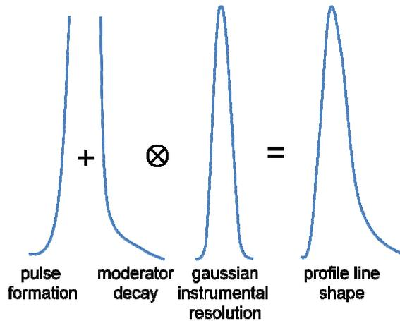
**Figure 2-12 Illustration (exaggerated) of the complex peak line shape as a result of spallation source neutron formation and moderation (adapted from Bennington, 2006. p. 38).**
