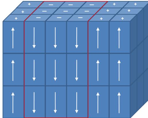
**Figure 1-12 Illustration of 180° domain formation with a single domain of similarly polarised unit cells outlined in red.**
