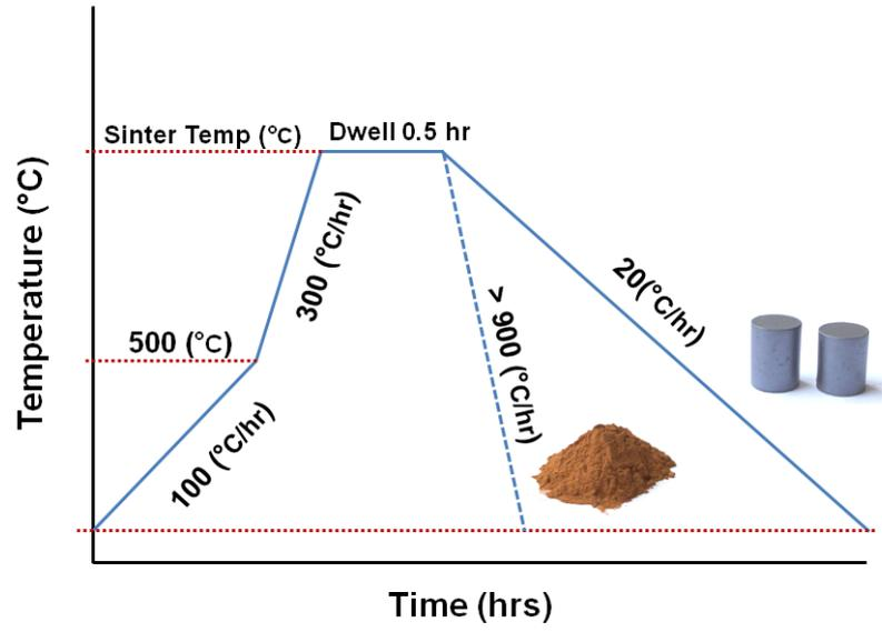
Figure 3-1 Furnace routine for synthesis of various forms of  $\text{BiFeO}_3 - \text{PbTiO}_3$
