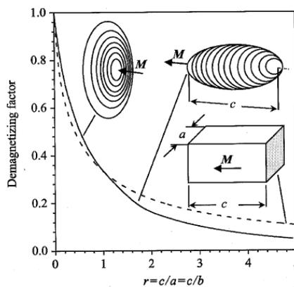
Figure 1-27 Plot of demagnetizing factor as a function of sample dimension ratio (Fiorillo, 2004)
