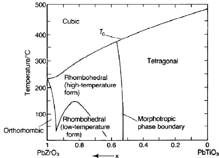
Figure 1-18 Phase diagram of the  $\text{Pb}(\text{Zr}_x\text{Ti}_{1-x})\text{O}_3$  system from 1971
