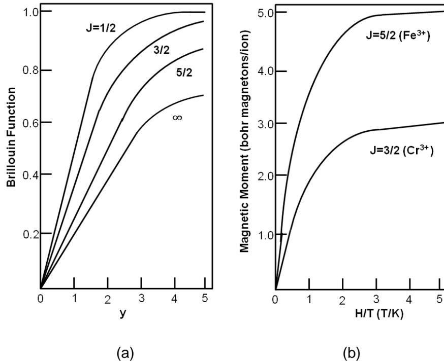
Figure 1-26 Brillouin function curves where a) Brillouin function vs. small values of  $y$  for  $J = 1/2, 3/2, 5/2$  and  $\infty$ , and b) Brillouin curves for  $J = 5/2$  and  $3/2$  for  $\text{Fe}^{3+}$  and  $\text{Cr}^{3+}$  respectively on a plot of Magnetic moment vs. Field-Temperature ratio (adapted from Crangle, 1977. p.28-29)
