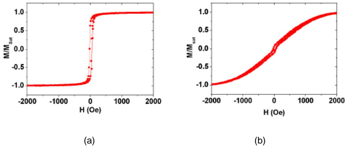
**Figure 2-2 Examples of VSM hysteresis loops of thickness dependent magnetic Co/Ru multilayers. Thick samples are a) ferromagnetic, whilst thinner films present b) antiferromagnetism (Kinane, 2008).**
