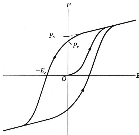
Figure 1-14 Hysteresis loop schematic of typical ferroelectric behaviour. Origin ( $O$ ), coercive field ( $E_c$ ) remnant ( $P_r$ ) and spontaneous ( $P_s$ ) polarization are labelled along electric field ( $E$ ) and polarization ( $P$ ) axis.
