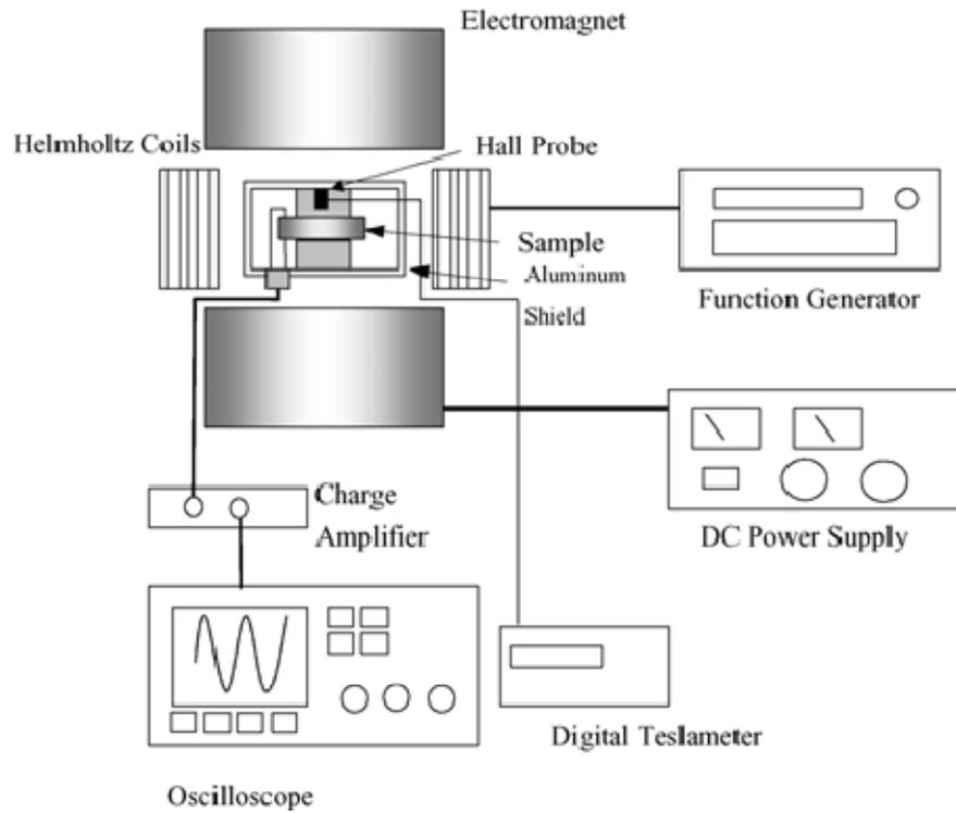
**Figure 1-38 Schematic of a ME measurement system (Reprinted by permission from Springer; J. Electroceramics. (Ryu, 2002. p.112)**
