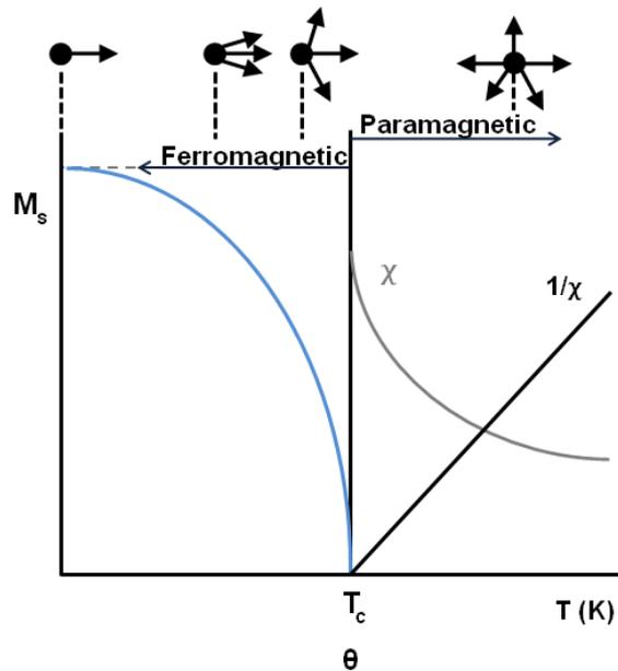
**Figure 1-25 Magnetization and susceptibility curves below and above the Curie temperature with sketches at the top to indicate distribution of magnetic moment direction with zero applied field within a domain (below  $T_c$ ) and a group of atoms (above  $T_c$ ). (Adapted from Cullity, 1972. p.127)**
