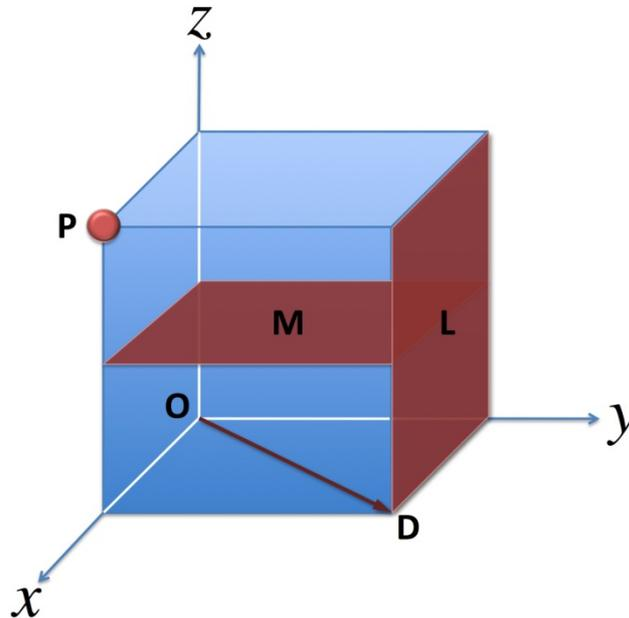
Figure 1-3 A unit cell labelled with a point (**P**), direction (**D**) and plane (**L**)
