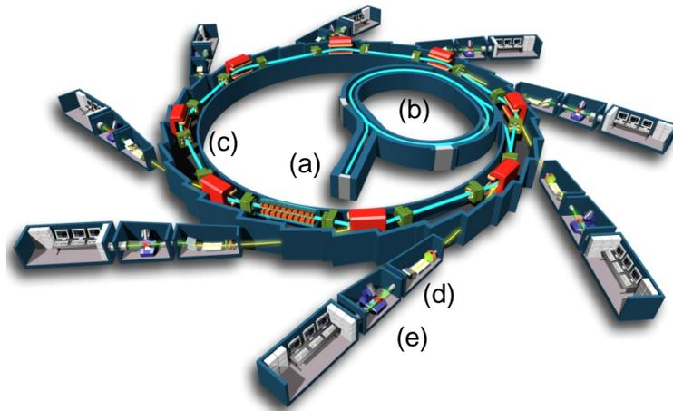
**Figure 2-7 Schematic of a synchrotron illustrating the path of electrons (blue) through a) the linear accelerator, b) booster ring, c) storage ring with bending magnets (red) and the resultant X-ray photons emitted (yellow) to d) the beamlines optics and e) experimental hutches (reproduced with permission, Chaix & Morel, 2005.)**
