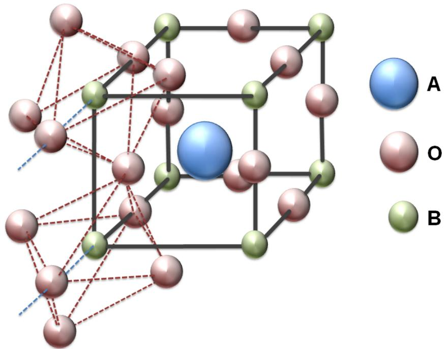
**Figure 1-7 Perovskite unit cell showing an example of the oxygen octahedra tilt and its effect on neighbouring cages**
