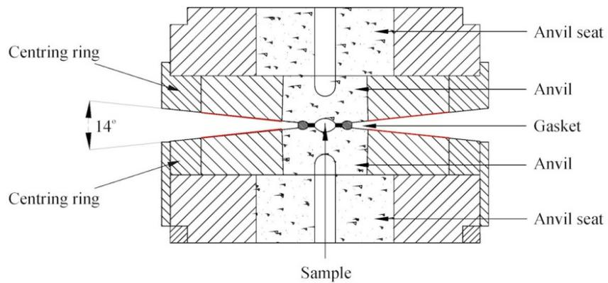
Figure 3-6 Schematic of the Paris Edinburg cell gasket and anvil setup. The red lines indicate presence of cadmium shielding, and the incident beam enters from the top. (Godec, 2004.)
