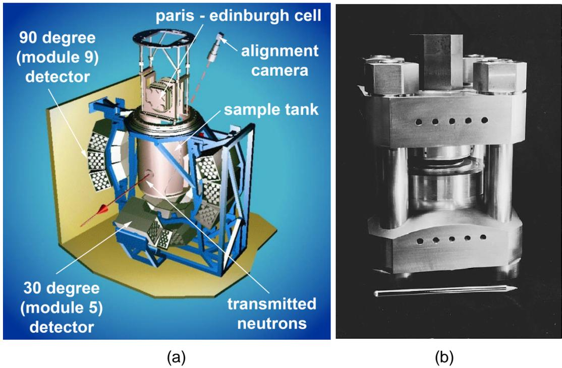
Figure 3-5 (a) The PEARL beam line and instrument setup at ISIS, Oxford, UK. (Pearl, 2010) (b) The Paris Edinburg cell used at PEARL (pencil shown for scale) (Klotz, 1995)
