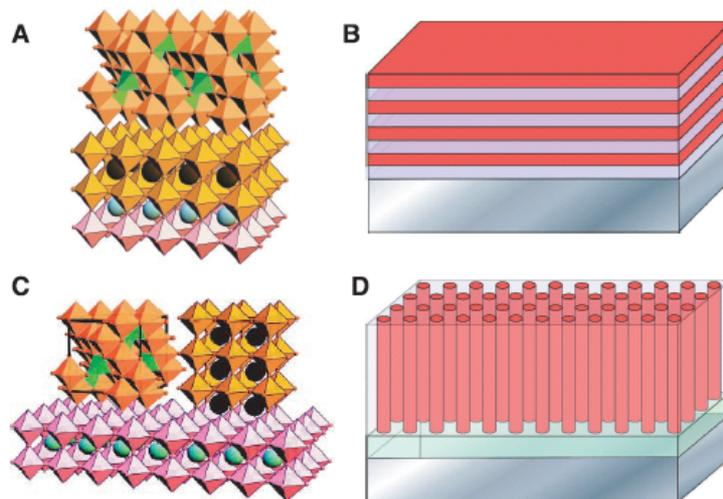
**Figure 1-40 a) Multilayer heterostructured spinel (top) and perovskite (middle) on a perovskite substrate (bottom) b) A schematic of thin film multilayers on a substrate c) Epitaxial nanostructures of a spinel and a perovskite on a perovskite substrate d) Schematic of a self-assembled nanostructure on a thin film and substrate. (Reprinted by permission from AAAS; Science. (Zheng, 2004).**
