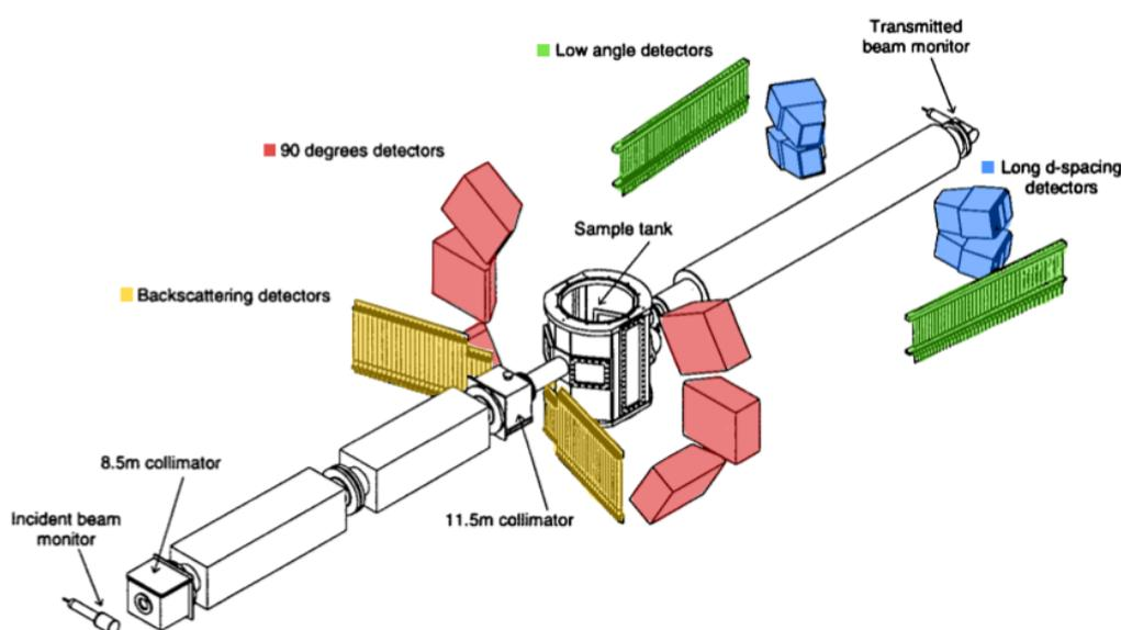
**Figure 3-2 Schematic of the Polaris neutron powder diffractometer instrument at ISIS, Oxford, UK (Smith, 1997).**
