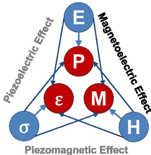
**Figure 1-34 Multiferroic coupling illustration. The magnetoelectric effect is highlighted as per the example given in the text.**
