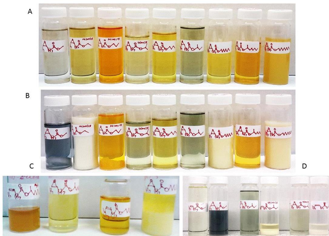
**Figure 3- 11 Variation of colour shades with (a) alkyl oleate epoxides at production, (b) frozen alkyl oleate epoxides days after production, (c) alkyl oleate juxtaposed with corresponding epoxides at production, (d) alkyl oleates juxtaposed with corresponding epoxides days after production**
