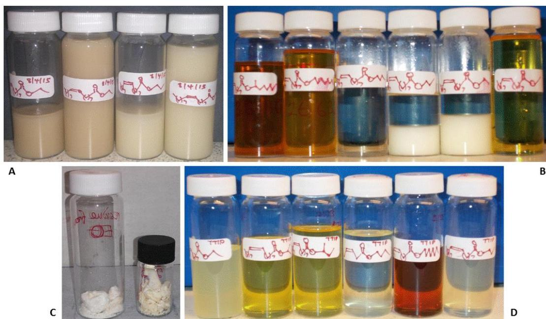
**Figure 2- 11 Transesterification products showing (a) formation of waxy oleates (b) different shades of amber coloured  $KF/Al_2O_3$  and  $MgO-T600$  catalysed oleates (c) residues from filtered waxy oleates (d) different shades of amber coloured  $Ti(O-i-Pr)_4$  catalysed oleates**
