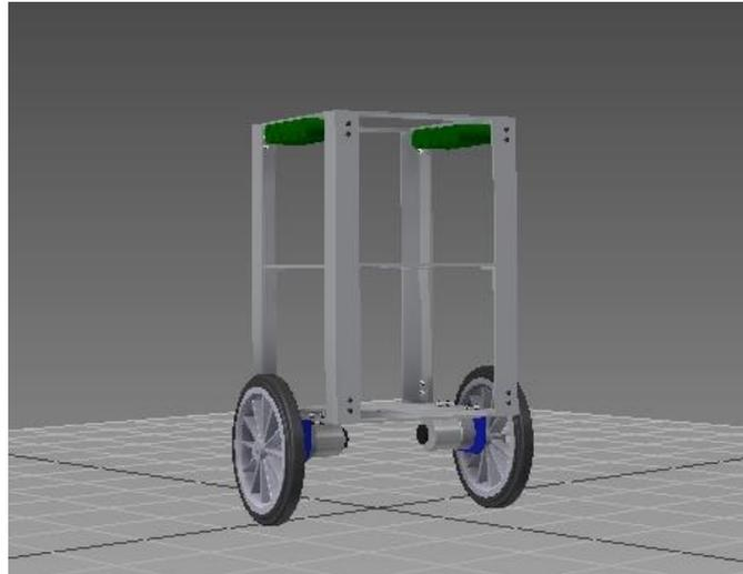
**Figure 2.3:** CAD model of the two-wheeled robot
