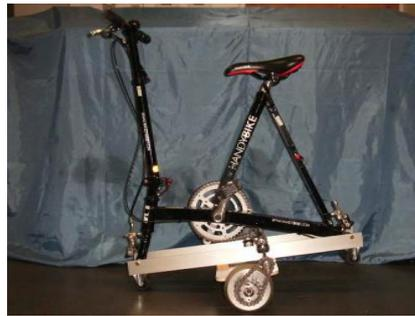
**Figure 1.7:** *The two-wheeled inverted pendulum vehicle with pedals*
