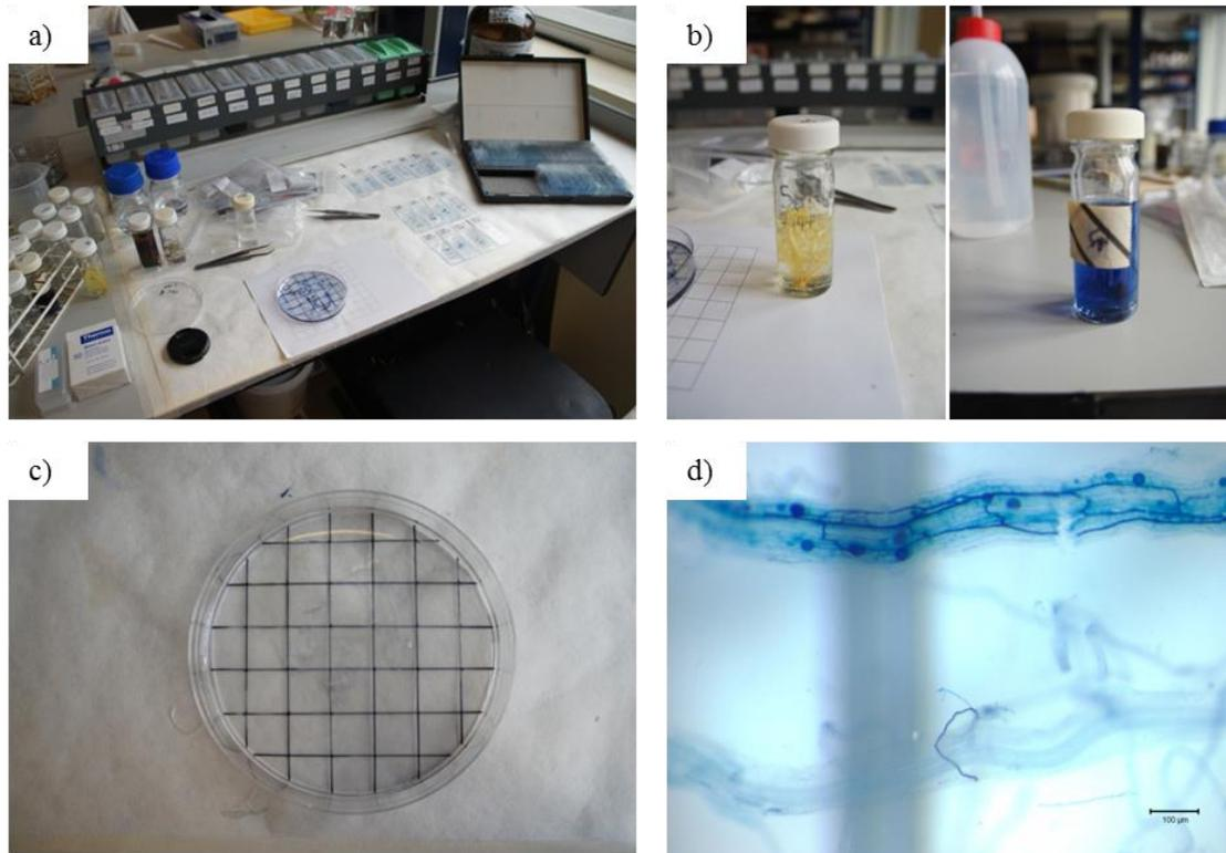
**Fig. 2.4** Equipment used for staining and quantifying mycorrhizal colonisation. a) Picture of all equipment used. b) Roots in 10 % KOH before staining and in 50 % glycerol after staining. c) Grid lines drawn onto 9 cm petri dish to make 1.27 cm diameter squares. d) View of roots under dissecting microscope x80 magnification. The top root is colonised with visible intraradical hyphae and vesicles, while bottom root is not colonised. Scale bar = 100 µm.
