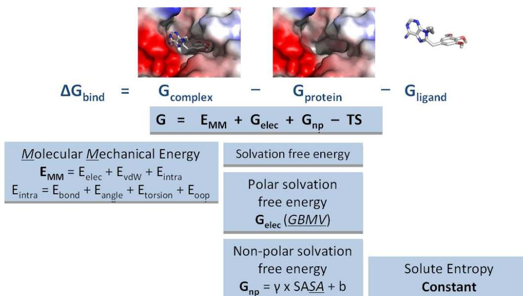
**Figure 4.4. Summary of the scoring scheme (MM/GBMV-SA) used in this study.**
