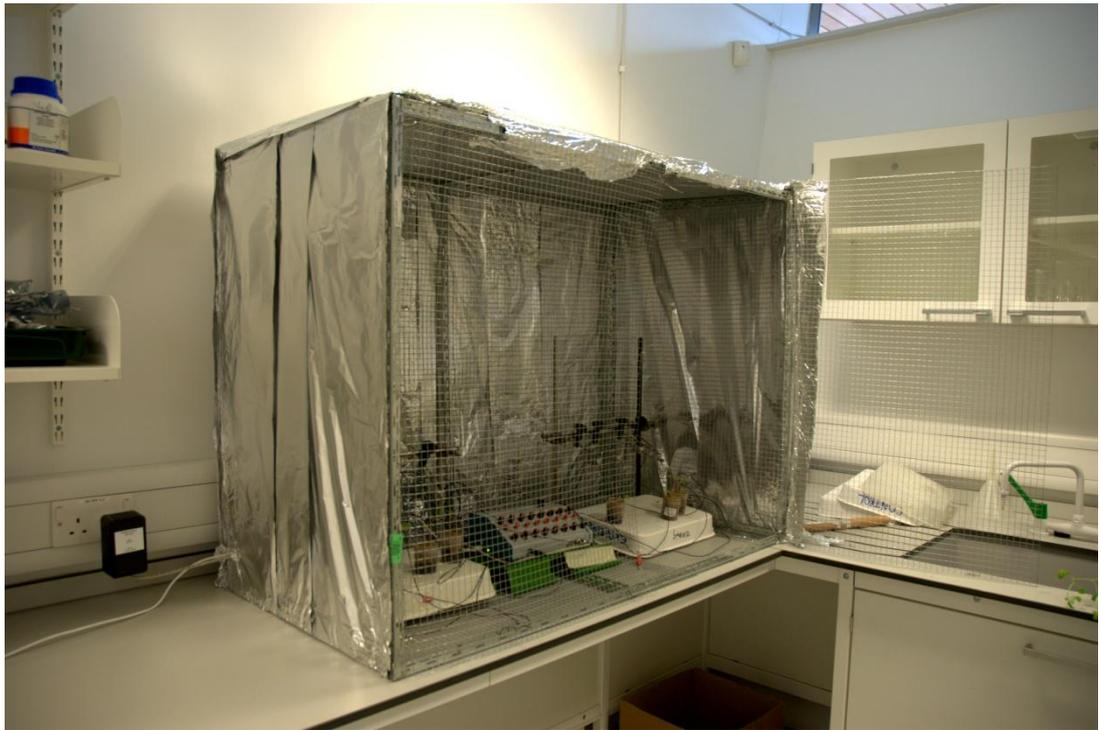
*Figure A5.1: Side view of full EPG set-up contained within Faraday cage.*
