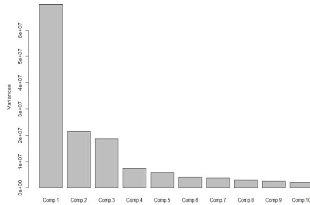
*Figure A8.1: Screen plot for PCA of 60waveforms. Results show that nearly all the variance is contained within the first three PCA components, and more than half within PC1.*
