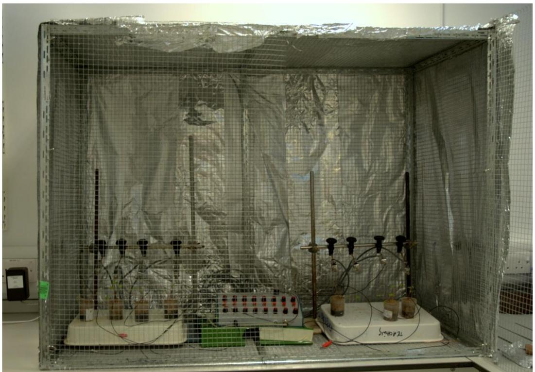
*Figure A5.2: Front view of full EPG set-up contained within Faraday cage.*
