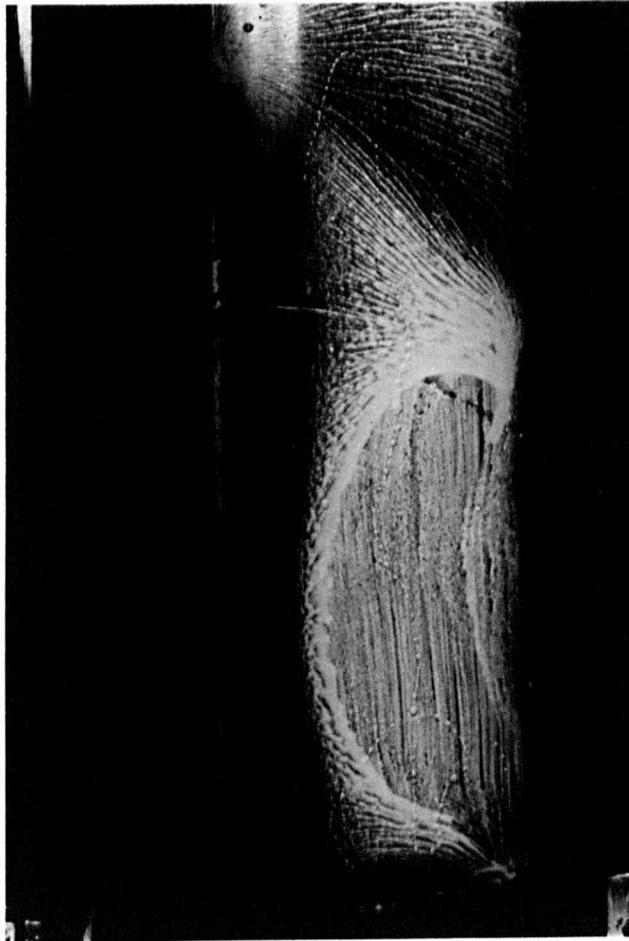
**Figure 8.13 – The Vertical Striations of the Oil Pattern as Originally Applied are Unchanged in the Region of Tail Separation. Evidence of Re-entrant Flow Can Be Seen at the Trailing Edge.**
