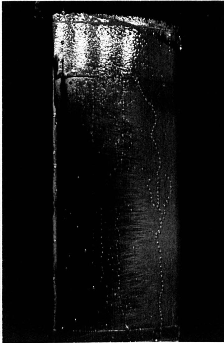
Figure 8.7 – Blunt Biogive with Tape on Upper and Lower Part of Slot and Smoothed Leading Edge. 20 ft/s (6m/s)  $\beta = 12$  Degrees, Maximum Suction.
