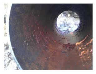
Figure 6.39: The TM-WB main was drained down during September 2012 to repair a leak. This allowed for the visual inspection of condition of the pipe wall. Part of the DI section is shown here.
